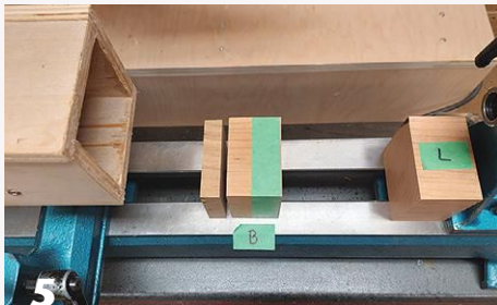
5 Add a spacer and then the box base with its top wrapped with masking tape into the clamp.
