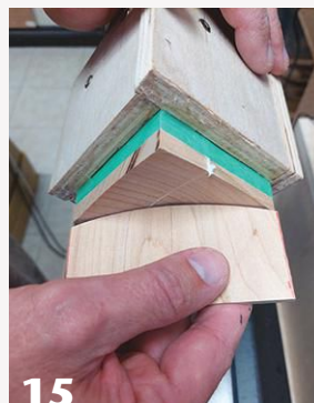
(13) Creating a simple template for the dents helps achieve a consistent shape on all six sides of the box.
