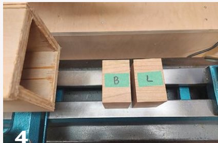
4 Cut the turning blank to create top and bottom box sections. Label each face.
