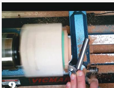
9 Create a tenon to fit the base using a shoulder cut across the square lid.
