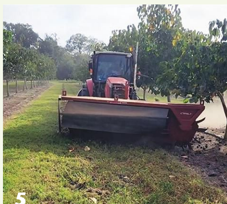
Modern harvesting utilizes equipment developed for pecan orcharding. A sweeper piles the fallen fruit in the center of the row where a harvester can glean the crop and load it in a hopper for transport.
