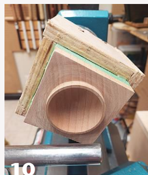
10 Hollow the lid, going no deeper than 3/4" past the square face.
