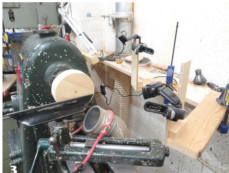
Two camera angles on the lathe give the audience the best view of the action.
