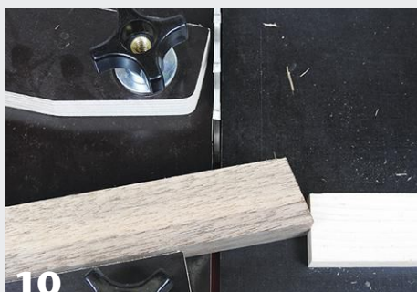
10 Now set the long point of the angle against the stop and cut a segment. Flip the strip so the long point is once again at the bottom, push it against the stop, and cut another segment. Continue this process until all segments are cut.
