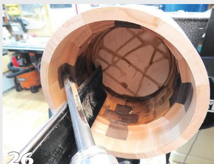
A variety of tools is used on the box's interior—a bowl gouge, a bottom feeder bowl gouge, and a negative-rake scraper.
