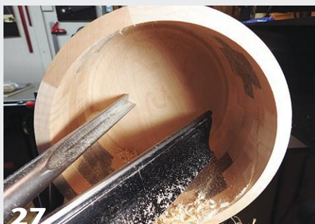
A variety of tools is used on the box's interior—a bowl gouge, a bottom feeder bowl gouge, and a negative-rake scraper.
