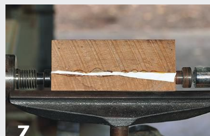
The author pre-drills the center points to avoid accidentally splitting the blank while mounting it between centers.
