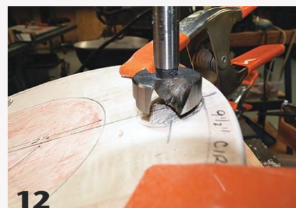
12 Carefully position the drill bit on the 120-degree line and just touching the inner circle, ensuring the hole will be 1/2" from the seat's edge.
