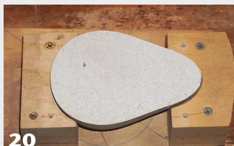
A custom holding jig opens up possibilities for mounting non-round objects on the lathe. Ensure the work is held securely and is centered and balanced. Larger odd-shaped pieces might require counter weights, but not this small avocado box.
