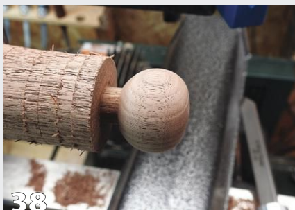
38 Shape the knob, then drill a recess to accept the BoC logo bead.
