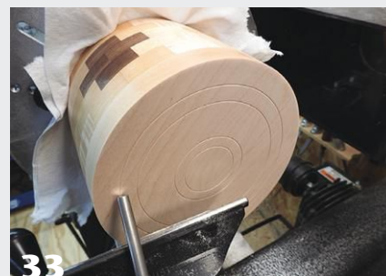
The box is reverse-mounted so the bottom tenon can be removed and decorative lines added to the base.
