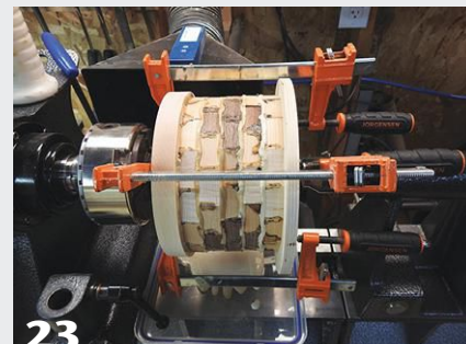
23 Glue the rest of the rings, applying pressure with clamps.
