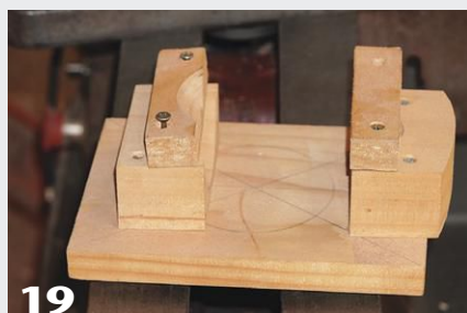
A custom holding jig opens up possibilities for mounting non-round objects on the lathe. Ensure the work is held securely and is centered and balanced. Larger odd-shaped pieces might require counter weights, but not this small avocado box.
