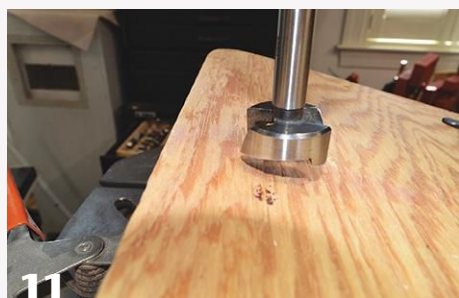
11 Set the depth stop on the drill press to leave 1/4" of wood. The leg hole should not extend through the top of the seat.
