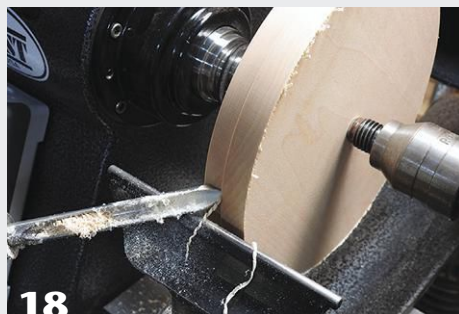
18 The disk is mounted on the lathe and trued. Form a tenon for remounting in a chuck.
