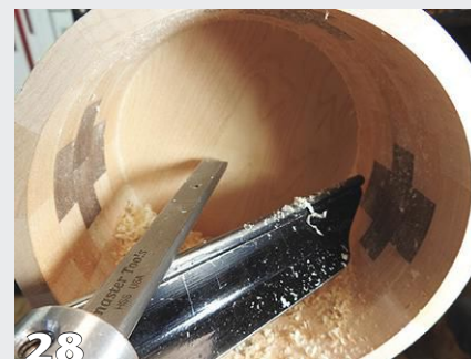
A variety of tools is used on the box's interior—a bowl gouge, a bottom feeder bowl gouge, and a negative-rake scraper.
