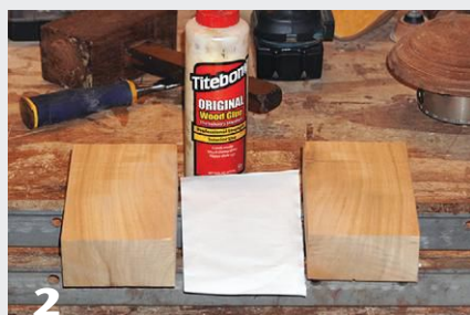
2 Spread wood glue evenly and clamp the two halves together with paper between them.
