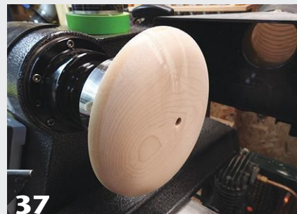
36 Complete the shaping of the lid, reverse-mounting it on the woodworm screw to gain full access to the top.
