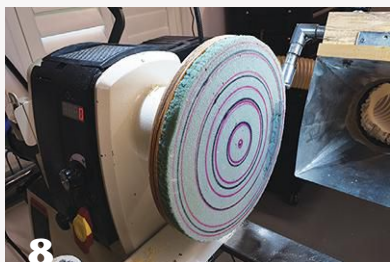
8 The author uses a jam chuck to mount the seat blank on the lathe. Cover a circle of plywood with carpet underlayment and mount on a faceplate as the drive portion of the jam chuck. The work is held in place with tailstock pressure.
