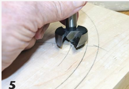
5 Position a 1 3/8" Forstner-style bit at the intersection of the 9 1/2" layout circle and the 120-degree line and create an indent. This marks where the drill bit should be placed for the leg holes to be 1/2" inside of the edge of the seat.
