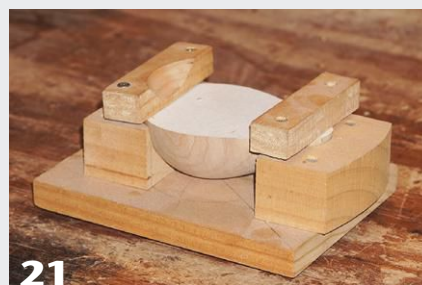
A custom holding jig opens up possibilities for mounting non-round objects on the lathe. Ensure the work is held securely and is centered and balanced. Larger odd-shaped pieces might require counter weights, but not this small avocado box.
