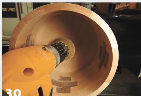
29 Power-sand the outside walls of the box and the interior bottom.
