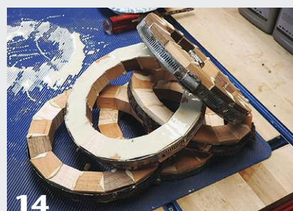
13 Glue the segments into rings—in this case, sixteen segments per ring. Band clamps apply gluing pressure.
