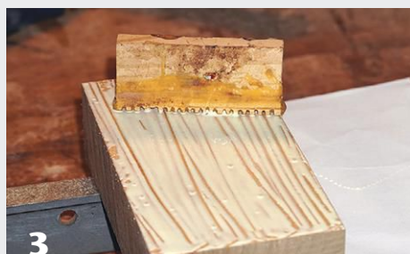
2 Spread wood glue evenly and clamp the two halves together with paper between them.
