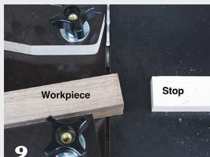
9 Without contacting the stop, first establish a cut angle on the end of a strip.
