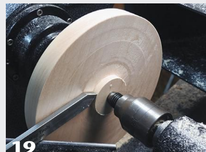
18 The disk is mounted on the lathe and trued. Form a tenon for remounting in a chuck.
