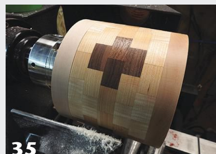
Material for the lid is mounted on a screw chuck (woodworm screw) and fitted to the box rim.
