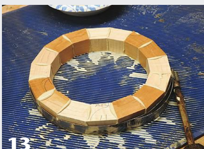
13 Glue the segments into rings—in this case, sixteen segments per ring. Band clamps apply gluing pressure.
