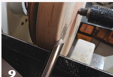
9 True the outside surface and relieve both edges of the seat.
