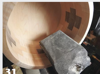
The authors use a soft sanding pad on the interior walls.
