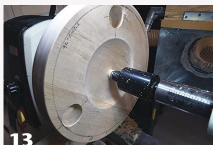
13 The author forms a 3/8"-deep recess in the center of the seat bottom. This allows for the removal of the live center indent and makes the stool easier to hold.
