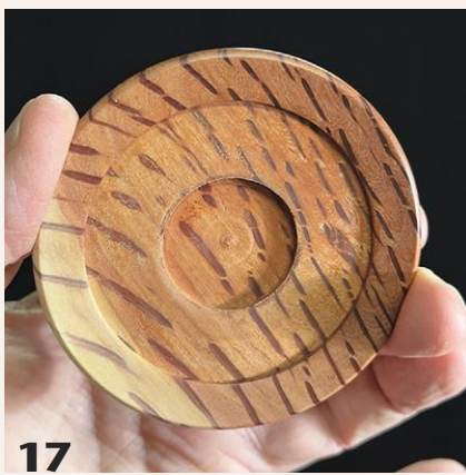
The completed mirror casing, ready for final buffing.
