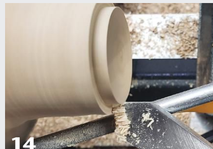
13 Rough-turn the ornament body and form a tenon at the top sized to fit into the recess in the roof.
