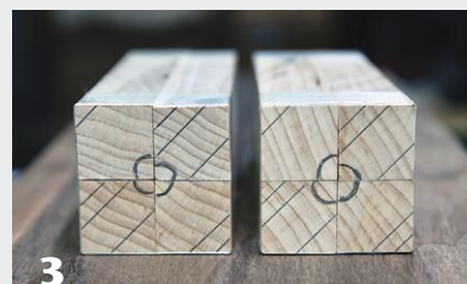
3 Rotate each piece of the blank so that the outside corners are toward the inside of the blank. Your penciled arcs should form a rough circle. Your blank is now ready for taping.
