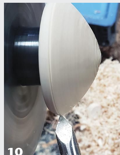
The author uses a point tool to add a groove separating areas of two different texture patterns.
