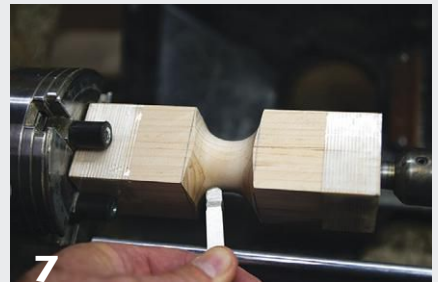
7 Refine the shape and depth of the cove by taking light cuts with a 3/8" (10mm) scraper and retesting the template often.
