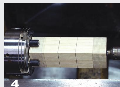
4 The author mounts the blank between a four-jaw chuck fitted with repurposed Cole jaw rubber pins at the headstock and a live center with cup and point at the tailstock.
