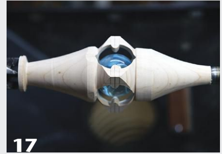
17 Begin shaping the exterior of the cage, making sure to leave enough mass to support the blank.
