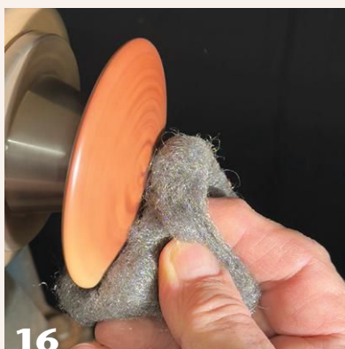
With the work still on the lathe, the author polishes it with 000 steel wool.
