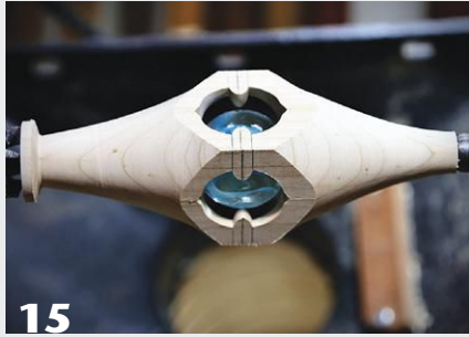
15 Mark three lines around the blank for accurate placement of the outside bead: one at the center of the inner bead and one at each outside edge.
