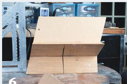
6 To safely cut the cone shape into angled sections at the bandsaw, the author made a custom V-block sled with 75-degree ends.
