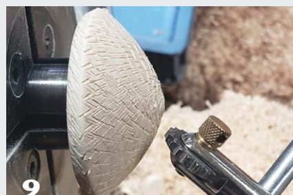
7 The author chooses a texturing tool and then applies it to the spinning roof top. The trick is not speed but concentration and deliberate movement of the tool.
