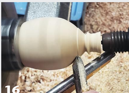
16 Reverse-mount the workpiece, now holding it by the tenon, so you can shape and finish the body.
