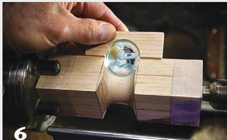
6 Check your progress by placing the shop-made arch template at the corner and seeing if the marble passes through.
