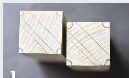
1 Mark one end of your blank with three diagonal lines and an arc at each corner.
