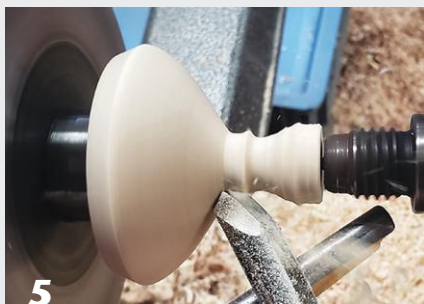
5 Reverse-mount the roof, now gripping it with pin jaws in expansion mode. Shape the roof top.
