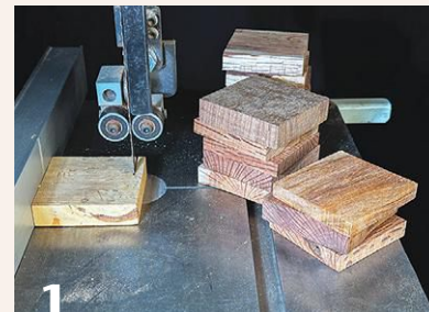
1 Cut multiple blanks the same size. The author keeps a mirror blank near the bandsaw for quickly setting the fence.
