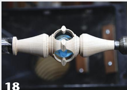
18 Continue refining both the cage and the finials, moving back and forth between detail areas.
