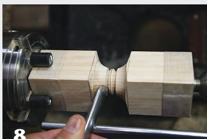
8 Mark a pencil line at the center of the cove, then turn a symmetrical bead around it, leaving the line intact.
