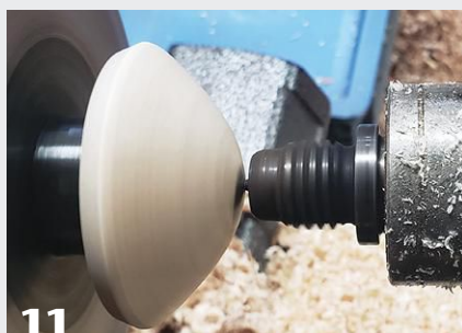
Use the tailstock live center point to make an indent as a starter hole, then drill for the screw eye.
