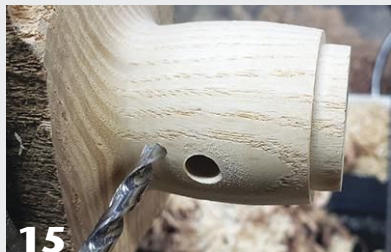
15 Drill three holes: one for the bird's perch, one for its entry port, and one to hollow the ornament body from the endgrain.
