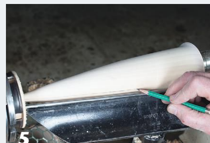
5 Using the toolrest as a straightedge, draw two lines the length of the form at center height, 180 degrees apart from each other.
