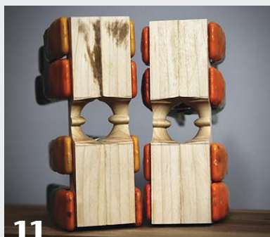
11 Glue up each half of the blank, placing clamp pressure along the full length of the glue joint and ensuring the ends and faces are flush ( See sidebar, Tips for Gluing the Blank ).
