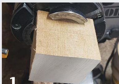
1 The square roof blank is mounted in the chuck.
