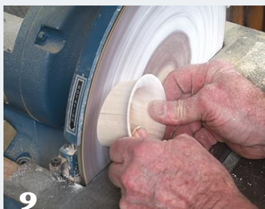
9 Lightly sand the surfaces that are to be glued.
