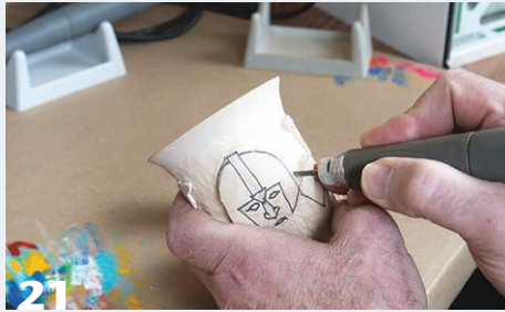
20 After drawing feature elements onto the wood, the author defines edges using a straight-sided carving bur, then trims away background areas.
