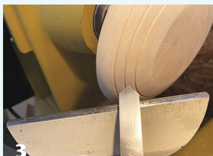
3 Form a V-groove (or grooves) using a pointed scraper.
