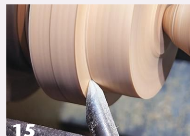
15 The author uses a detail gouge to form a tight corner at the shoulder of the dome.
