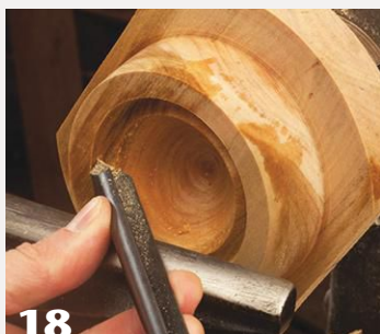
18 Hollow the interior of the bowl. The author starts with a bowl gouge with a traditional side grind and then switches to a blunter "bottom feeder," which maintains bevel support at the bottom.
