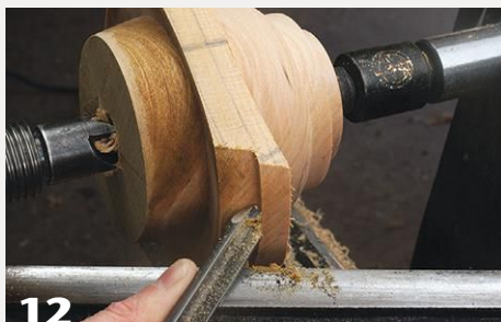
12 Shape the outside edge of the handle to a slight angle.
