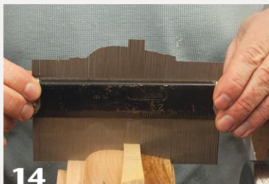
14 Check the profile of the bowl with the help of a contour gauge. Aim for a continuous line above and below the handle flange.
