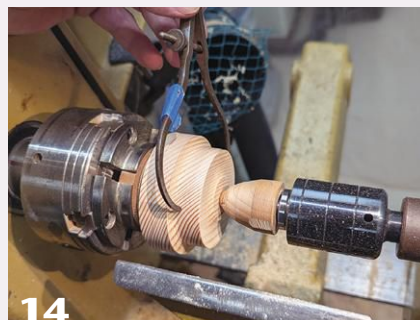
13 The dome's diameter is established and confirmed with a preset caliper.
