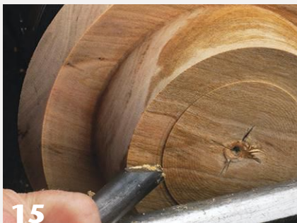
15 With the bowl now mounted in a chuck, the author first flattens the face using a shear-scraping cut and then angles the rim inward with a bevel-supported cut.
