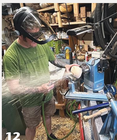
12 Periodically during hollowing, the wood shavings must be cleared. A blast of compressed air does the job.
