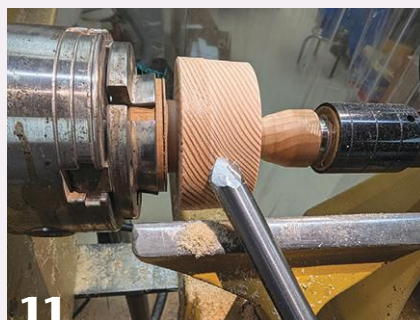
11 The author turns the work to its maximum diameter, 3\frac{1}{2} ".
