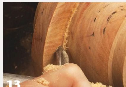
13 The author uses a small spindle gouge to clean up the corners where the flange meets the bowl.
