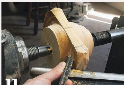
11 Shape the top half of the bowl, leaving a rectangular flange that will later become the handles.
