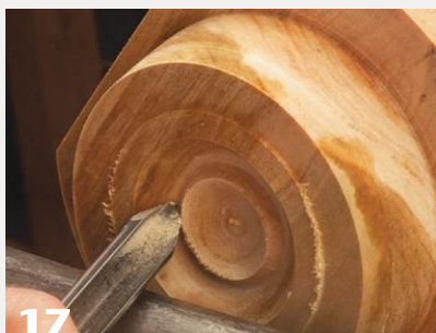
17 Hollow the interior of the bowl. The author starts with a bowl gouge with a traditional side grind and then switches to a blunter "bottom feeder," which maintains bevel support at the bottom.
