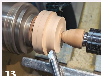
13 The dome's diameter is established and confirmed with a preset caliper.
