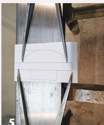
5 Dividers are set directly from the printed design drawing.
