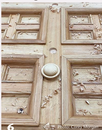
6 The author's customer, a professional woodworker, predrilled mortises in the custom doors to accept the tenons turned on the medallions.
