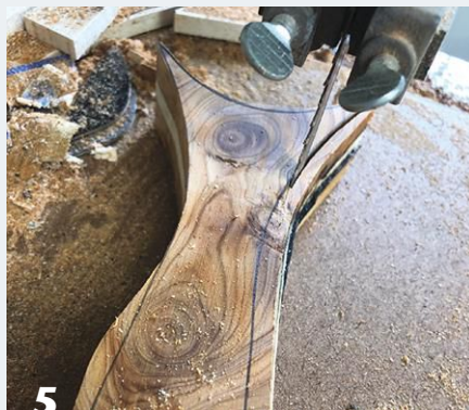
5 Prior to turning the handle, refine the upper area that will later accept the laminated hoop strips.
