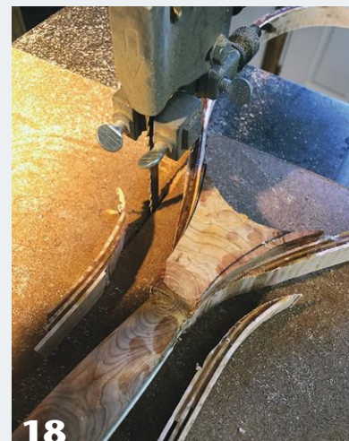
18 When the glue has dried, remove the frame from the form. The author cuts away excess material prior to hand-shaping and refining.
