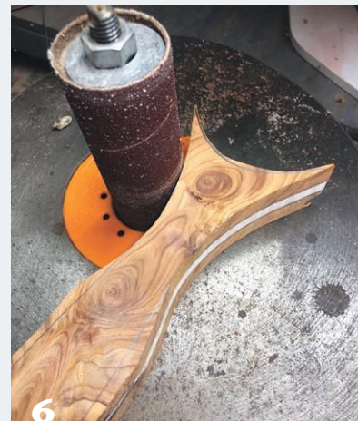
5 Prior to turning the handle, refine the upper area that will later accept the laminated hoop strips.
