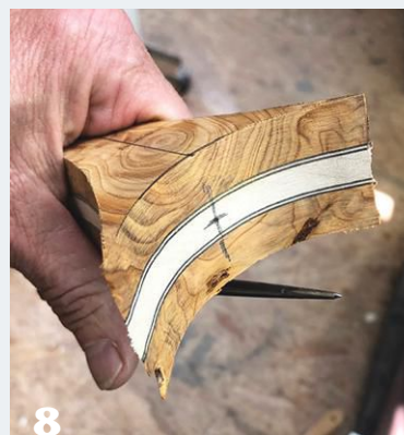
The top end of the handle should be sanded smooth and the center marked in preparation for mounting on the lathe.
