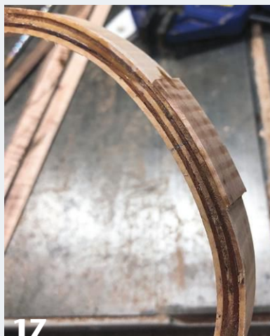
17 The author glues on an extra layer at the top of the frame where a magnet will be embedded.
