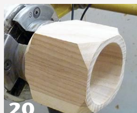
Mount the base and drill to depth. Then hollow the base and carefully size the interior width for a good fit to the spigot on the lid.
