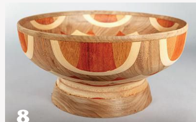
8 A good way to assess the design of a work in progress is to remove it from the lathe. Hence, the importance of reliable mounting and remounting methods. Thus far, the bowl shape is nearly complete, but the base must be reduced further.
