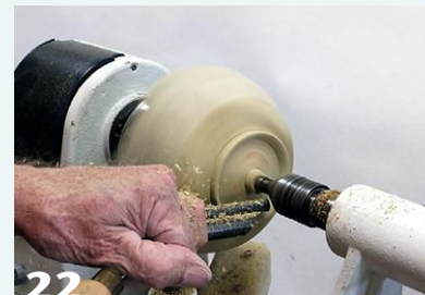
22 With the bowl reverse-mounted on the lathe, turn the base and create a foot ring.
