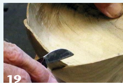
A sharp knife is used to define tight transitions.
