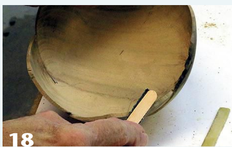
The author uses a sanding sleeve in a micromotor tool and shopmade sanding sticks to refine the petal surfaces and edges.
