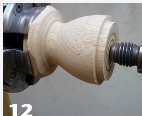
12 The author begins to shape the domed lid and uses a gouge and scrapers to hollow the lid.
