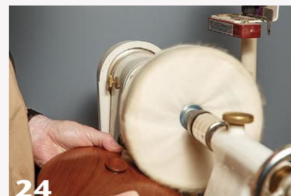
24 Once the finish has cured, both the lid and the bowl make a trip through the lathe-mounted buffing wheels to achieve the final sheen.
