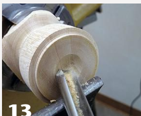
12 The author begins to shape the domed lid and uses a gouge and scrapers to hollow the lid.
