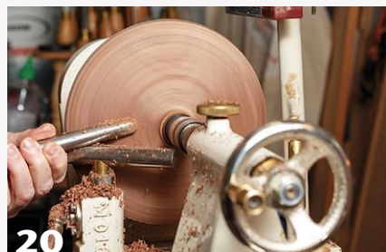
20 The author turns and power-sands the top of the lid.
