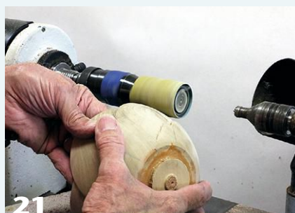
21 A lathe-mounted pneumatic sanding drum is used to refine the bowl's exterior.
