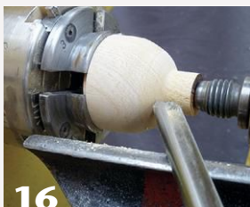
Reverse-mount the top with the spigot used as a chucking tenon. Carefully turn the dome shape, keeping the tailstock in place as long as possible. The author forms a subtle band at the bottom and a small finial at the top.
