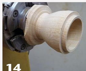
The spigot is refined to a suitable length with parallel sides, and the shoulder undercut slightly for a good fit to the base.
