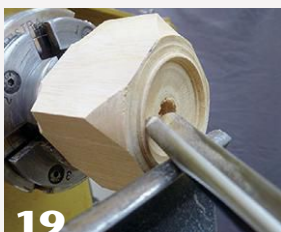
Mount the base and drill to depth. Then hollow the base and carefully size the interior width for a good fit to the spigot on the lid.
