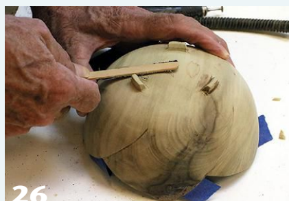
25 The author uses a knife and sanding sticks to refine the feet and base.
