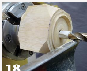
Mount the base and drill to depth. Then hollow the base and carefully size the interior width for a good fit to the spigot on the lid.
