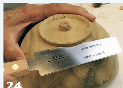
23 Cut away the waste wood from the foot ring, leaving only three small feet.
