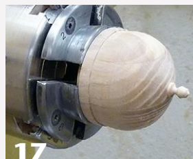
Reverse-mount the top with the spigot used as a chucking tenon. Carefully turn the dome shape, keeping the tailstock in place as long as possible. The author forms a subtle band at the bottom and a small finial at the top.
