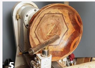
5 With the underside thinned and reshaped, the interior is addressed while there is still sufficient wall thickness for some cutting and reshaping as needed.
