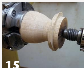
Reverse-mount the top with the spigot used as a chucking tenon. Carefully turn the dome shape, keeping the tailstock in place as long as possible. The author forms a subtle band at the bottom and a small finial at the top.
