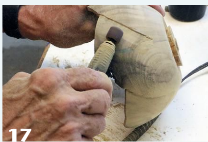
The author uses a sanding sleeve in a micromotor tool and shopmade sanding sticks to refine the petal surfaces and edges.
