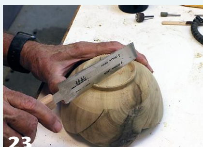
23 Cut away the waste wood from the foot ring, leaving only three small feet.
