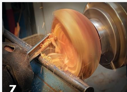
Use ample downward pressure on the toolrest when making the intermittent entry cuts on a natural-edge bowl.
