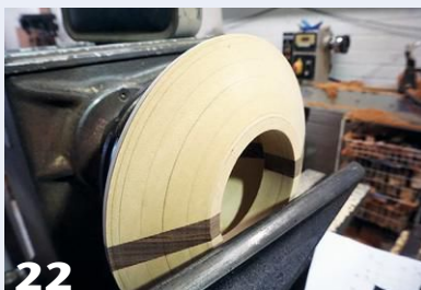
22 A straight angled cut represents the line between the tail tips, on which intermediate points are drawn.
