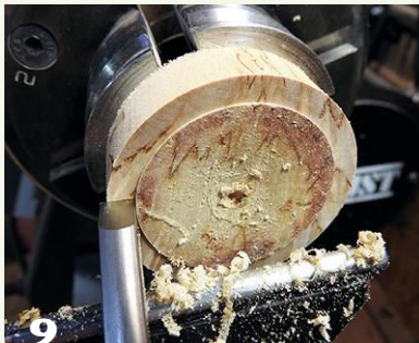
The lid material is mounted in the chuck and its face trued up.
