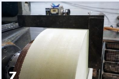
7 The author turns the blank to the exact diameter and checks for square.
