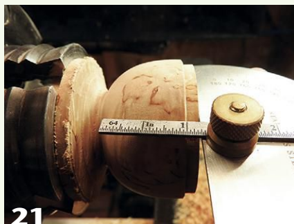
21 A gauge indicates hollowing depth, and the author hollows, sands, and finishes the inside of the box, just as he did the lid's interior.
