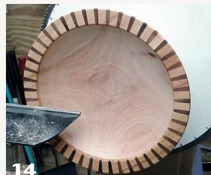
13 The author glues in contrasting inlays and then turns them flush.
