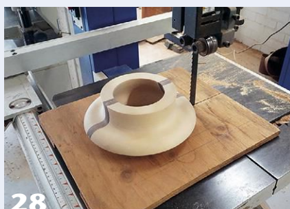
28 At the bandsaw, cut the ring in half, splitting the accent wood down the middle.
