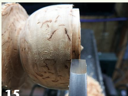
15 With the lid removed from the chuck and the box body mounted, form a tenon sized to accept the mortise inside the lid. Stop the lathe frequently and test the fit of the top to the box.
