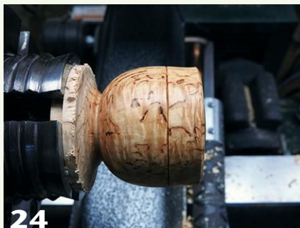
24 After sanding and finishing the outside of the box (with the lid on), the author parts the box from the wastewood, leaving extra material to work with when completing the bottom.
