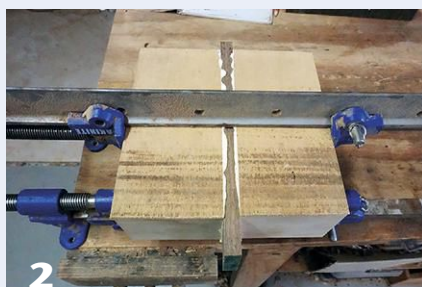
2 The turning blank is first laminated with an accent strip in the middle, then bandsawn round, ready for the lathe.
