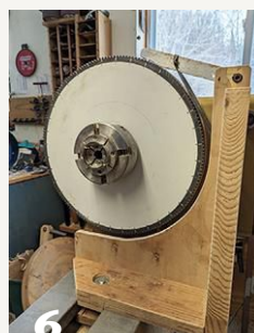
(4) A pivot arm made from aluminum locks the indexing wheel in place.
