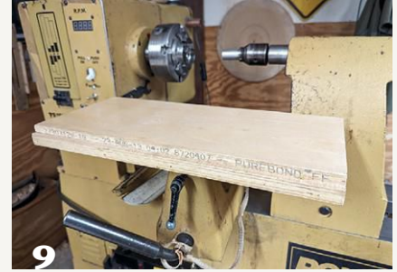
8 A double layer of plywood, mounted in the lathe banjo, serves as a platform for the router.
