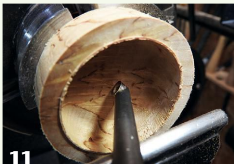
Most of the hollowing is accomplished using a carbide-tipped tool. Then the surface is refined using a negative-rake scraper, whose bottom bevel is sharpened to 70 degrees and top bevel, 20 degrees.
