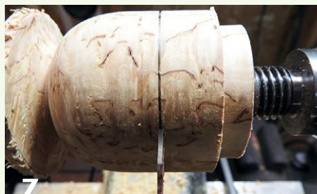
7 Use a very thin parting tool to separate the lid from the box. The golden ratio provides good proportions.
