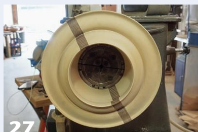
27 The turning is complete. Sand lightly to avoid altering your carefully achieved shapes and transitions.
