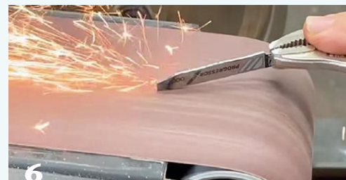
A jigsaw blade will serve as the chatter tool cutter. Grind off its teeth and shape it using a grinder or belt sander.
