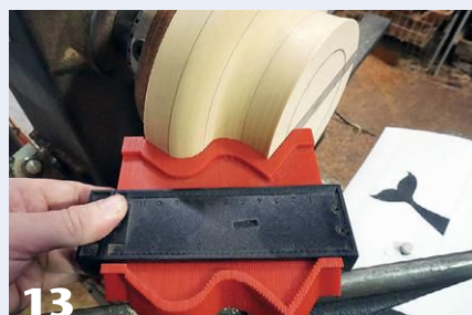
13 The author uses a profile gauge to test the shape of the wood against his template. The gap at the base of the tail indicates where more wood needs to be removed to achieve the desired shape.
