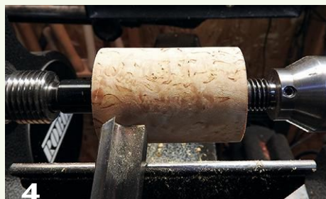
4 Turn the workpiece round and form a tenon at each end.
