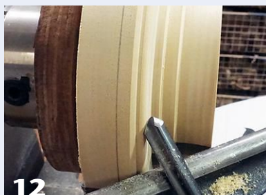
12 The curves are formed and blended using shear-scraping cuts with the wing of the bowl gouge.
