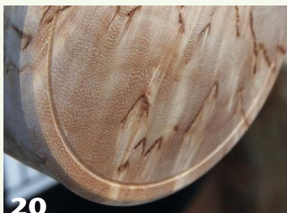
19 With the tape removed, two accent lines are added, one at the lid joint and one near the edge of the top of the lid. Understated styling details along with good form highlight the wood's natural beauty.
