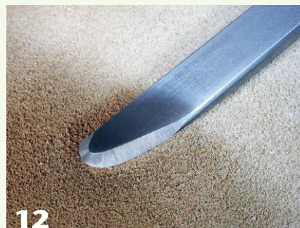
Most of the hollowing is accomplished using a carbide-tipped tool. Then the surface is refined using a negative-rake scraper, whose bottom bevel is sharpened to 70 degrees and top bevel, 20 degrees.
