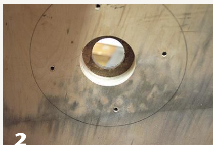
2 The flywheel ring is modified to fit on a lathe spindle.
