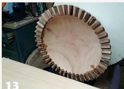
13 The author glues in contrasting inlays and then turns them flush.
