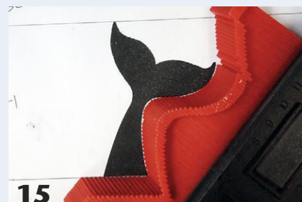
13 The author uses a profile gauge to test the shape of the wood against his template. The gap at the base of the tail indicates where more wood needs to be removed to achieve the desired shape.
