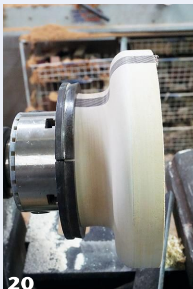
20 The work is reversed and held in large dovetail jaws.
