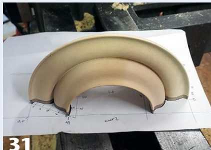
31 A final check against the paper template confirms accurate turning.
