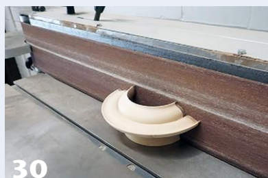
30 Flatten the ends and lightly sand away the bandsaw marks. The author uses a linisher and then sands by hand.
