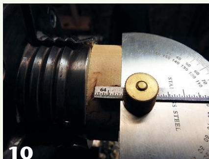
Use a depth gauge to note how deep you can hollow the lid without busting through the top.
