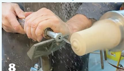
The author presents the side of the flexible blade to the hardwood endgrain, producing intermittent cuts. Adding color accentuates the chatter marks beautifully.
