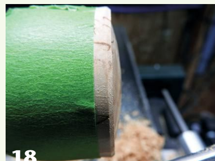
17 The author applies painter's tape over the lid-to-box union for added holding power. He then turns away the chucking tenon and forms a subtle dome at the top of the lid.
