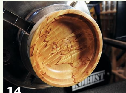
14 The author sands inside the lid, but not the carefully shaped mortise. He applies and buffs an abrasive wax finish.
