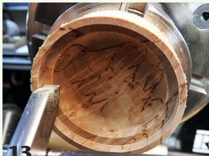
13 A wide parting tool, or bedan, is used to form a mortise, or stepped recess, inside the lid. This mortise will later fit precisely to a tenon on the box body.
