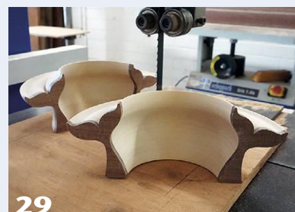
28 At the bandsaw, cut the ring in half, splitting the accent wood down the middle.
