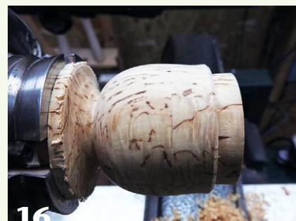
16 The lid is friction-fit onto the box tenon, allowing for final shaping of the outside of the box. The chucking tenon at far right will be removed.
