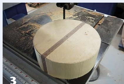
2 The turning blank is first laminated with an accent strip in the middle, then bandsawn round, ready for the lathe.
