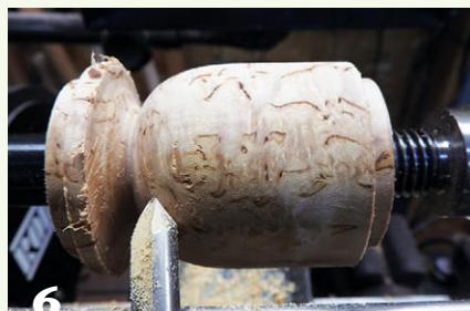
6 A spindle gouge is used to rough-shape the box's round bottom.
