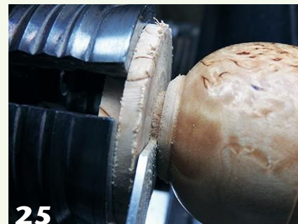
24 After sanding and finishing the outside of the box (with the lid on), the author parts the box from the wastewood, leaving extra material to work with when completing the bottom.
