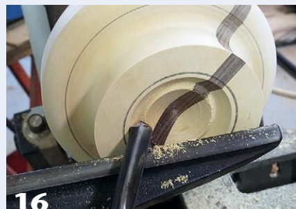
16 The author uses a bowl gouge to remove wastewood from the center.
