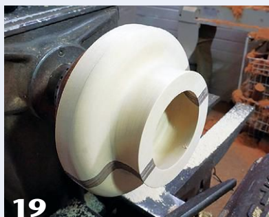
19 With the curves of the first side completed according to the measurements on the template, sand the piece lightly.
