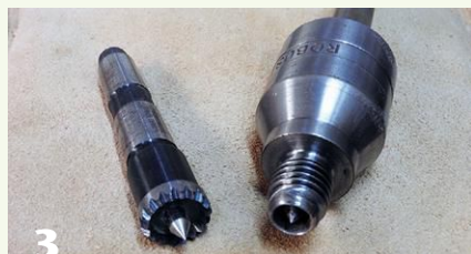
3 The combination of a multi-toothed drive and a live center whose point is adjusted to protrude only slightly reduces the chance of splitting the wood when it is mounted between centers.
