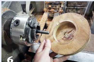
6 A spacer ring with a recess adds surface area when using a screw chuck, increasing stability during turning.
