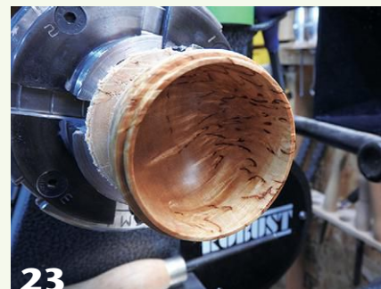
21 A gauge indicates hollowing depth, and the author hollows, sands, and finishes the inside of the box, just as he did the lid's interior.
