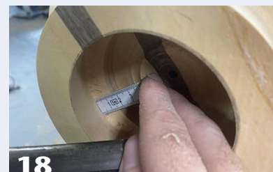
18 The author transfers measurements to the enclosed central area using a cut-down plastic ruler. Making cuts precisely in this area is more challenging than on the outside.
