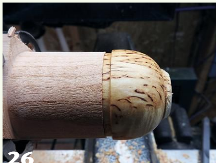
26 A length of scrap wood is mounted in the chuck, and the author forms a jam chuck. Not shown is a short tenon at the end of the jam chuck onto which the interior of the box is friction-fit.
