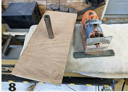
8 A double layer of plywood, mounted in the lathe banjo, serves as a platform for the router.
