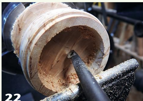
21 A gauge indicates hollowing depth, and the author hollows, sands, and finishes the inside of the box, just as he did the lid's interior.
