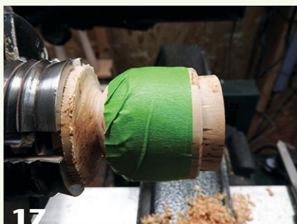
17 The author applies painter's tape over the lid-to-box union for added holding power. He then turns away the chucking tenon and forms a subtle dome at the top of the lid.
