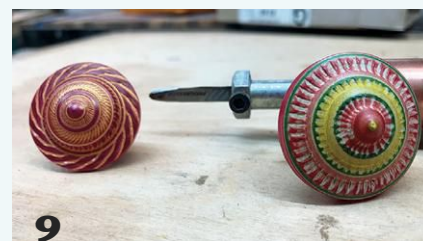
The author presents the side of the flexible blade to the hardwood endgrain, producing intermittent cuts. Adding color accentuates the chatter marks beautifully.
