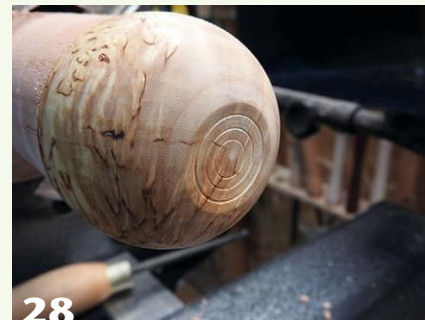
28 A flat is cut into the round bottom, making a stable base so the box can sit upon a surface without rocking.
