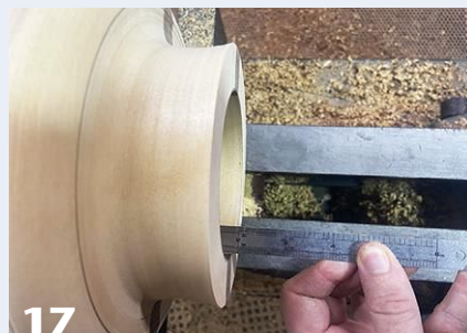
17 The walls in the center should be straight in (parallel with the bed of the lathe). A metal ruler held tight against the wall visually confirms this.
