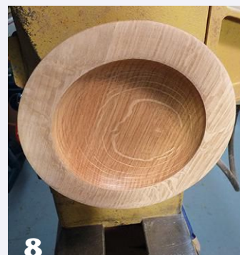
Now the top is reverse-mounted using the recess and chuck jaws in expansion mode. The wide flat rim will serve as the foundation for the segments used in the stack lamination.
