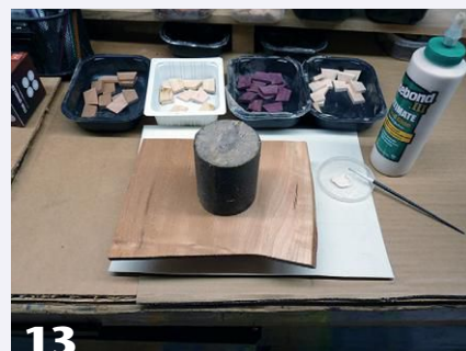
13 The first three layers are arranged and glued. Pressure is applied via a weight and flat board.
