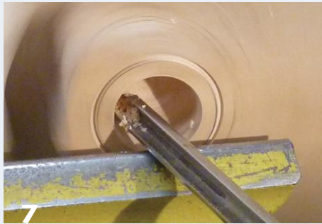
The author uses a spindle gouge and round nose scraper to hollow the bowl of the scoop.
