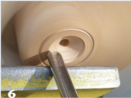
The author uses a spindle gouge and round nose scraper to hollow the bowl of the scoop.
