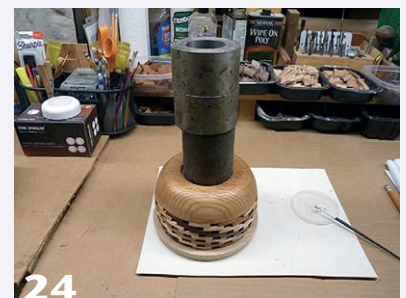
The author glues the segment assembly onto the base ring using weights for gluing pressure.
