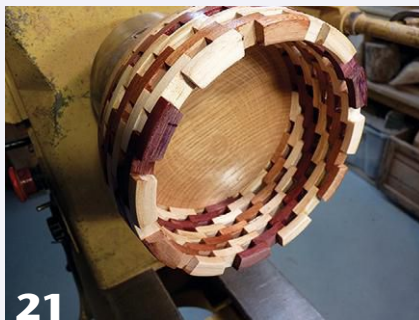
Now with nine segment layers assembled, the work is returned to the lathe and turned outside and in.
