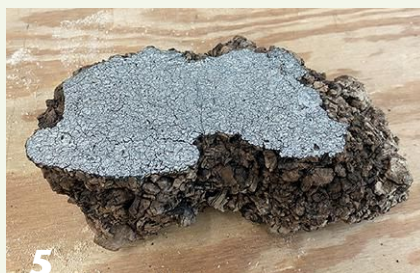
3 After bottle corks are punched from the cork oak bark, the scraps are ground into small pieces and pressed into workable blocks.
