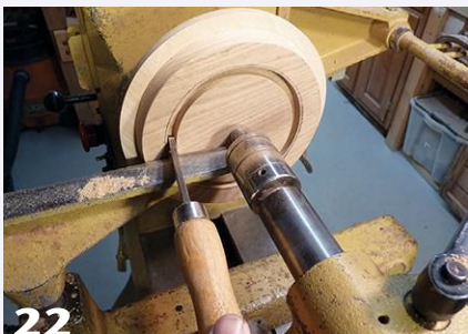
Material for the base ring is affixed to the wood faceplate using strips of double-sided tape and tailstock pressure. The author uses a parting tool to form the base ring.
