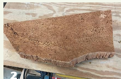
2 The average cork bark thickness is approximately 2" after it is stripped from the tree.
