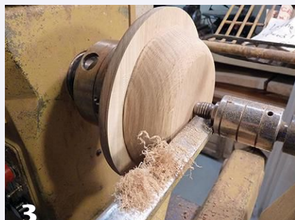
3 The top is shaped and a temporary chucking recess, or mortise, is formed.
