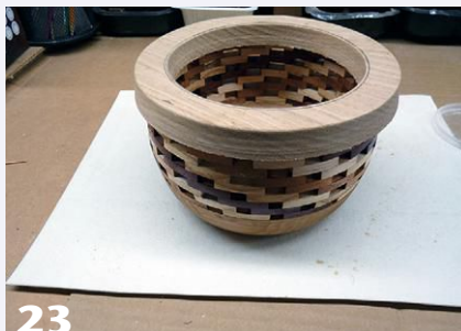
The ring is dry fit on the turned segment assembly.
