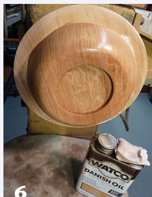
Prior to removing the top with a drywall knife, the author applies a Danish oil finish.
