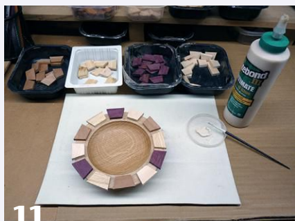
11 An assortment of precut segments in various wood species is a color palette, with which the author chooses a pattern for the open stack lamination.
