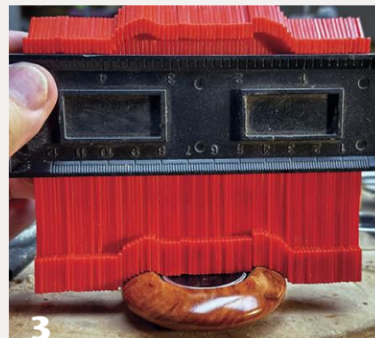
2 A sample desk compass the author was commissioned to copy in multiples. He uses a profile gauge to take a physical record of the shape to be duplicated.
