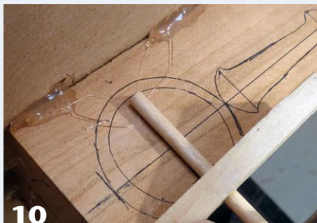
A simple shopmade jig comprising a piece of wood and a dowel is used to gauge the depth of the bowl. Holding it against the side view drawing on the blank accurately shows the progress.
