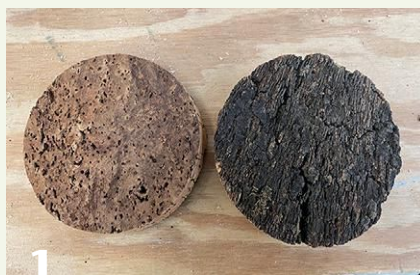
1 Examples of cork bark without and with the outer layer intact (left and right, respectively).
