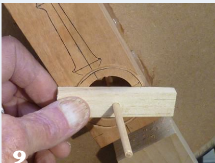
A simple shopmade jig comprising a piece of wood and a dowel is used to gauge the depth of the bowl. Holding it against the side view drawing on the blank accurately shows the progress.
