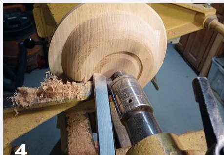
3 The top is shaped and a temporary chucking recess, or mortise, is formed.
