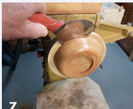
Prior to removing the top with a drywall knife, the author applies a Danish oil finish.
