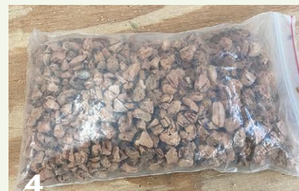
3 After bottle corks are punched from the cork oak bark, the scraps are ground into small pieces and pressed into workable blocks.
