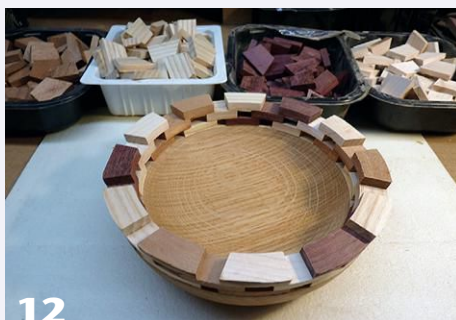
11 An assortment of precut segments in various wood species is a color palette, with which the author chooses a pattern for the open stack lamination.
