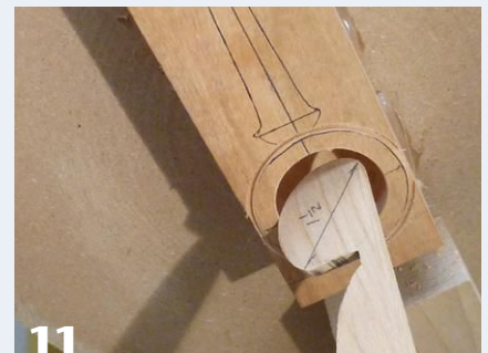
A half-round template is used to confirm the interior curve.
