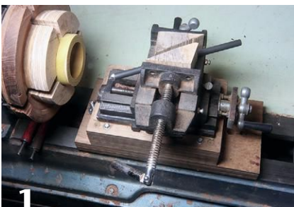
Ready to increase the diameter of the hole in an Osage orange workpiece using a gouge clamped between the vise jaws.
