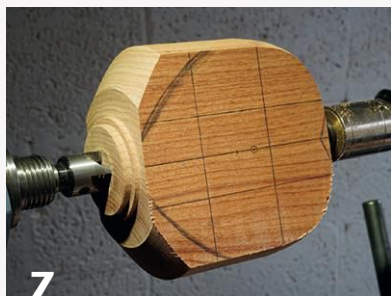
7 Form a chucking tenon at the bottom of the heart.
