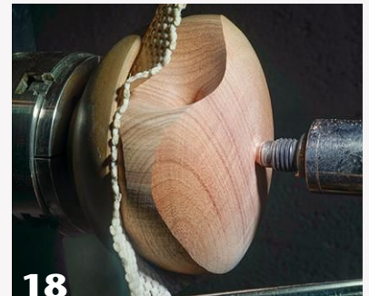
With the work jam chucked in a repurposed bowl and some drawer liner as a cushion, the author removes the tenon from the other face.
