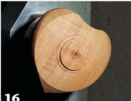
The first tenon is now held in the chuck to allow for a second tenon to be formed on the other side.
