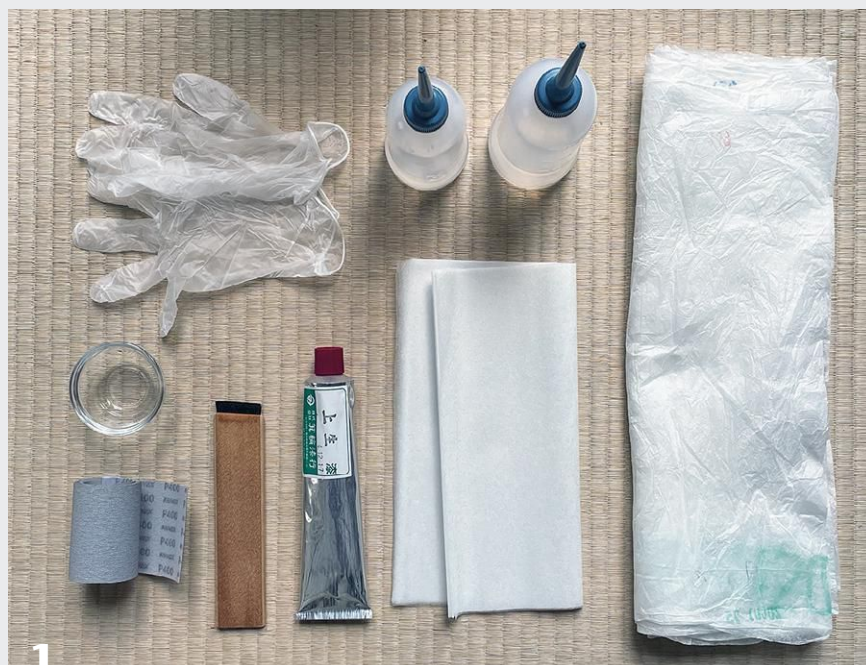
The gathered materials, clockwise from top left: vinyl gloves, solvents, filtering/straining paper, “keku” paper, a tube of lacquer, brush for applying the lacquer, 400-grit sandpaper, a dish for the lacquer.
