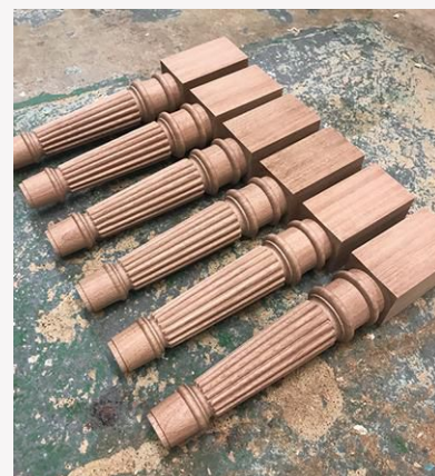
Sofa legs in sapele for a regular customer who makes replica furniture in an antique style. Findley reeded the legs with a shopmade router jig.
