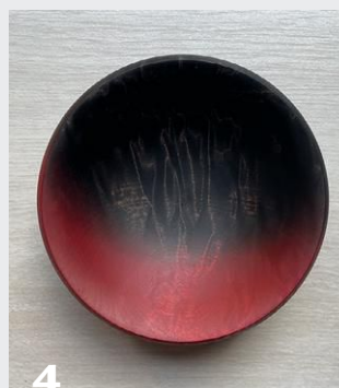
The sample bowl before lacquer is applied and after the first tinted layer is applied and then wiped. Use a wiping cloth that is not so soft that it removes all the lacquer but also not so stiff that it scratches the wood.
