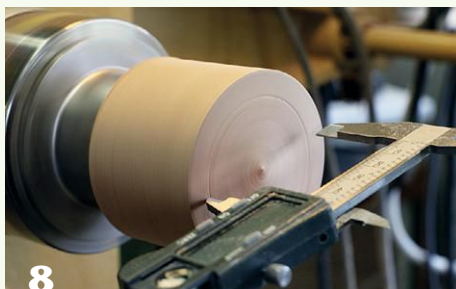
8 Use one leg of the caliper to mark what will become the inside diameter of the mortise ring, about \frac{1}{8} " smaller than the desired OD of the tenon ring. Form a straight-walled recess at this mark.
