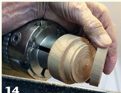
14 The freshly parted mortise ring is used to roughly gauge the diameter of the tenon ring.
