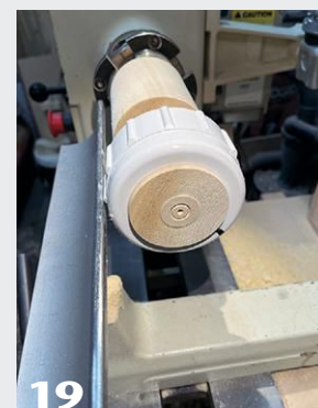
19 Remove the tailstock to test the fit of the PVC compression nut to the tapered area. Fine-tune the angle as needed.
