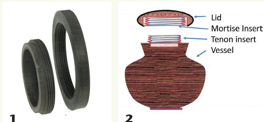
1 Threaded inserts comprise two rings, one with interior threads that fits into a recess in the lid (mortise ring), and one with exterior threads that fits into the mouth of the vessel (tenon ring).
