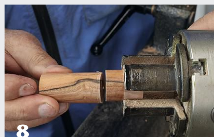
7 Use a thin parting tool to separate the box body from the lid.
