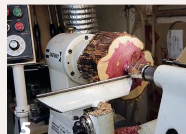
5 To turn a bowl in endgrain orientation, the work is mounted on the lathe in "spindle" orientation—i.e., with the grain running parallel to the lathe's axis.
