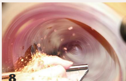
8 9 As with any endgrain hollowing, the author makes cuts from the depth hole toward the outer rim. The cedar's fluted perimeter means the hollowing should stop near the endpoint of the darker heartwood.
