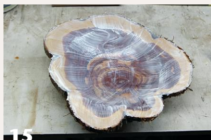
15 Since the bowl was rough-turned green, or wet, the author takes steps to dry it before final turning. First, he applies a wax emulsion sealer, then follows up with silica desiccant beads.
