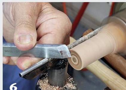
5 The author mounts the blank in spigot jaws, turns it round, and faces off the end.
