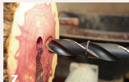
6 7 With a chucking tenon formed and the bowl blank remounted in a chuck, the author drills a depth hole using a Morse taper drill. An O-ring slid over the bit serves as a depth gauge.
