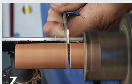
7 Use a thin parting tool to separate the box body from the lid.
