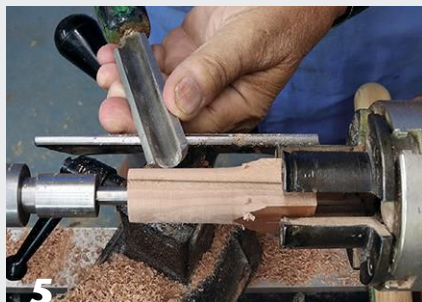
5 The author mounts the blank in spigot jaws, turns it round, and faces off the end.
