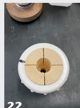
22 The face of the collet, trued and ready for use. To true the face, insert a dowel into the collet and tighten the compression nut to keep the four quadrants from flexing.
