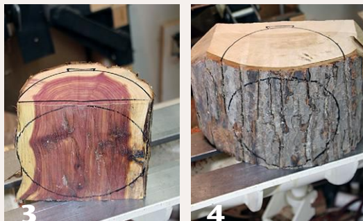
3 4 In sidegrain orientation, the turner can choose to set the rim facing the log's pith or the outer bark.
