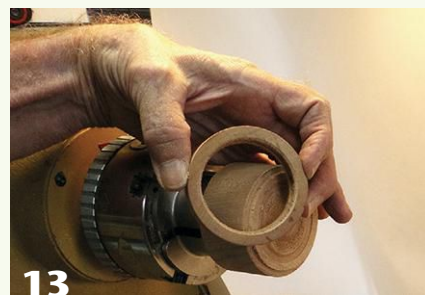
12 The author uses a parting tool to part off the mortise ring, which will later be glued into the lid.
