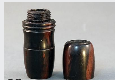
18 A completed etui container in Macassar ebony with hand-chased threads for the lid connection. For more on hand-chasing threads in wood, see Sam Angelo's June 2020 AW article, "The Basics of Hand-Chasing Threads in Wood" (vol 35, no 3, page 22).
