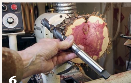
6 7 With a chucking tenon formed and the bowl blank remounted in a chuck, the author drills a depth hole using a Morse taper drill. An O-ring slid over the bit serves as a depth gauge.
