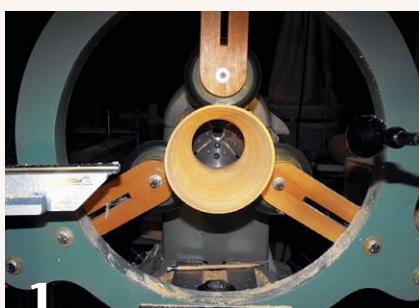
(1) The wood is hollowed in endgrain orientation to a roughly cylindrical or conical shape. A shopmade steady rest provides support.
