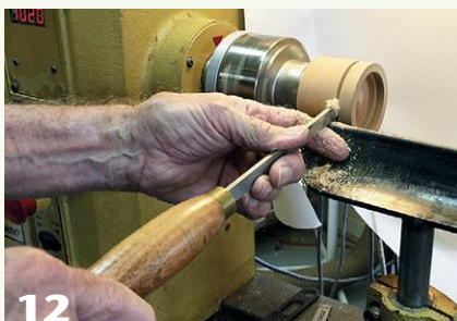
12 The author uses a parting tool to part off the mortise ring, which will later be glued into the lid.
