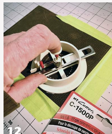
11 A caliper is used to measure the width of the recess, then the author uses a circle cutter to cut the leather to fit.
