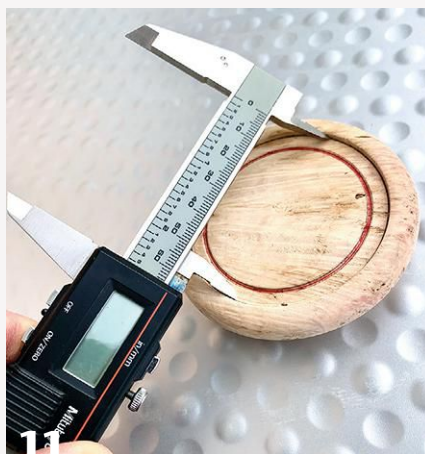
11 A caliper is used to measure the width of the recess, then the author uses a circle cutter to cut the leather to fit.
