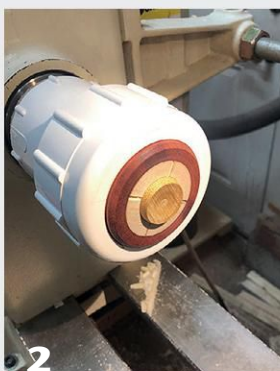
2 The chuck mounted on the lathe, ready for turning the bottom of a game piece (shown at center). The threaded PVC nut compresses the wood collet onto the workpiece.
