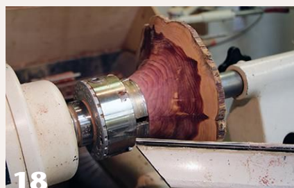
18 With the bowl remounted on the lathe, the author turns and sands it to completion.
