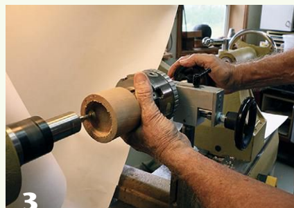
3 A threading jig provides consistent results.
