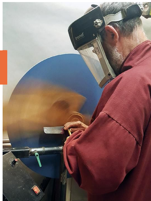
The carrier disk in these photos is 31½" (80cm) in diameter, and the irregular-shaped workpiece measures 24" (61cm) long.
