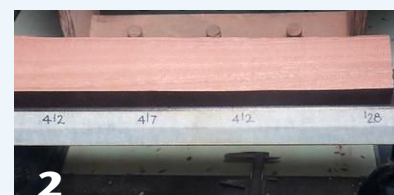
Rolling pin workpiece ready to turn. The two-stem toolrest is positioned, and a length of paper tape with reference markings is stuck to it.
