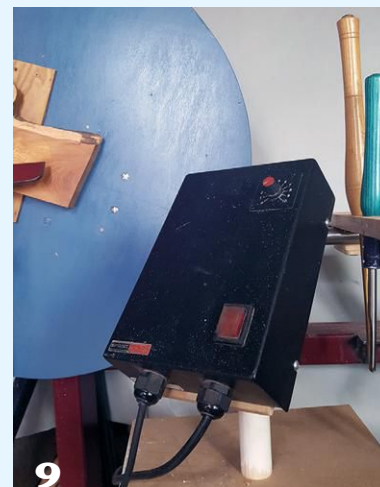
9 Ensure you can safely reach the lathe controls during turning. Never reach across or near the spinning workpiece/carrier disk. Reposition the controls as needed.
