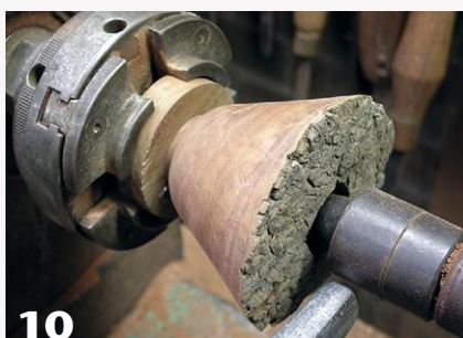
A scrap of wood is held in the chuck and a shallow recess with straight walls formed. Then the author uses hot-melt glue to temporarily affix the bowl's base in the recess. Tailstock pressure is applied during gluing and the initial phases of hollowing.
