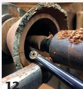
(11) A gouge is used to begin hollowing. Take care to leave the bark edge intact. A flat "step," or shoulder, is formed just below the rim to later accept the lid.
