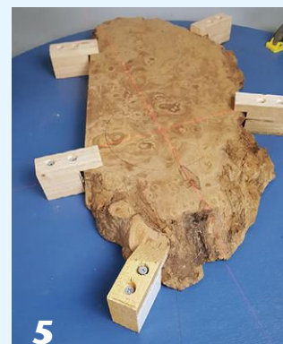
Softwood holding blocks “clamp” the workpiece to the carrier disk.
