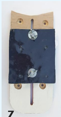
7 Back of counterbalance unit, with metal weight attached via wingnuts.
