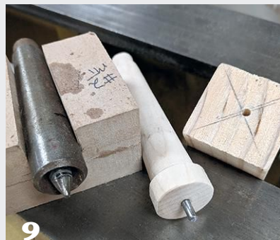
9 At left, a purchased point-and-cup drive. At right, the author's shopmade version made from wood and a short length of nail that registers in a hole in the end of the blank. Both act as safety drives that allow the wood to stop spinning in the event of a catch.
