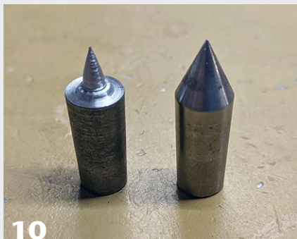
10 Tailstock live center tips. At left, the author's modified tip for mounting thin spindles; the standard 60-degree tip can split thin turning blanks.
