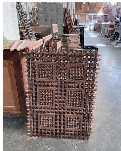
At the NADIM workshop in Cairo, a woodturner creates small spindles that will comprise large, complex mashrabiya.
