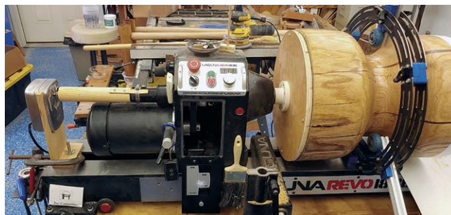
The author adapts a rotisserie motor to slowly turn the usu during epoxy coating.
