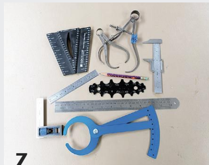
7 An assortment of good layout tools, such as calipers, rulers, squares, and diameter gauges, is essential for making a good story stick.
