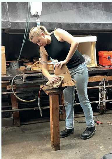
In 2022, milliner Sydney Strickler of American Hats, LLC, makes a felt bonnet using Harman Baugh's 1840s-era multiaxis-turned hat form.
