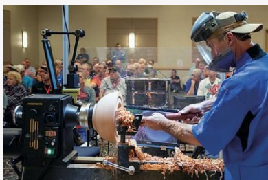
Mike demonstrating bowl coring with the McNaughton system at the 2022 AAW Symposium, Chattanooga, Tennessee.
