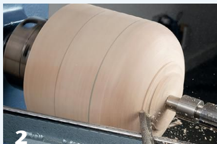
After rough-turning the work between centers, the author remounts it in a chuck and maintains tailstock support. A bowl gouge is used to first shape the top and shoulder, then the base. In both areas, extra wood is left intact for added support during hollowing.
