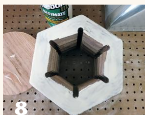
8 Prior to gluing a wasteblock to the bottom of the nut, drill six holes at the inside joints. These holes will later accept alignment keys.
