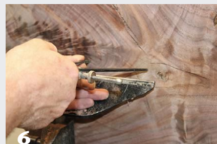
6 Use the dividers to mark the size of a chucking recess. Line up the middle of the divider's legs with the middle of the blank. Be sure to scribe very lightly with the left leg only; if the scribed line matches up with the right leg, you've got it centered.
