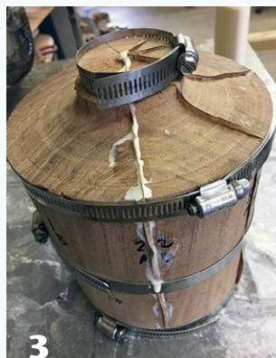
3 After dry-fitting the segments, they are glued together with paper between the joints. This allows them to be split apart later.
