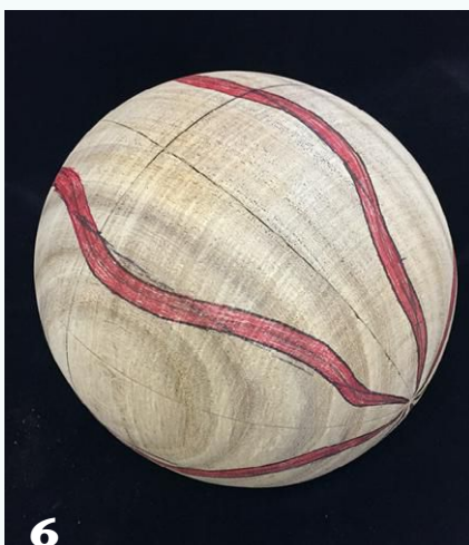
5 With the form turned to a sphere by eye, the author draws random “waves” between the glue joints.
