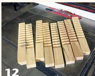
(11-12) Rip the grooved shank material into eight staves skewed to 3.5 degrees. The angle is achieved by first making an angled cut at the bandsaw, then using that side against the table saw fence.
