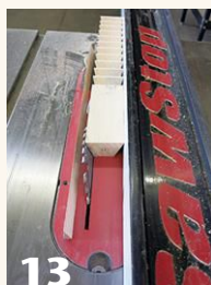
(11-12) Rip the grooved shank material into eight staves skewed to 3.5 degrees. The angle is achieved by first making an angled cut at the bandsaw, then using that side against the table saw fence.
