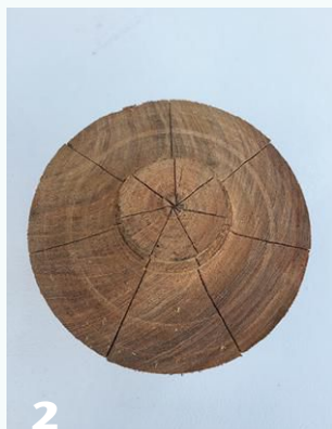
2 The segment divisions are drawn on the surfaces of the cylinder, which is then carefully cut apart at the bandsaw.
