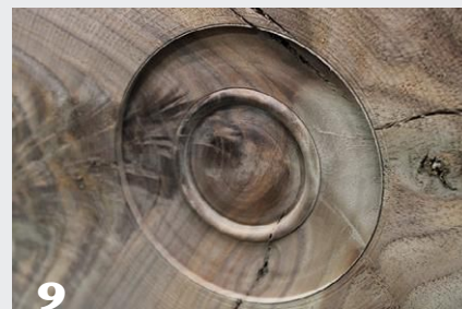
9 The waste wood in the center of the recess is turned into a decorative bead.
