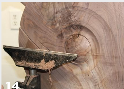
14 The author turns a fillet and cove just outside the boss to frame this decorative element.
