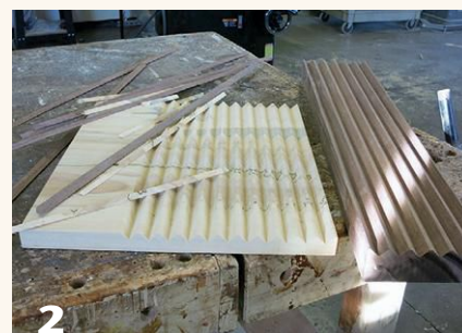
1 With the table saw blade tilted to 45 degrees, cut V-grooves that will become large screw threads.
