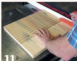
(11-12) Rip the grooved shank material into eight staves skewed to 3.5 degrees. The angle is achieved by first making an angled cut at the bandsaw, then using that side against the table saw fence.
