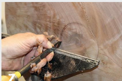
7 The author uses a parting tool to create a chucking recess on the back of the shield.
