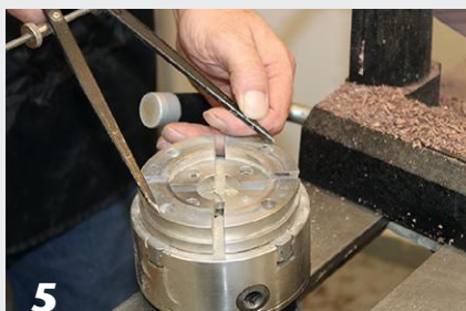
5 With the chuck jaws nearly closed, the outer diameter is gauged using dividers.
