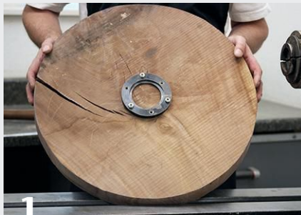
1 The author uses a faceplate ring to mount the shield blank on the lathe. A regular faceplate could also be used, but be aware of the screw-hole depth. The faceplate is mounted on the front of the shield, providing access to turn the back.
