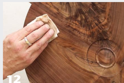
12 Apply a finish to the back before reverse-mounting the work. Here, Danish oil makes the wood's crotch grain pop.
