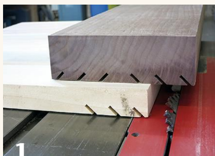
1 With the table saw blade tilted to 45 degrees, cut V-grooves that will become large screw threads.
