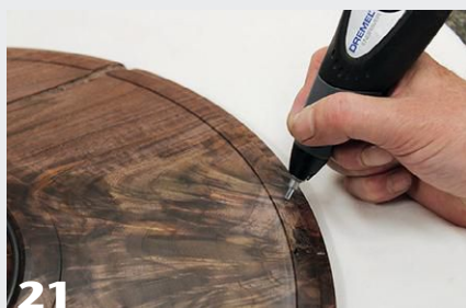
21 A rotary tool is used to add texture. A band of subtle texture next to the darkened bead leads the viewer from center outward.
