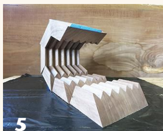
5 Tape the joints together on the outside, apply glue to the beveled surfaces, and roll the nut together, making sure the threads align. Plastic stretch wrap is used to apply gluing pressure.
