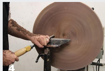
3 A bowl gouge is used to make draw, or pull, cuts to true up the back.
