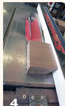
(3) Cross-cut the nut segments at a slight angle, in this case 3.8 degrees. This allows the V-groove threads to come together as one continuous thread when glued up.
