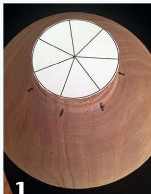
1 After turning a cylinder (not shown), the author creates a seven-segment pie chart using a spreadsheet program and uses it to mark off seven pie-shaped segments.
