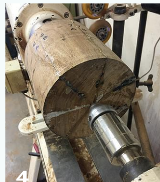
4 The glued-up cylinder remounted on the lathe. Not shown: the cylinder is turned to a sphere shape.
