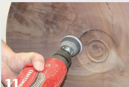
11 The author uses a drill to power-sand the back.
