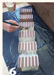
5 Tape the joints together on the outside, apply glue to the beveled surfaces, and roll the nut together, making sure the threads align. Plastic stretch wrap is used to apply gluing pressure.
