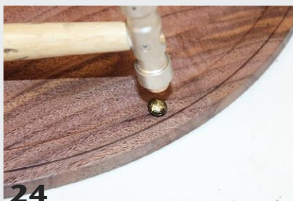
23 The author first drills holes at the rim, then taps in decorative studs.
