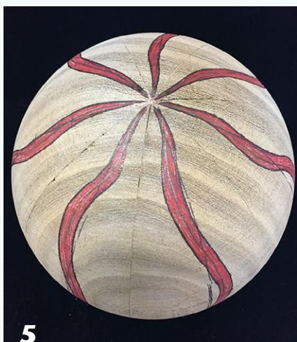
5 With the form turned to a sphere by eye, the author draws random “waves” between the glue joints.
