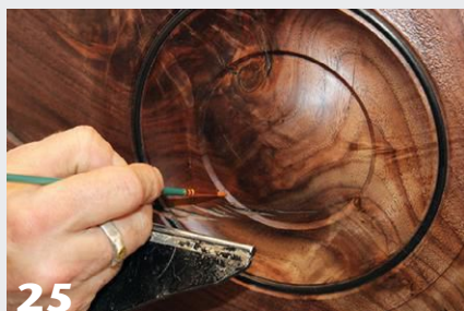
25 The center boss is adorned with 24k gold leaf. First, adhesive is applied carefully by turning the lathe by hand and keeping the brush still.
