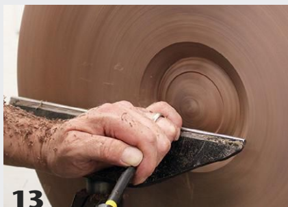
13 Remount the work on a chuck in expansion mode, using the recess you turned on the back. Turn a convex shape in the center of the front to form the shield's boss.
