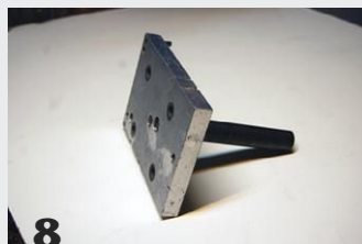
8 A support platform with banjo-mount post.
