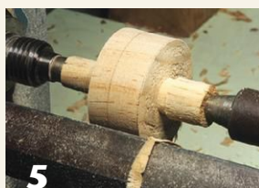
The bottom and left side of the parting-tool trench; both are badly torn.
