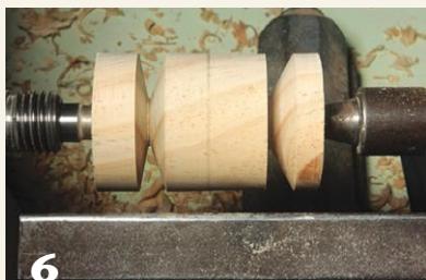
At left is a symmetrical V-groove, and at right, a canted V-groove. Both were cut with a skew's long point and are useful for defining a bead's shape and dimensions.
