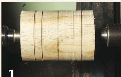
1 The inner pair of fine V-cuts mark the intended bead width. The outer fine V-cuts are \frac{3}{8} " (10mm) away.
