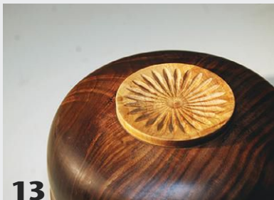
A convex and concave rosette ( Photos 12 and 13 , respectively), both routed at the lathe.
