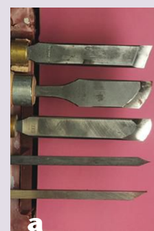
(a) Five chisels that can be used to cut V-grooves and roll beads. Top to bottom: a skew with a 70° long-point angle, a curved skew with a 90° long-point angle, a skew with a rounded long point and a long-point angle of 110°, a beading-and-parting tool, and a bedan. The latter two lack the skew's versatility and are essentially redundant.
