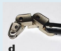
d Adjustable articulations allow for comfortable positioning of the cutter head inside a hollow form.
