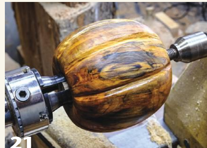
The pumpkin is placed over the jam chuck and held in place with tailstock pressure. Mounted in this way, the tenon can be turned away.
