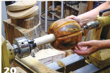
The pumpkin is placed over the jam chuck and held in place with tailstock pressure. Mounted in this way, the tenon can be turned away.
