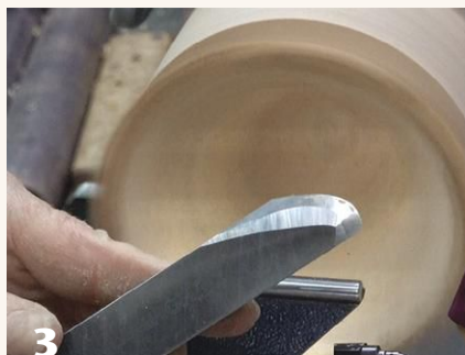
A negative-rake scraper has a bevel on the top and bottom. It is the author's tool of choice for preparing the burl surface for dye and for scraping off most of the dye from the first application.
