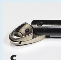
b In Photo b, the guard is fully closed—no cutting occurs. In Photo c, the guard is fully open, with about 1mm of the cutter exposed—an aggressive bite. The user can adjust the depth of cut anywhere between these two extremes.
