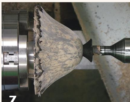
The author scrapes away most of the first application of dye. Dye remains in the endgrain areas of the burl figure, where it penetrated the wood more deeply.
