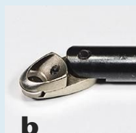
b In Photo b, the guard is fully closed—no cutting occurs. In Photo c, the guard is fully open, with about 1mm of the cutter exposed—an aggressive bite. The user can adjust the depth of cut anywhere between these two extremes.
