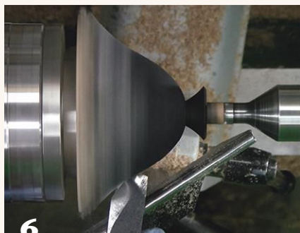
The author scrapes away most of the first application of dye. Dye remains in the endgrain areas of the burl figure, where it penetrated the wood more deeply.
