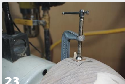
With glue applied, set the inlay into the recess. If the patch is near the bowl rim, a clamp will do the job; if not, gently tap in the inlay.
