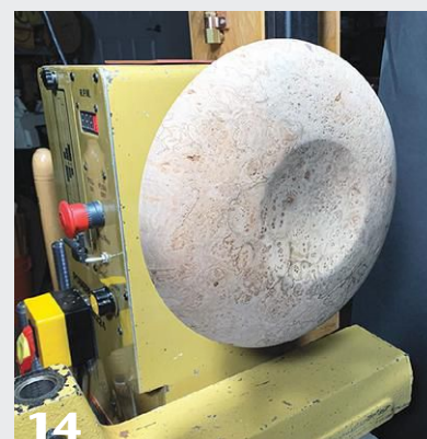
14 With the base remounted once again, turn away the expansion recess in the top, leaving a concave depression with a final thickness ⅛" or less in the center. Finish shaping the top of the base.
