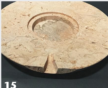
Carve a channel on the bottom of the base to accommodate the adaptor plug and wires. Test-fit the electromagnet and adaptor plug before applying a finish.
