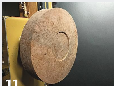
11 The base is turned to overall size, with an expansion recess turned on top.
