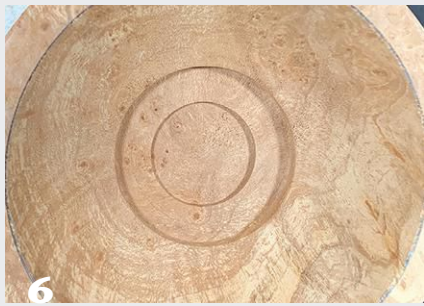
6 A stepped recess inside the bottom of the sphere accepts the magnet. The deepest part of the recess stops \frac{1}{4} " from the bottom of the sphere.
