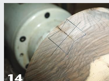
Scribe around the inner portion of the pattern to mark the placement of the butterfly inlay.
