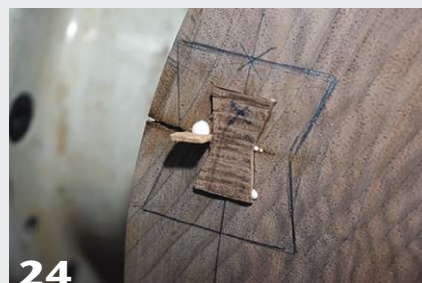
A wood wedge, or splinter, is used as a dam to prevent glue from squeezing into the crack.
