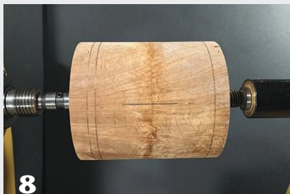
8 The two hollowed halves are glued back together with wood grain carefully aligned. Clamp the pieces between centers and allow the glue to cure.
