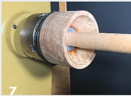
7 Glue and clamp the magnet in place, using tailstock pressure with a length of scrap wood.
