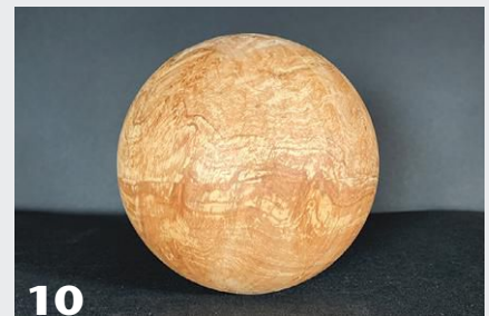
9 Turn the sphere, being sure to stick to the predetermined diameter (in this case, 4\frac{1}{2} "). The glue line is nearly imperceptible.
