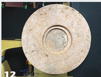
12 With the base remounted in the chuck in expansion mode, turn a stepped recess in the bottom to accept the electromagnet. The base is scooped slightly (made concave) to allow for a good fit of the chuck in expansion mode in the wider recess.
