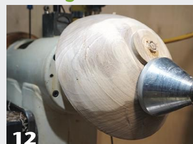
12 Mount the bowl (on or off the lathe) in such a way that the cracked work area is horizontal.
