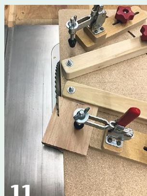
Always register the top, or wide, end of the stave against the fence—never the smaller end. Adjust the hold-down position and clamp the stave in place. Use a steady, even pressure to cut the first side.
