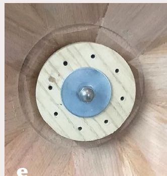
a A simple shopmade drawbar comprises all-thread rod and a centering cone.
