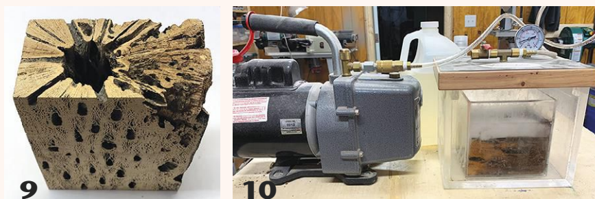
Stabilizing wood is not the same as casting, but it is a good idea to stabilize punky wood prior to casting it. Here, a vacuum pump “pulls” stabilizing solution into the wood pores. It is then baked to a hardened, useable state.
