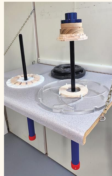
The Stomper, designed by Lloyd Johnson of Woodturner Pro. This jig aligns segment rings for accurate blank assembly. Above: in use with a Seg-Easy plate developed by Jerry Bennett; right: in use with a Longworth chuck.
