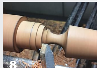
A central line indicates the left edge of the cove and the right edge of an angled cut, which is formed with a skew.
