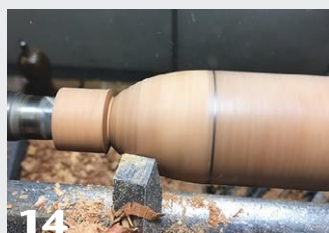
14 Shaping the end of the handle aids in gauging its overall shape as you transition the upper end of the handle into the cove.
