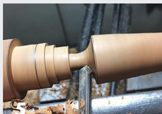
A spindle gouge is used to shape the right half of the cove under the blade.
