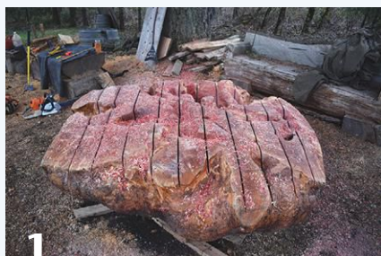
1 With the stump burl upside down, the author lays out slabs and cuts only part of the way in.
