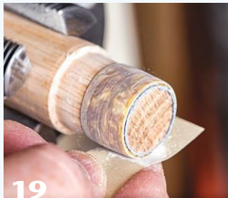
19 The outside of the ring is turned, sanded, and parted to a custom width.
