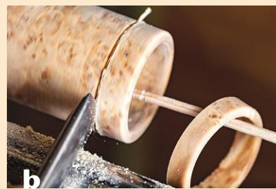
The author turns and hollows a cylinder of burl, then parts away multiple rings. A thin dowel held in the cylinder catches the rings as they come off.
