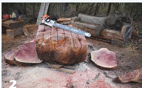
2 A sharp chain ensures straight cuts the rest of the way through. Slabs are cut off each side in alternating fashion to keep the work balanced.
