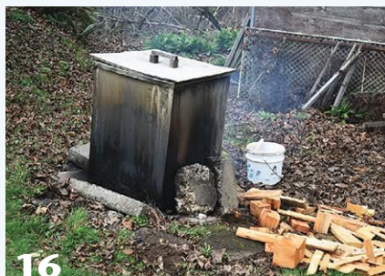
The author's boiler, a homemade stainless-steel tank heated with firewood. Boiling the rough-turned madrone helps to stabilize it so it won't crack during drying.
