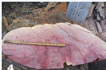
4 Circles of varying sizes are drawn on each slab using a large compass. The best burl figure is positioned for maximal effect.
