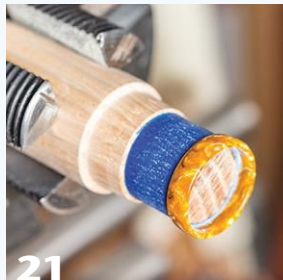
The author cleans up the ring's edge by partially mounting it on the mandrel.
