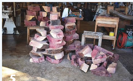
5 The blanks are first rough cut with a small chainsaw and then made round at the bandsaw.
