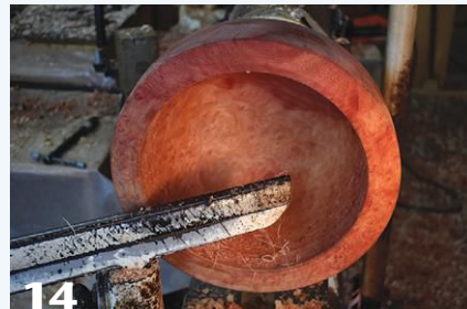
The bowl walls are then rough-turned to consistent thickness.
