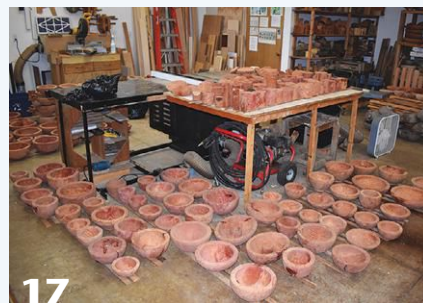
The boiled bowls are set out to dry, and a box fan circulates the air. Now the time pressure is off. The bowls can take months to dry, but they can be finish-turned at any time.
