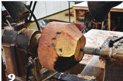
9 This blank's lower half was rough-shaped using an electric chainsaw to further improve its balance on the lathe.
