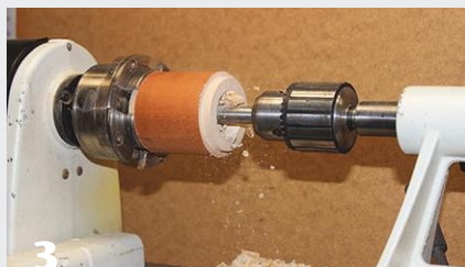
3 Drill halfway into the dowel, then widen the hole using a hollowing tool. Stop the lathe and confirm a snug fit of the hose or tool fitting. Flip the adapter around in the chuck and repeat the process for the other side.
