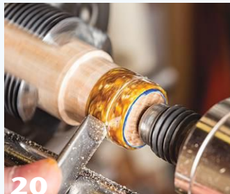
19 The outside of the ring is turned, sanded, and parted to a custom width.
