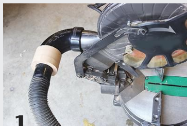
1 The author turned a wood adapter to connect his dust hose to a 2" PVC elbow attached to his miter saw. The adapter fits over , not into , the hose and PVC fitting.
