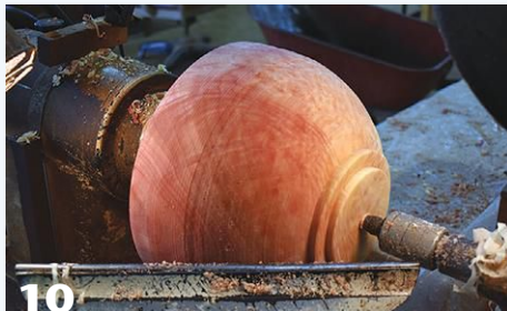
10 The outside profile is shaped using a bowl gouge. Note the chucking tenon on the foot. Since this project involves batch processing, several bowls are turned to this stage before proceeding.
