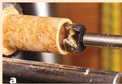
The author turns and hollows a cylinder of burl, then parts away multiple rings. A thin dowel held in the cylinder catches the rings as they come off.
