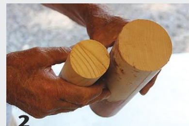
2 Store-bought 2"- and 3"-diameter dowels are perfect for making most hose adapters.
