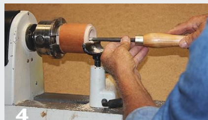
3 Drill halfway into the dowel, then widen the hole using a hollowing tool. Stop the lathe and confirm a snug fit of the hose or tool fitting. Flip the adapter around in the chuck and repeat the process for the other side.
