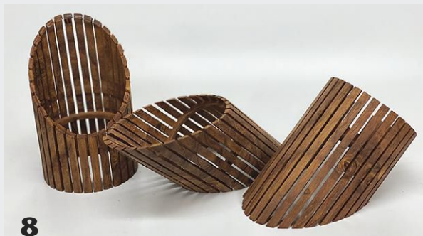
The 12"-tall cylinder is cut to precise angles using an Incra jig at the bandsaw.
