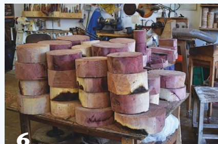
5 The blanks are first rough cut with a small chainsaw and then made round at the bandsaw.
