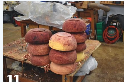
10 The outside profile is shaped using a bowl gouge. Note the chucking tenon on the foot. Since this project involves batch processing, several bowls are turned to this stage before proceeding.
