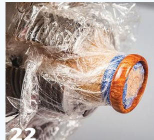
Plastic wrap keeps the ring from getting stuck on the mandrel during finishing.
