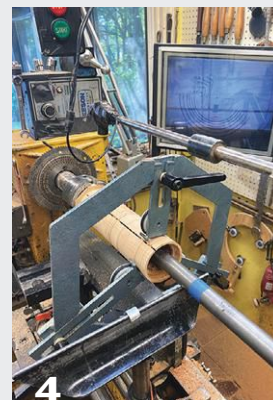
The cylinder is slotted and hollowed.
