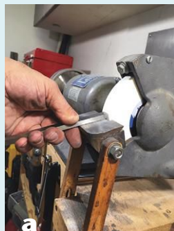
The typical method is to present the scraper cutting edge up (left). The author takes the opposite approach (right) and prefers the burr produced in this manner.
