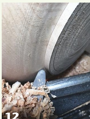
12 Again, the roundnose scraper is used to ease the transition to the foot and under the rim.
