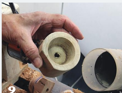
9 The author's shopmade cup chuck, turned from scrap wood.
