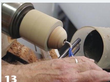
12 Before hollowing the second half, give the sphere a tap with a dead-blow hammer to ensure a snug fit. Then hollow the second half as you did the first half.
