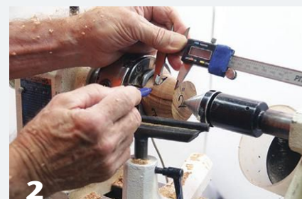
2 Rough the cube round, then measure and mark the centerline.
