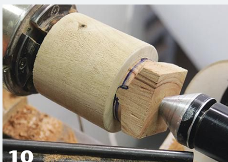
10 Insert the rounded half-sphere into the cup chuck, and hold it in place with the tailstock. Turn the second half of the sphere, again cutting from centerline toward the tailstock.
