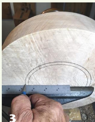
3 After truing up the face of the blank, the author marks lines to relieve the foot.
