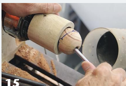
15 The lathe's knock-out bar is useful for removing the sphere from the cup chuck.
