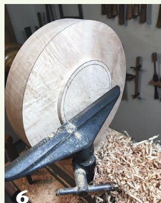
5 Use a square-end scraper to make plunge cuts up to the pencil lines.
