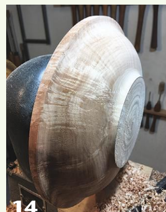
12 Again, the roundnose scraper is used to ease the transition to the foot and under the rim.
