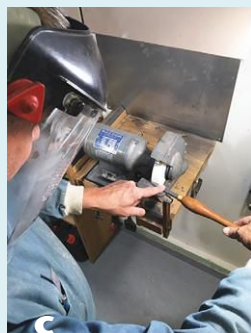
The roundnose scraper must be swung 180 degrees in a fluid motion. Press the tool flat on the toolrest using your finger.
