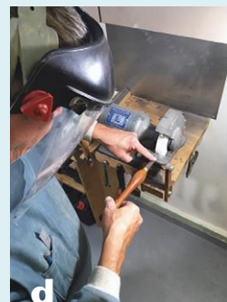
The roundnose scraper must be swung 180 degrees in a fluid motion. Press the tool flat on the toolrest using your finger.
