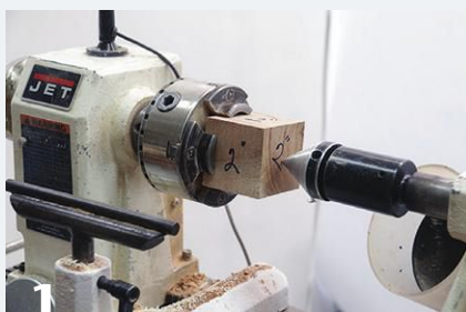
1 The sphere begins as a cube mounted in a scroll chuck.
