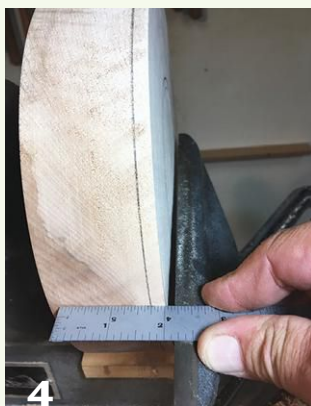
3 After truing up the face of the blank, the author marks lines to relieve the foot.
