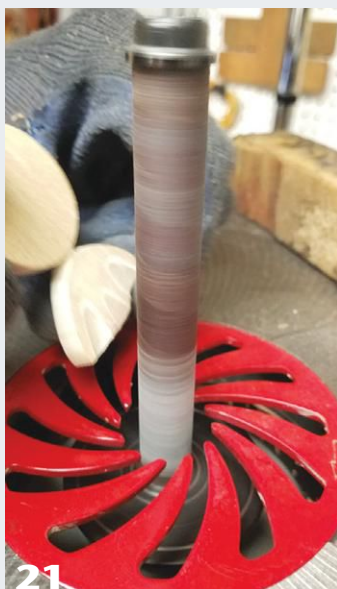
A disk and spindle sander help to shape the "cellophane" wrapper.
