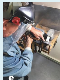
The roundnose scraper must be swung 180 degrees in a fluid motion. Press the tool flat on the toolrest using your finger.
