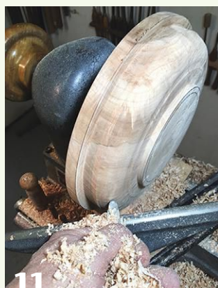
11 With the foot and rim defined, use a roundnose scraper to round off the bowl's profile.
