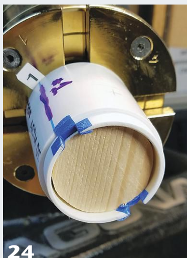
24 (24) The author's shopmade PVC candy holder. Note the backing inside the PVC, which prevents the ornament from going off center, and the notches to accommodate the twisted wrappers.
