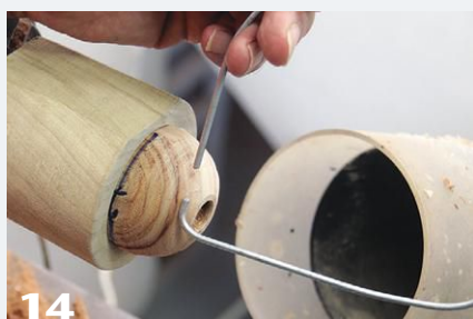
14 The author's shopmade thickness gauge can be made from a wire coat hanger. Bend the wire so the ends are facing each other and \frac{1}{2} " apart.
