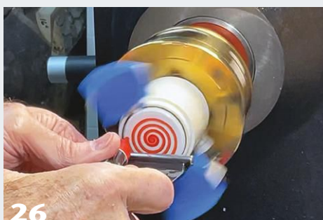
26 (25-26) The ornament is held in the PVC chuck and spun at a very slow lathe speed. A red paint pen moved along the toolrest from center to edge creates the candy's spiral.
