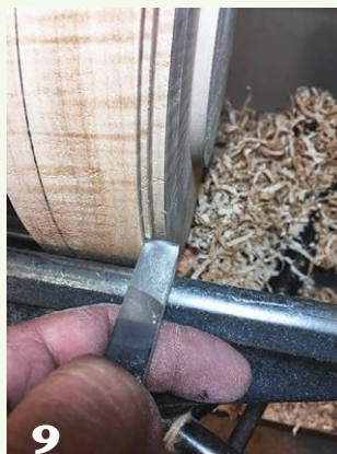
9 Use a square-end scraper, approaching from the outer edge, to remove wood from within the pencil lines.
