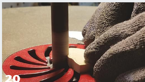
A disk and spindle sander help to shape the "cellophane" wrapper.
