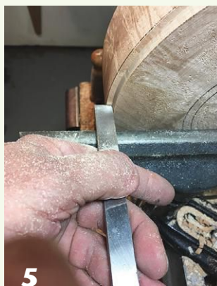
5 Use a square-end scraper to make plunge cuts up to the pencil lines.
