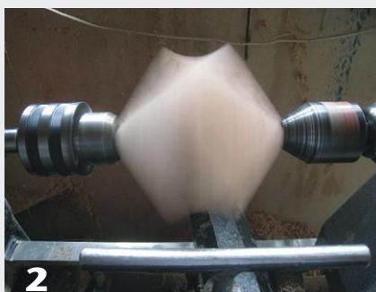
1 The cube is mounted between centers, corner to corner, using a drill chuck in the headstock as a drive and a live center cup in the tailstock.
