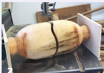
2 The turned form is cut in half crosswise at the bandsaw. Note the square plywood pieces attached to the ends for safe cutting.
