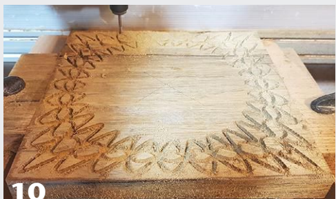
The grooves in this square platter were cut using a three-axis CNC machine. Patterned slots were formed at the perimeter from above, and then at the center of the platter—in the bowl portion—from below.
