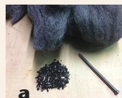
(a) Iron components that can be added to vinegar to make an ebonizing solution—in this case, steel wool, iron filings, and an iron nail.
