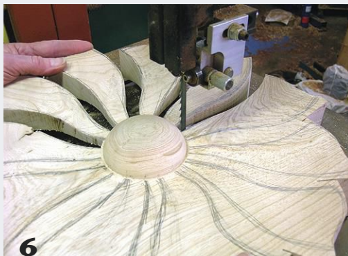
The waste material between the fins is cut away at the bandsaw.
