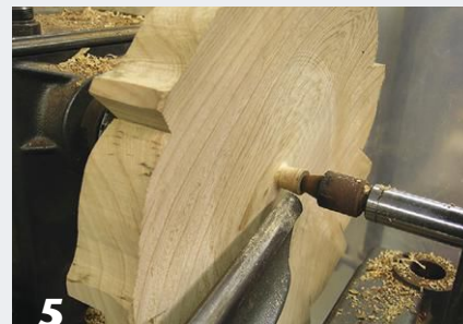
4 A scrap block makes a good jam chuck. In this case, it is hollowed to accept the hemisphere on the front of the sculpture. This allows the author to reverse-mount the piece, with tailstock support, so he can shape the back.
