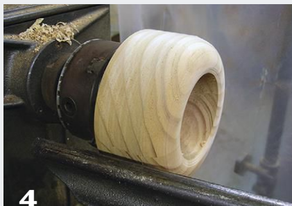
4 A scrap block makes a good jam chuck. In this case, it is hollowed to accept the hemisphere on the front of the sculpture. This allows the author to reverse-mount the piece, with tailstock support, so he can shape the back.
