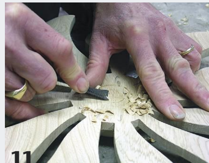
9 Hand-sanding, filing, and carving complete the form and make it ready for finish—in this case, wipe-on polyurethane.
