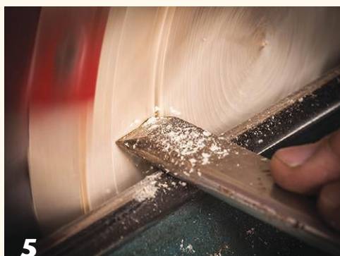
5 Using a skew chisel presented flat on the toolrest, the author forms a shallow spigot. Just \frac{1}{8} " depth is enough with a tenon this wide.
