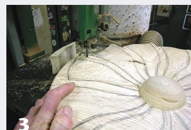
3 "Fins" are drawn onto the wood freehand. Then a bandsaw is used to cut the ends accordingly.
