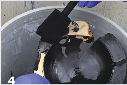
4 The author applies a first coat of black dye using a foam brush. Flood the surface and allow the dye to be absorbed into the open wood grain.
