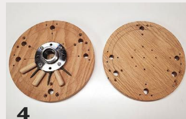
4 Two endplates are drilled for pivot dowels as well as for spindle mounting screws, all spaced inside the “footprint” of the spindle turning blocks. A faceplate is used to mount the rig on the lathe.
