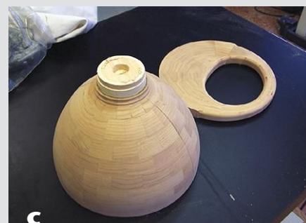
A traditional ring-segmented bowl is turned, with an extra ring pressed (but not glued) to the rim with the tailstock. After it is turned flush, the extra ring is removed and cut into the shape of a basket handle.
