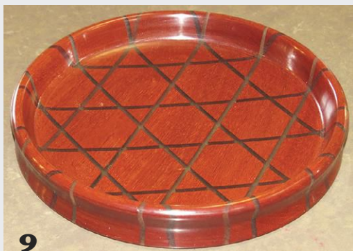
This platter, with multiple Stars of David, began as a hexagonal blank. Each of the six sides was registered against the table saw fence so parallel grooves could be formed.
