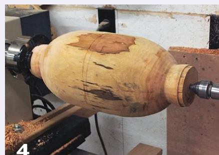
4 The two hollowed halves are glued back together, resulting in a fully enclosed oblong hollow form.
