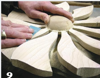
9 Hand-sanding, filing, and carving complete the form and make it ready for finish—in this case, wipe-on polyurethane.
