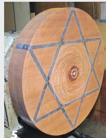
5 (5) After the epoxy has cured, the piece is remounted on the lathe and turned. Not shown: Reverse-mount the platter to turn away the remaining wood under the grooves, leaving distinct segments held together only by the epoxy.
