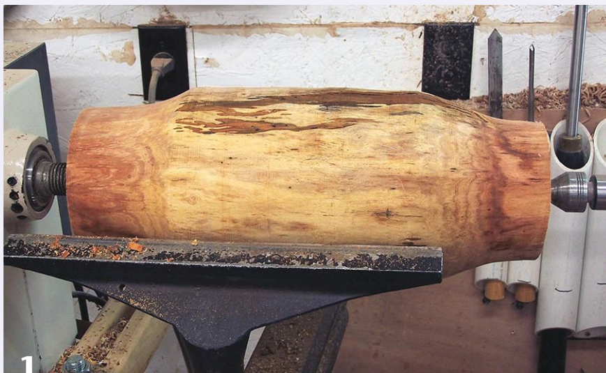
1 Starting with a mahogany log 18" long, the author turned the outside profile of an oblong bowl, knowing the piece would eventually be cut in half to make two identical bowls. He also turned a tenon at each end.
