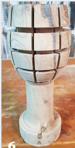
The horizontal grooves in this wine glass, or goblet, were formed on the lathe, and the vertical grooves were cut at the table saw. The slots are sealed with tape, the epoxy poured, and the form turned to final shape.
