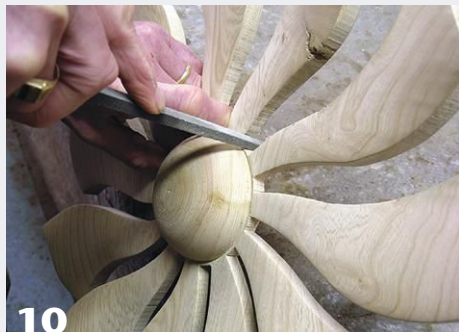
9 Hand-sanding, filing, and carving complete the form and make it ready for finish—in this case, wipe-on polyurethane.
