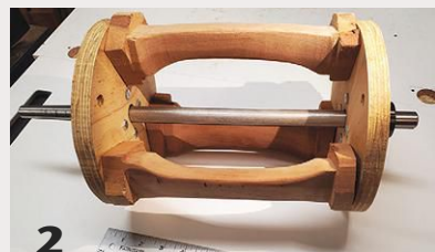
2 A therming rig with center shaft.
