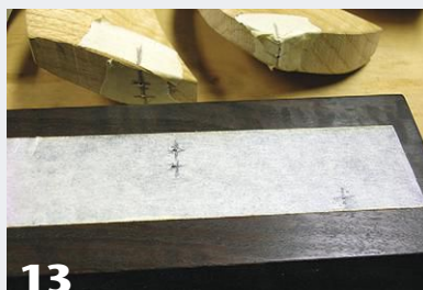
13 The author opts for three small pins to mount the work to its ebonized red gum base. Brads are driven into the ends of two fins and are then used to mark drilling locations on the base.
