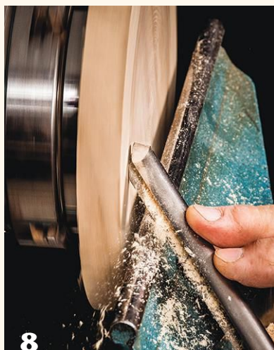
8 The author shear-scapes the top of the plate using the left wing of a bowl gouge and the tool handle held low.
