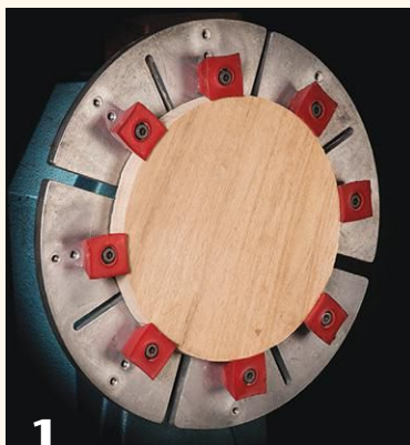
With a precut ¾"-thick blank mounted on bowl jaws, true the surface using a pull cut.
