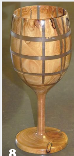
The horizontal grooves in this wine glass, or goblet, were formed on the lathe, and the vertical grooves were cut at the table saw. The slots are sealed with tape, the epoxy poured, and the form turned to final shape.
