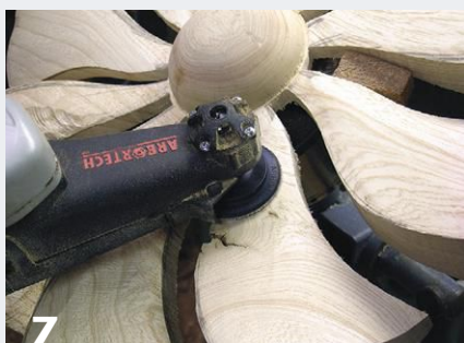
7 Cork wedges are inserted between the fins during power-carving to help dampen vibration. The juncture where fin meets hub is narrow and fragile, with the grain running either directly across or at an angle to the fin.
