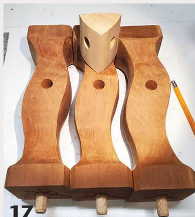
17 The author made a triangular center block, attached to the legs with separate dowels, for added stability (shown in the lead image).
