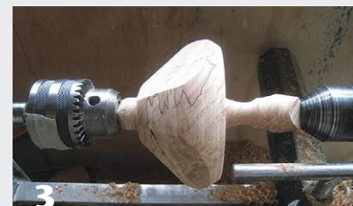
3 Cutting "downhill" toward the headstock, the author forms the outside profile of the bowl. Since the initial block was a cube, three flats remain. A small tenon is formed at the base, and waste wood at the tailstock end is turned away.
