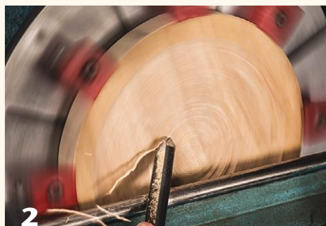
With a precut ¾"-thick blank mounted on bowl jaws, true the surface using a pull cut.
