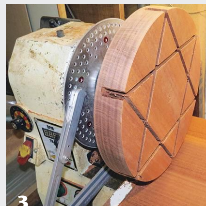
3 The six linear grooves that make up the Star of David, formed using a \frac{1}{4} "-diameter cutter, are completed in multiple light passes. The indexing wheel is used to ensure precise angular positioning; in this case, the lines are 60 degrees apart.
