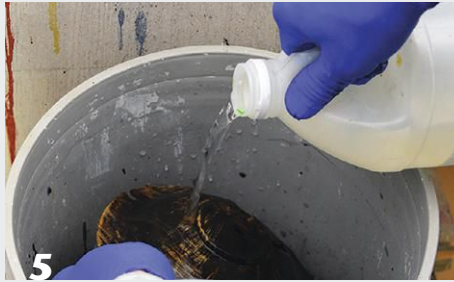
5 Rinse the workpiece with clean water to wash away excess dye from the surface. Then wipe off as much of the black dye as you can using clean paper towels. Rinse again and blot dry.
