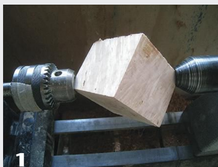
1 The cube is mounted between centers, corner to corner, using a drill chuck in the headstock as a drive and a live center cup in the tailstock.
