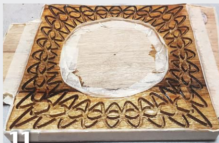
The grooves in this square platter were cut using a three-axis CNC machine. Patterned slots were formed at the perimeter from above, and then at the center of the platter—in the bowl portion—from below.
