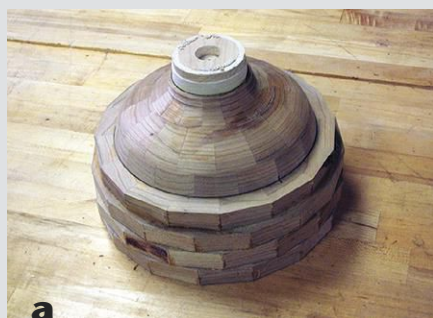
A traditional ring-segmented bowl is turned, with an extra ring pressed (but not glued) to the rim with the tailstock. After it is turned flush, the extra ring is removed and cut into the shape of a basket handle.
