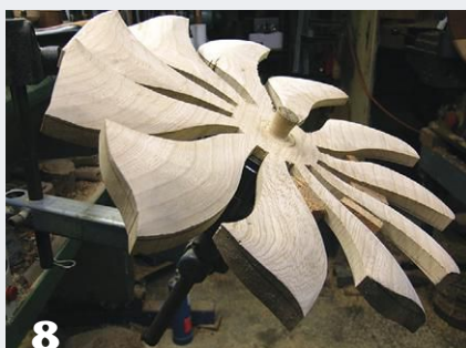
8 The piece is reversed on the carving mount so the back can be carved and sanded as well.
