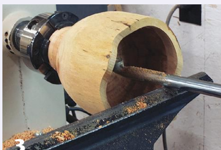
3 Each end is mounted on the lathe in a chuck and hollowed.
