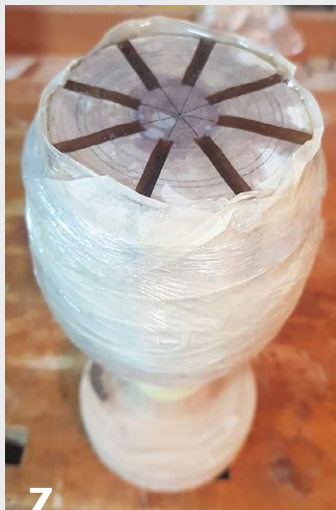
The horizontal grooves in this wine glass, or goblet, were formed on the lathe, and the vertical grooves were cut at the table saw. The slots are sealed with tape, the epoxy poured, and the form turned to final shape.
