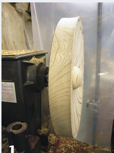
1 The author starts by turning a disk of ash, slightly scooped on the front face, with a hemisphere protruding at the center.
