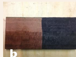
(b) A sample of red gum, half natural and half ebonized using a shopmade brew. A clear finish was applied to the bottom half of both sides.
