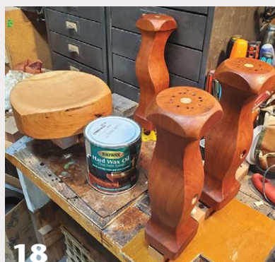
18 Finish is applied, then buffed, prior to assembly. The legs are mounted to the seat bottom using dowels.
