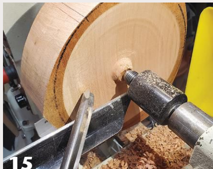
15 The seat block is mounted on a chuck by expanding the jaws into a drilled recess on the bottom. Turn a dish-shaped profile in the top of the seat for added comfort.
