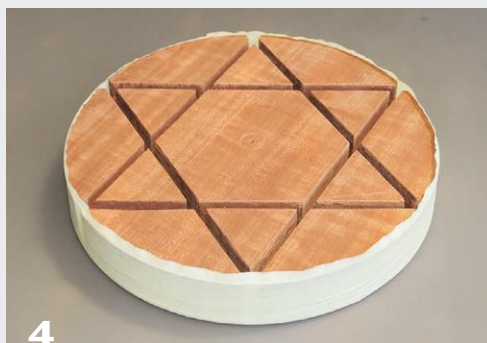
4 (4) Masking tape applied around the edge of the workpiece acts as a dam during the epoxy pour.
