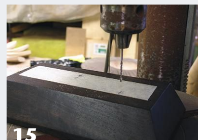
15 With the brads removed, the author drills final holes for stainless-steel mounting pins.
