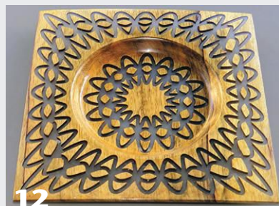
The grooves in this square platter were cut using a three-axis CNC machine. Patterned slots were formed at the perimeter from above, and then at the center of the platter—in the bowl portion—from below.
