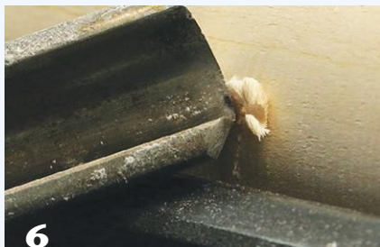
With the spindle-roughing gouge held straight on to the wood (90 degrees), a peeling cut results. When you angle the gouge (either left or right), the cutting edge shears the wood fibers and results in a cleaner surface.
