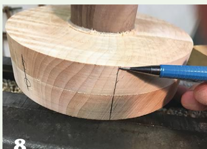
8 Carry the hole locations from one base to the other. Use an awl to indent the hole locations deep enough to remain after sanding.
