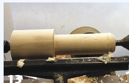
The A-B-C approach applies to the skew as well. Anchor the tool with the handle low, rub the bevel without cutting, then lift the handle until the cutting edge engages the wood. The peeling cut goes straight in, removing wood quickly.
