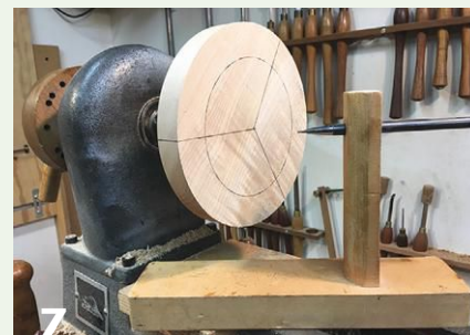
7 Draw a circle that identifies the distance of the holes from the center. Then, using a jig that holds a pencil at center height, mark the hole locations.
