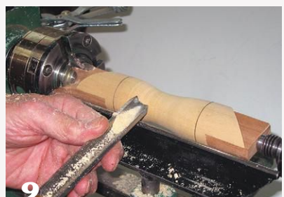
Turn the spindle round, then add features as desired. The author finds the center of the spindle, defines its depth, and then forms a long cove. A burn line is also added at the center of the cove (not shown).
