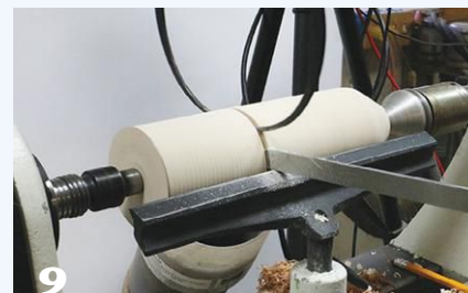
The author uses a spring caliper to gauge and transfer key dimensions.
