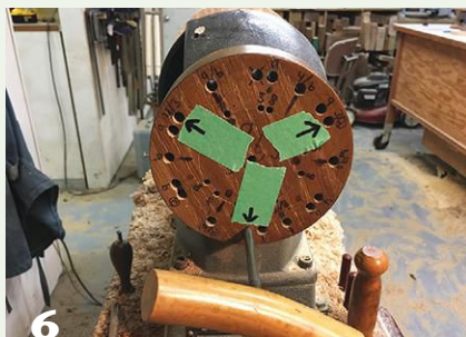
6 Tailstock view. Use the indexing head on your lathe to divide the circle into three sections.
