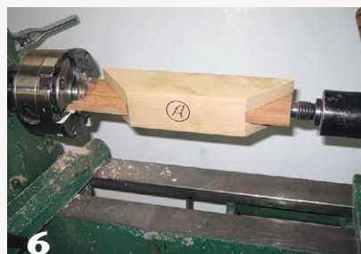
To mount the mitered workpiece on the lathe, a filler block is used at each end. The drive-end block is held in a chuck and features a short nail filed to a point for positive registration inside the slotted miter cut.
