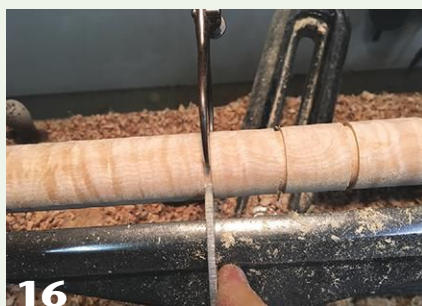
16 Make several parting cuts along the spindle to your desired diameter, checking with a caliper, then use a spindle-roughing gouge to "connect the dots."
