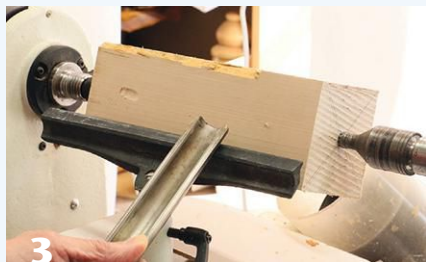
The A-B-Cs of woodturning. Anchor the tool on the toolrest with the handle held low, rub the Bevel without yet cutting, and lift the handle to engage the Cut.
