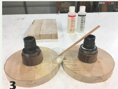
3 The author mounts both bases on separate faceplates with glueblocks.
