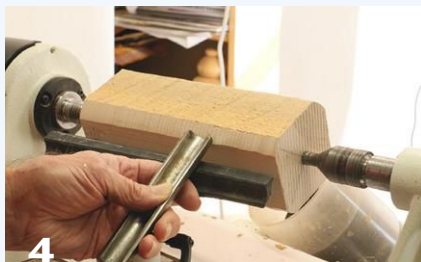
The A-B-Cs of woodturning. Anchor the tool on the toolrest with the handle held low, rub the Bevel without yet cutting, and lift the handle to engage the Cut.
