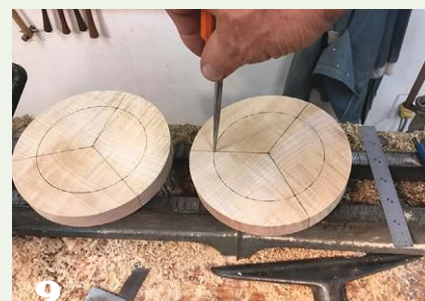
8 Carry the hole locations from one base to the other. Use an awl to indent the hole locations deep enough to remain after sanding.
