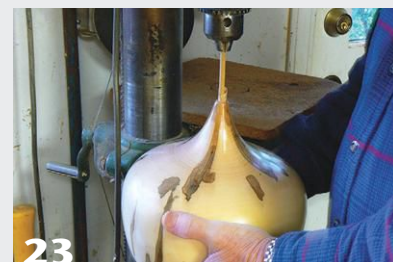
23 A custom flap-sander made from a dowel reaches inside the spout.
