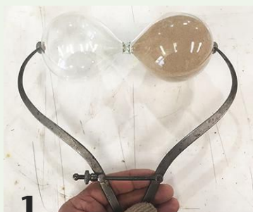
Measure the length and largest diameter of the glass you will be using. Draw a plan to determine base and spindle dimensions.
