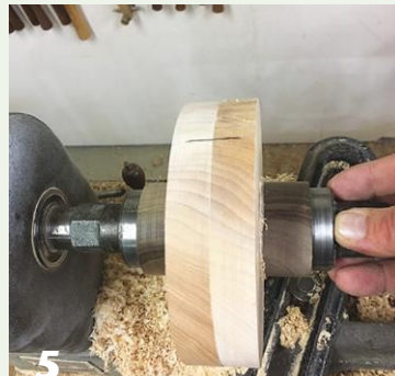
(4, 5) Turn the bases to their final diameter, compare for good measure. A reference mark across both bases indicates grain alignment, as these pieces came from the same board.
