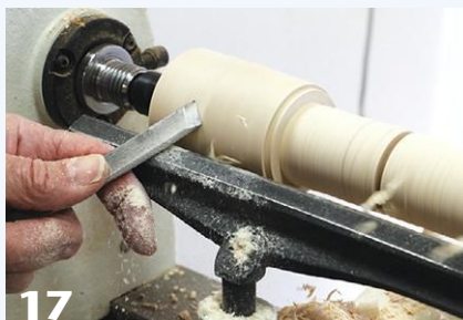
A planing cut with a skew does a nice job of tapering the mallet head, shearing the wood fibers to a smooth finish.
