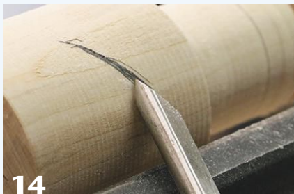
A pencil line at a 45-degree angle indicates the correct angle of the skew's cutting edge. Rub the bevel first, then lift the handle to begin cutting (in this case, left to right).
