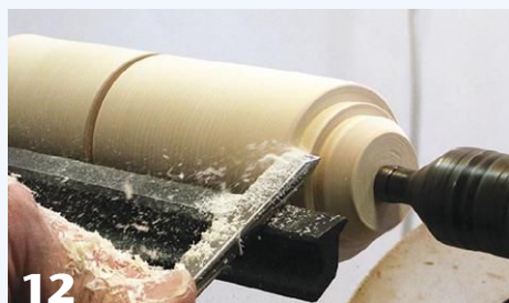
The A-B-C approach applies to the skew as well. Anchor the tool with the handle low, rub the bevel without cutting, then lift the handle until the cutting edge engages the wood. The peeling cut goes straight in, removing wood quickly.
