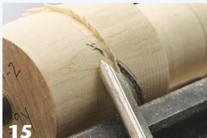
A pencil line at a 45-degree angle indicates the correct angle of the skew's cutting edge. Rub the bevel first, then lift the handle to begin cutting (in this case, left to right).
