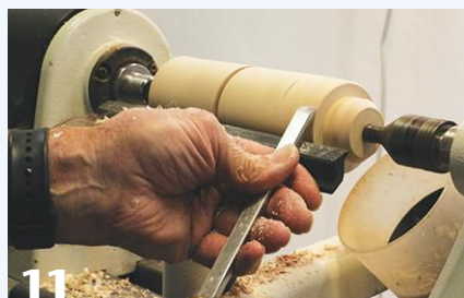
The A-B-C approach applies to the skew as well. Anchor the tool with the handle low, rub the bevel without cutting, then lift the handle until the cutting edge engages the wood. The peeling cut goes straight in, removing wood quickly.
