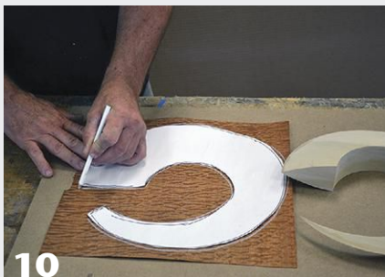
10 A slightly oversized paper template of the sculpture surface is transferred to the veneer, which is then cut out.
