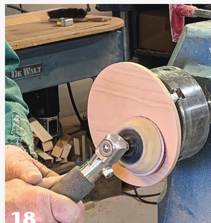
17 With the lid now mounted in a chuck in expansion mode, the author turns and sands the top of the lid.
