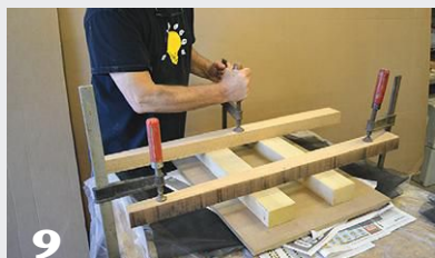
9 The conditioned veneer, together with the fiberglass screen material and newspapers, is compressed between sheets of plywood. Clamping cauls help to distribute pressure.
