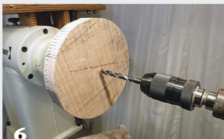
6 Drill a pilot hole for a screw chuck in the top of the base. Then turn a flat in the center 3" to 4" wide.
