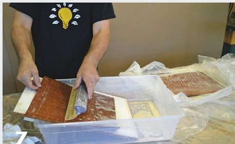
7 The conditioner is squeegeed off the veneer, which is then sandwiched between layers of window screen material and newspapers.
