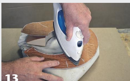
13 Heat from an iron is applied first between the markings indicating the "pleat" locations and then on those markings. The softened veneer is flexible enough to flatten onto the sculpture's compound curve.
