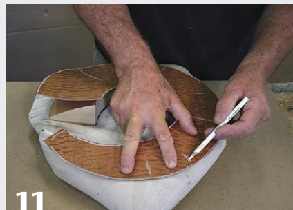
11 A pillowcase filled with sand helps support the workpiece, as the author marks where the veneer buckles due to the compound curve.
