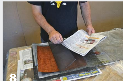
7 The conditioner is squeegeed off the veneer, which is then sandwiched between layers of window screen material and newspapers.
