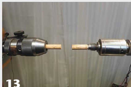
13 The lamp shaft parts with \frac{1}{2} " center holes are mounted between centers on \frac{1}{2} " wooden dowels.
