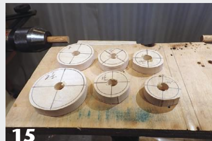
15 Wasteblocks cut from \frac{1}{2} "-thick plywood with a \frac{1}{2} " hole in the center. These blocks serve as size references, similar to mandrel bushings in pen turning.
