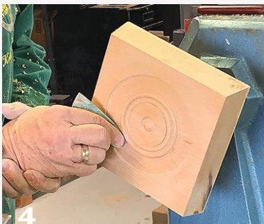
3 With the box mounted on a screw chuck, form a chucking recess in the bottom. Decorate and sand.
