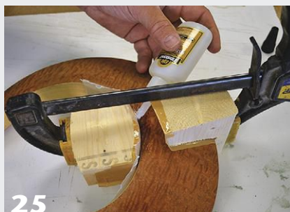
25 Custom clamping blocks, aka a compression mold, help to apply localized pressure, as a stubborn section of veneer is re-glued.
