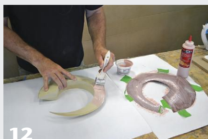
12 PVA glue is applied to both the veneer and substrate.
