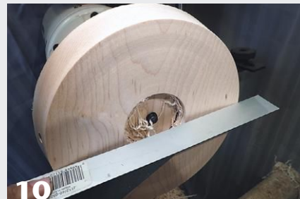
9 Use a bowl gouge and shear-scrapers to turn the bottom of the lamp base. After truing up the outside edge, form a concave surface in the middle. A straightedge touching only the outer edges indicates concavity.
