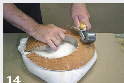
14 A cool steel roller draws heat away from the glue and ensures thorough adhesion.
