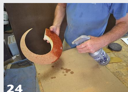
24 The author sprays the veneered form with a shellac/alcohol mixture, which reveals sanding marks and protects the surface during repair/touch-up.
