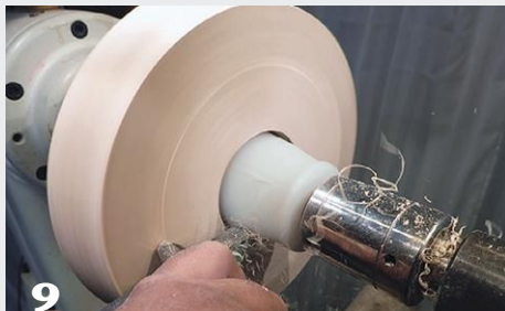
9 Use a bowl gouge and shear-scrapers to turn the bottom of the lamp base. After truing up the outside edge, form a concave surface in the middle. A straightedge touching only the outer edges indicates concavity.
