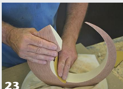
23 Sand carefully to avoid breaking through the thin veneer.
