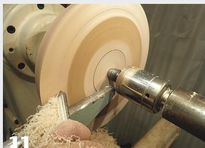
11 With the base now re-mounted on the chuck in expansion mode, mark a 2\frac{1}{2} "-diameter circle in the middle of the top. Create a concave area within this circle, then shape the remainder of the top.
