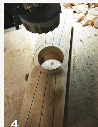
4 A Forstner bit will give you a flat bottom with a little dimple in the center. A large bit can grab and spin the piece out of your hands, so clamp the blank to the drill press table.
