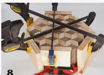
8 The author surrounds a core with additional cells, widening the diameter of the blank.
