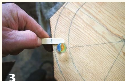
3 The author gauges the size of different objects to embed—a marble and a coin. This helps to confirm the projected wall thickness of the vessel and the depth the hole should be drilled.
