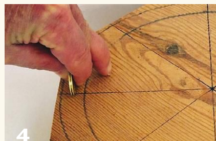
3 The author gauges the size of different objects to embed—a marble and a coin. This helps to confirm the projected wall thickness of the vessel and the depth the hole should be drilled.
