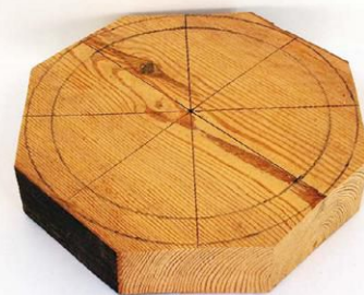
2 The flat parallel sides of an octagon make for even hole spacing and easy drilling.
