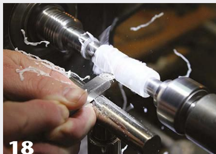
Use sharp tools when turning acrylics. Shape the pen barrels, sand, finish, and assemble.
