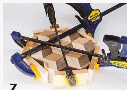
7 From a separate example, 2"-tall cells are glued into a seven-cell core.
