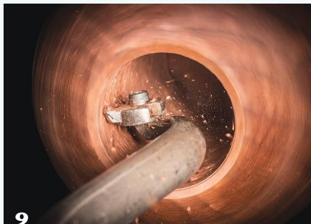
(8) The hollowing begins by drilling a hole with a large sawtooth bit.
