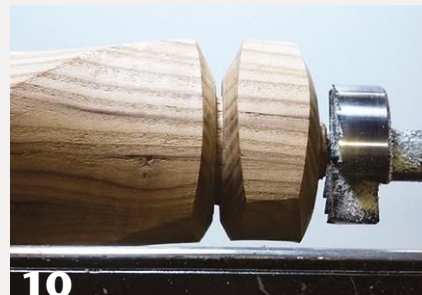
10 Drill through the napkin ring until it is cut free.
