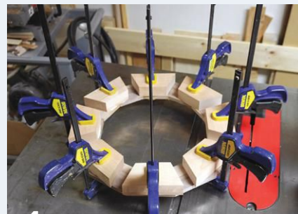
3 Segmented rings are fabricated to sandwich the wheel spacers. Save the fancy wood for the front-facing layer, as the back will be unseen, against a wall.
