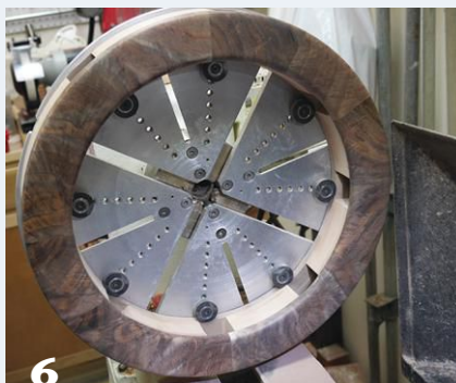
5 The glued-up wheel assembly is mounted on large plate jaws in expansion mode. Turn and sand one side, then flip the wheel around on the chuck to access the other side.
