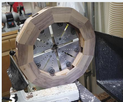
5 The glued-up wheel assembly is mounted on large plate jaws in expansion mode. Turn and sand one side, then flip the wheel around on the chuck to access the other side.
