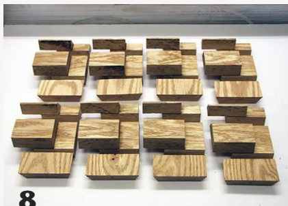
8 Components of all eight staves are glued up in pairs before final assembly.
