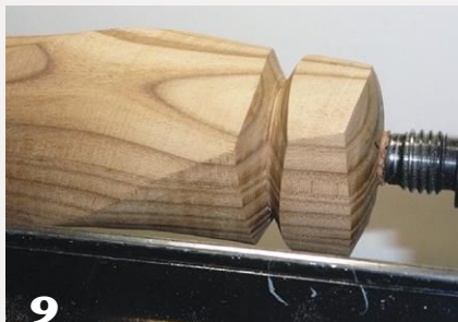
9 Turn the end of the twisted spindle to a slightly convex shape, and match that curve at the other end of the napkin ring.
