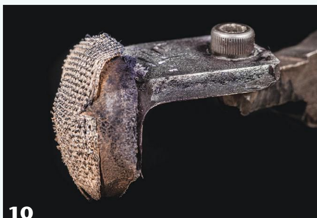
The author's shopmade sanding attachment, which mounts on his Stewart tool for reaching inside vessels. An angle of metal with hook-and-loop material glued onto it holds the abrasives.
