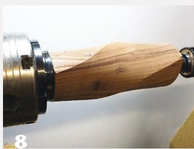
8 Remount the twisted spindle between centers on the original (true) axis. Form a tenon and mount the piece in a four-jaw chuck.
