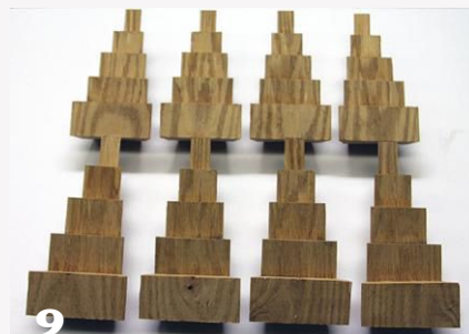
9 All stave segments glued and ready for bowl blank assembly.
