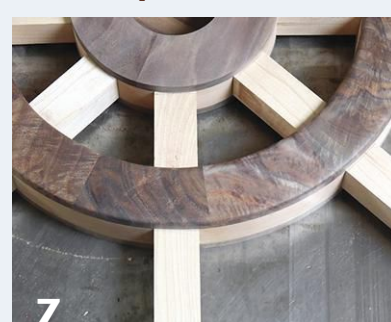
Spoke blanks are inserted through the wheel and into the hub for marking the areas that will be left square.
