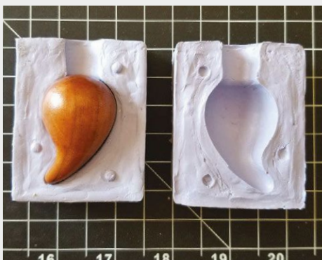
2) Two-part molds of the turned objects are created using a pourable silicone molding material.
