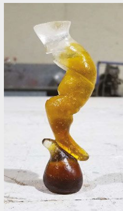
4) The wax positive is then encapsulated in a glass mold (a 50/50 mixture of molding plaster and silica) and then evacuated from the mold. The glass is then cast into the mold using kiln-casting methods, resulting in a glass positive form exactly the shape of the turned object.
