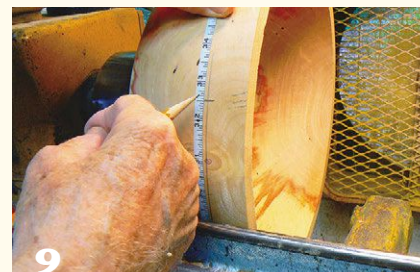
Lay out the drilling locations for the portholes, spaced evenly around the bowl.
