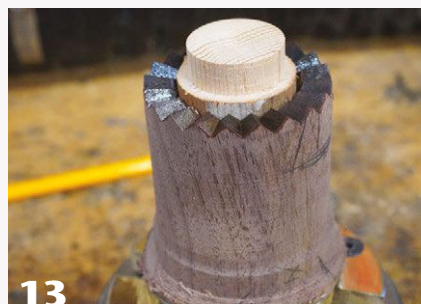
13 Glue in the spacer dowel.
