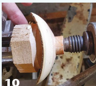
A custom jam chuck is turned from scrap wood, with a \frac{1}{4} " tenon to accept the hole of that size in the bowl. The double-sided tape and the tailstock live center also help hold the bowl in place.
