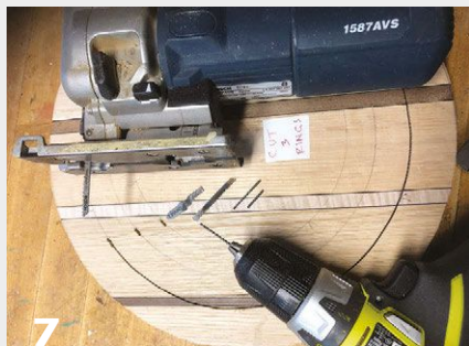
7 Mark and cut rings from each disk to create the sides of the bowl blanks using a jigsaw or scroll saw. Use a drill bit to create the initial kerf for the saw blade.
