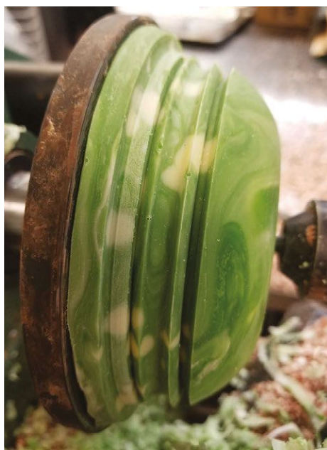
A freshly turned piece of green-tinted white chocolate. Note the lathe’s standard faceplate, at left.
