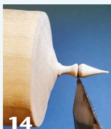
Begin turning the finial with tailstock support, until you've pared away the end to a point. For maximum support and to reduce vibration, work in small increments toward the headstock, shaping and sanding as you go.
