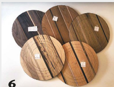
6 Cut the layers into five disks. Predominant wood species in each, clockwise from upper-left are walnut, cherry, butternut, oak, and maple. Each disk is labeled according to how many rings it will yield.
