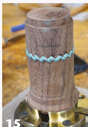
14 Colored epoxy clay fills the gap between the two halves of the ornament globe. After it has cured, the workpiece is ready for turning and hollowing.
