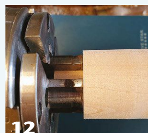
Finial stock mounted in pin jaws. Note that the tenon shoulder sits flush against the end of the jaws, and the tenon does not bottom out inside the chuck.
