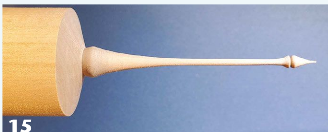
Begin turning the finial with tailstock support, until you've pared away the end to a point. For maximum support and to reduce vibration, work in small increments toward the headstock, shaping and sanding as you go.
