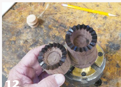
12 The exposed endgrain of the router cuts is best sealed with shellac or lacquer prior to gluing.
