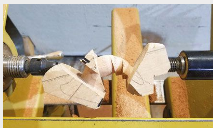
1) Forms are turned on the lathe using multi-axis techniques.
