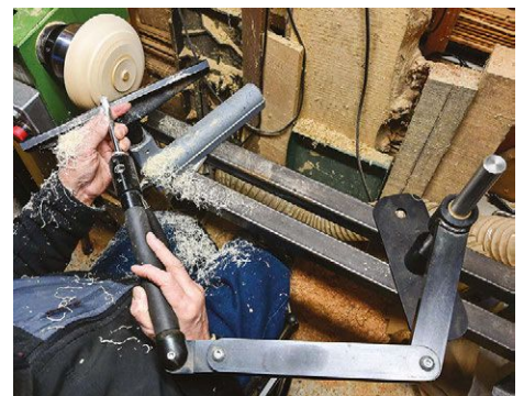
A supportive hollowing rig does most of the tool holding for you and can be adapted to non-hollowing cuts.
