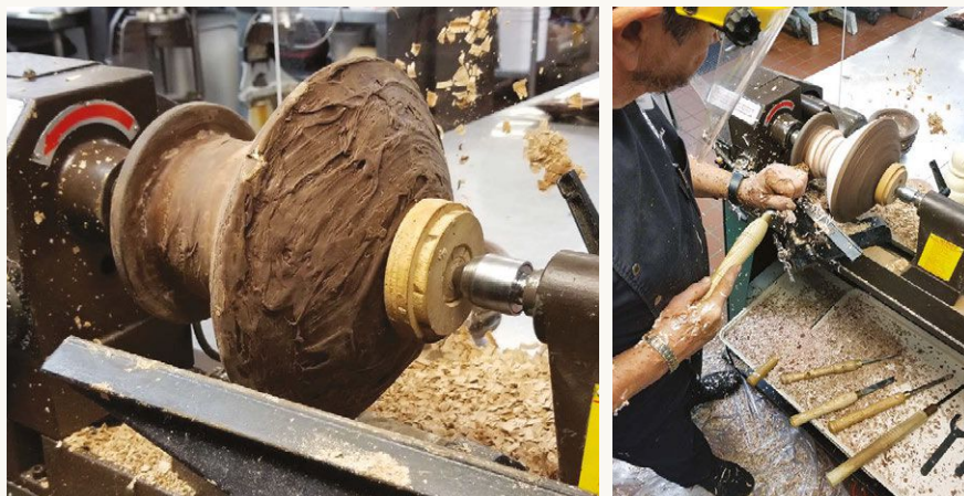
A rough blank comprises several pieces of chocolate “welded” together and to a faceplate with tempered chocolate “glue.” A tailstock-side wooden wasteblock minimizes marring. Day says the experience is like turning air, as the chocolate offers little resistance. Sharpening of tools is not necessary.
