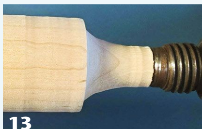
Begin turning the finial with tailstock support, until you've pared away the end to a point. For maximum support and to reduce vibration, work in small increments toward the headstock, shaping and sanding as you go.
