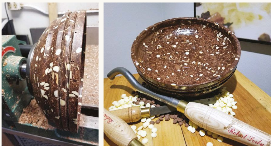
Day uses standard woodturning tools to turn chocolate forms like this bowl, made from a blend of dark, milk, and white chocolates.
