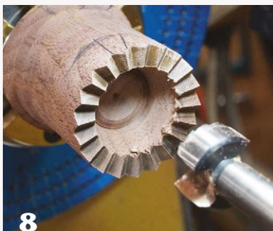
Drill a cavity to accept a spacer dowel.
