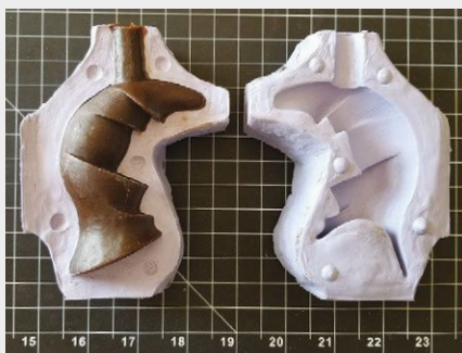
3) A wax positive is cast in the silicone mold.
