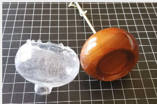
A positive form is turned on the lathe and then sealed. Using a combination of dipping and airbrushing techniques, silicone is applied to the exterior. After the silicone has cured, it is removed from the wood manikin and retains its new shape.
