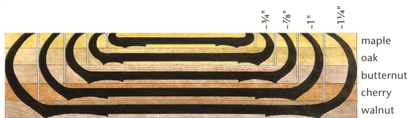
Figure 1. The rim thickness for each vessel decreases with the size of the form, an important detail when cutting the rings from their respective blanks.
