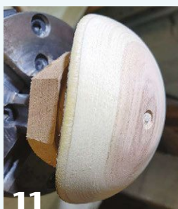
Turn away the tenon, then remove the tailstock so you'll have access to complete the bottom of the bowl.
