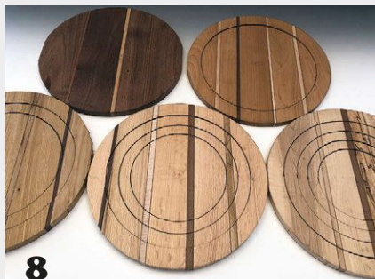
7 Mark and cut rings from each disk to create the sides of the bowl blanks using a jigsaw or scroll saw. Use a drill bit to create the initial kerf for the saw blade.
