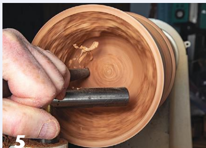
5 The top part of the urn is hollowed in the same progressive manner as the base. The neck hollowing is deepened beyond the planned opening point.
