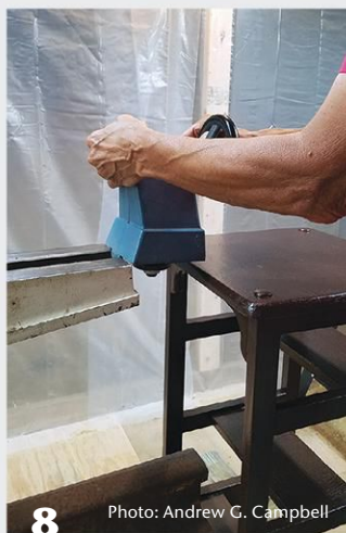
(8) A table at the correct height at the end of your lathe shortens the carry distance of a heavy tailstock, lessening the strain on your shoulders and arms.
