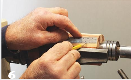
6 Measure napkin ring width and part off. Repeat the process for each additional ring.
