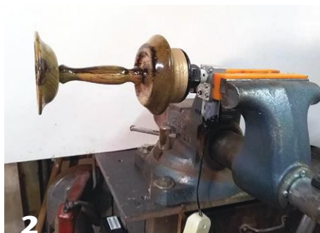
The low-rpm motor is held in a vise during use. The piece rotates slowly so the finish can dry without the issues of gravity.
