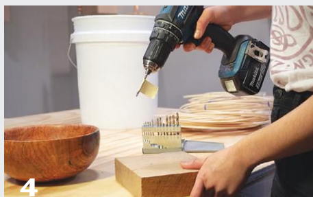
4 Use a hand-held drill to bore holes in the rim, angled slightly to facilitate a natural flow from bowl to basket.
