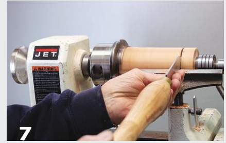
6 Measure napkin ring width and part off. Repeat the process for each additional ring.
