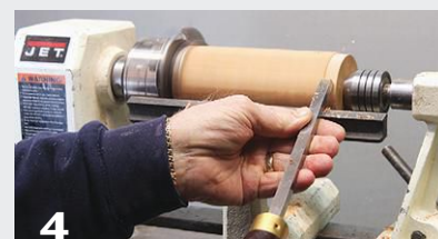
The blank is first mounted in a chuck and supported by a cone center in the tailstock. The author turns a tenon using a bedan.
