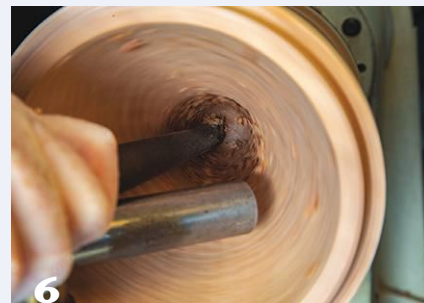
5 The top part of the urn is hollowed in the same progressive manner as the base. The neck hollowing is deepened beyond the planned opening point.
