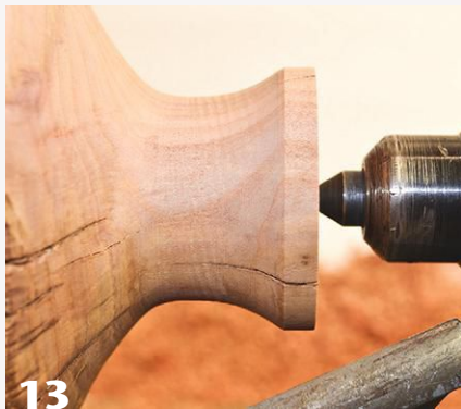
Refine the neck shape, carefully blending cove cuts from the top and bottom. Cut a slight relief in the spout before boring the opening.
