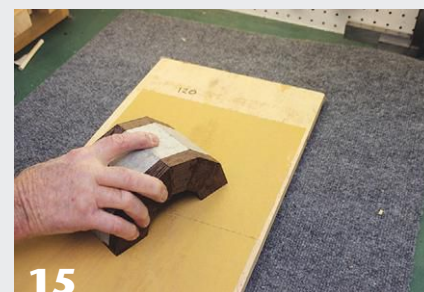
14 To correct for the gap, glue up the two halves but keep them apart using dowels opposite one another. After the glue dries, sand the remaining joints on a flat board, then glue the two halves together.
