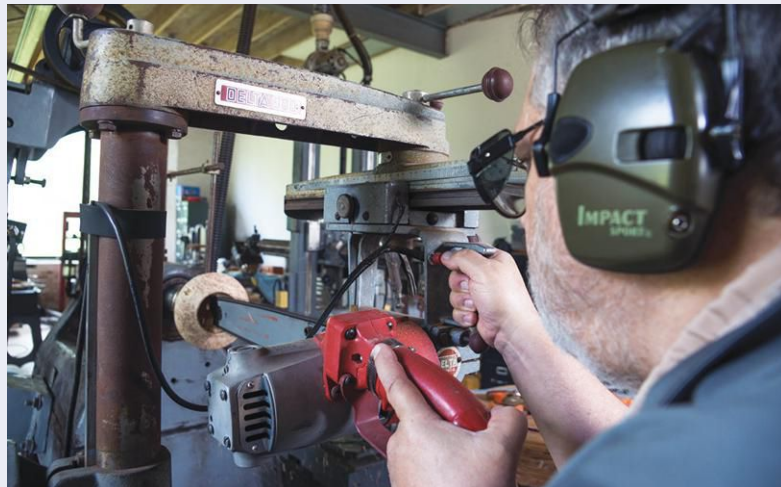
Mark's captive chainsaw system. The work is rotated in small increments and is stationary when each plunge cut is taken.
