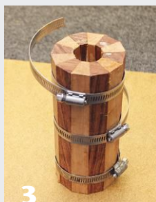
Apply glue to the staves; wide masking tape keeps them in position. Hose clamps provide gluing pressure.
