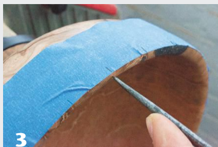
3 Mark out evenly spaced hole locations.
