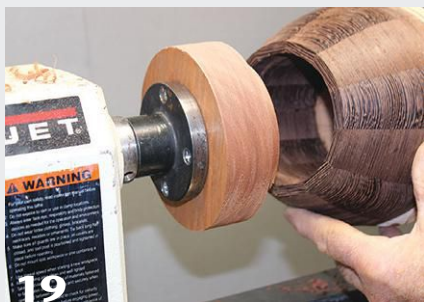
19 Attach the bowl base material to a faceplate, and form a rabbet that will fit snugly into the bottom of the bowl. Glue and clamp the base to the bowl.
