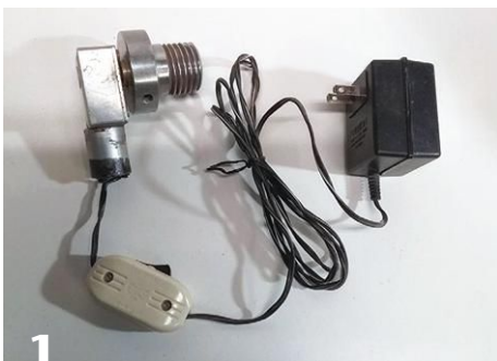
A small DC motor (upper left) is powered by a DC accessory cord, wired through a rocker switch. A small faceplate is mounted on the motor shaft by way of an adapter.
