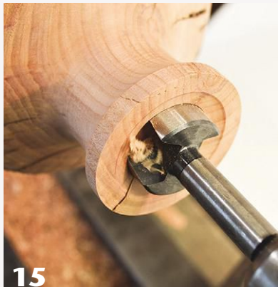
The author uses a Forstner bit to bore the opening. Retract the bit often to clear the shavings as you go.
