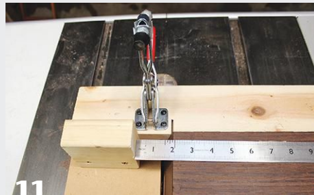
11 Set the position of the stop block indicating stave width.
