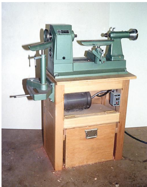
A working prototype of the Lewin Bowl Lathe, a short-bed, variable-speed innovation later manufactured by Woodfast under the name Woodfast BL300.
