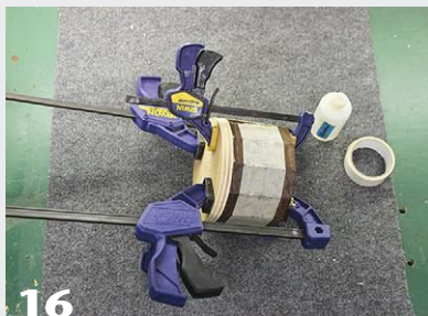
16 Smooth one end of the glued-up blank, and affix an auxiliary wood faceplate using double-sided turner's tape or glue.
