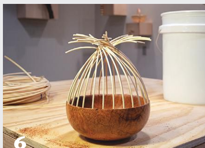
6 Insert spokes into the holes, then submerge them in water. The spokes will swell in the holes and should remain there securely.
