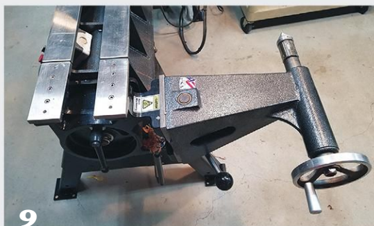
(8) A table at the correct height at the end of your lathe shortens the carry distance of a heavy tailstock, lessening the strain on your shoulders and arms.
