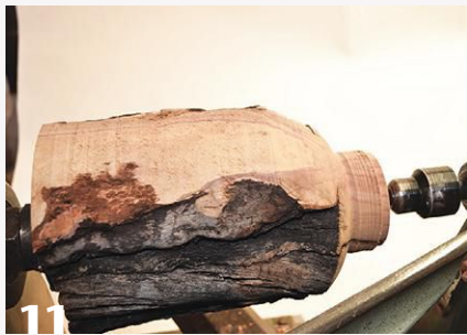
Cut away edges to rough the basic shape. Determine the size of the base in relation to the top. Note that the natural wood features are retained.
