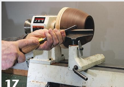
17 With the workpiece mounted on a metal faceplate, turn the blank round and begin to shape the bowl, its foot at the tailstock end. True the bottom and turn inside the lower part of the bowl near the base.
