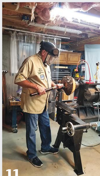
(10) With a typical lathe setup, bowl hollowing requires the right arm to reach out across the bed ways to begin the cut, a potentially painful endeavor if your shoulder is painful or weakened.
