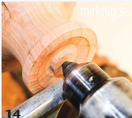
Refine the neck shape, carefully blending cove cuts from the top and bottom. Cut a slight relief in the spout before boring the opening.
