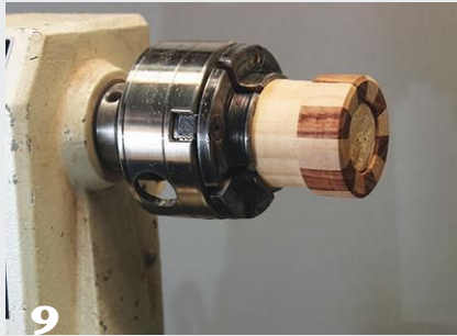
9 A softwood dowel turned to the right size serves as a jam chuck for remounting the rings for final trimming and sanding.
