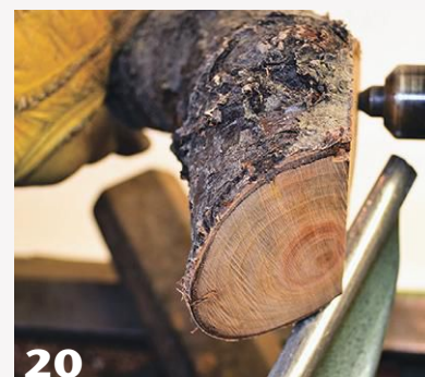
Flats are cut at the top and bottom ends to provide surfaces for a drive and live center. The bottom of the pot should be mounted at the tailstock end to provide better access for forming a tenon.
