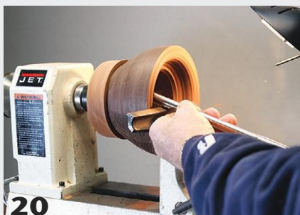
20 Finish-turn the bowl, outside and in. When the turning and sanding are completed, part the bowl at its base, taking care not to cut into the faceplate screws.
