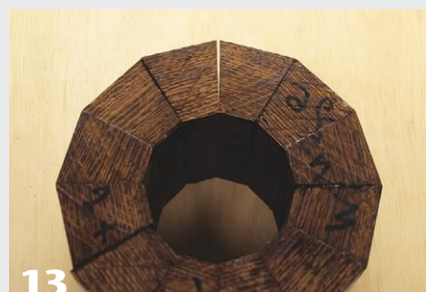
13 Dry-fitting the bowl staves reveals a gap!
