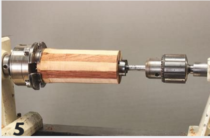
5 With the workpiece remounted in the chuck using the tenon, a 1 \frac{3}{8} " Forstner bit is used to drill a straight-walled center hole.
