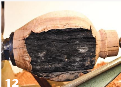
Cut away edges to rough the basic shape. Determine the size of the base in relation to the top. Note that the natural wood features are retained.
