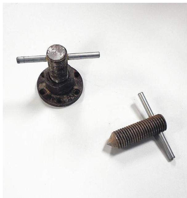
The Lewin Center Finder, used for accurately marking the center of faceplate-mounted turnings, an innovation used in various iterations today.
