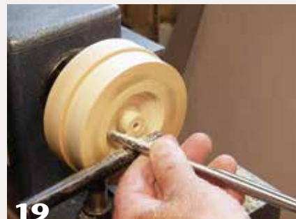
19 Then connect the dots with a gouge, turning a flat, angled surface.
