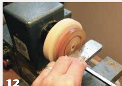
12 Reverse-mount the partially turned ring, using the faceplate dowel to center and hot-melt glue to hold it in place. Cut the second angled face, just as you did the first.
