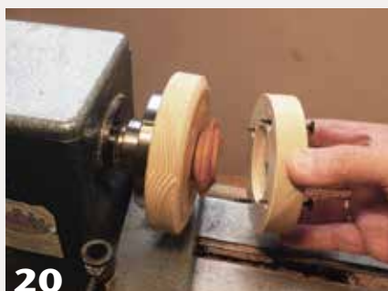
20 Support collar retains partly turned small rings, where hot-melt glue wouldn't suffice.
