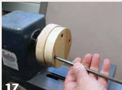
17 Fit a support collar blank to the faceplate, centering it on the dowel and screwing it in place.
