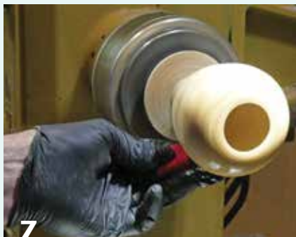
7 With the lathe spinning fairly quickly, apply multiple coats of the “wipe-on” lacquer, allowing them to dry to the touch between applications.
