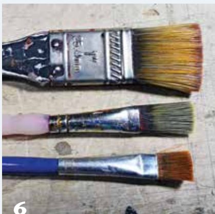
Common inexpensive golden and white taklon synthetic fiber brushes, in various widths, are great for gilding. Dux Paint Co. gold leaf oil-based size will gum up around the can opening, and partially full cans of Quick Dry type will usually skin over during storage. Remove skin and stir the contents of every can before applying size.
