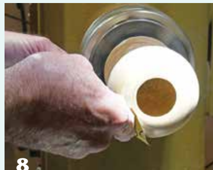
8 With the lathe turning slowly, sand the lacquer with a light touch, using a fine-grit abrasive. If the finish is sufficiently dry, this will produce a fine white powder.
