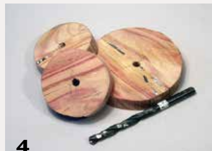
Bandsaw the blanks to the specified diameters, then bore \frac{1}{4} " holes at the center.
