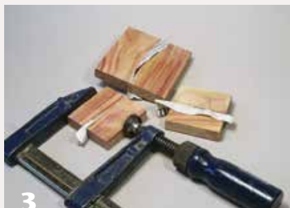
Glue and clamp blanks with a layer of newspaper in the joint, so you can split them apart later with no loss of wood.
