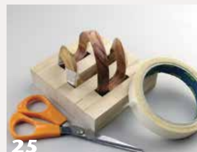
Masking tape holds the ribbon parts together while the glue dries.
