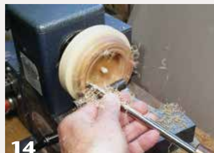
12 Reverse-mount the partially turned ring, using the faceplate dowel to center and hot-melt glue to hold it in place. Cut the second angled face, just as you did the first.
