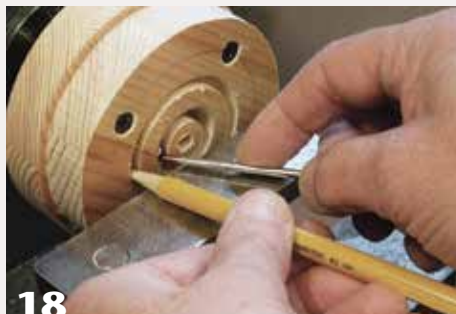
18 Mark and turn to the depths shown in Figure 3 . Then connect the dots with a gouge, turning a flat, angled surface.
