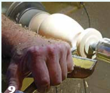
9 With the vessel reverse-mounted on a jam chuck and the tailstock brought up for support, carefully complete the turning of the foot. Sand and apply lacquer to the foot.
