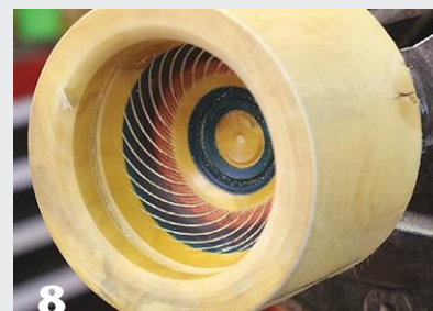
The box lid, ready for female threads.
