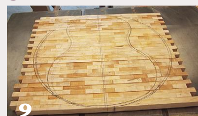
A segmented board is turned to thickness, then cut to shape and used as the guitar back.
