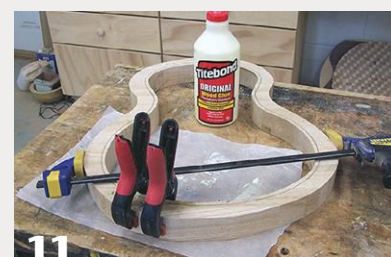
To cut out the inside of the form at the bandsaw, a kerf through the side is necessary to provide blade access. After cutting the inside shape, the kerf was closed back up with glue.
