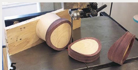
5 Soundhole accents are inserted, then turned flush before construction of the vessel continues.
