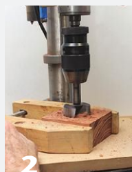
2 In the thickest piece, drill a hole for the glass cup. Trim the pieces round. The veneer can be trimmed using scissors.
