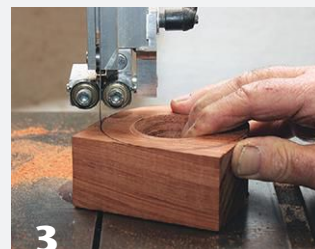
2 In the thickest piece, drill a hole for the glass cup. Trim the pieces round. The veneer can be trimmed using scissors.
