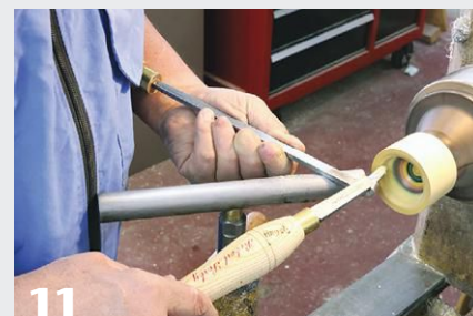
The female thread chaser is used with the armrest tool to form interior threads. An initial groove in the chamfer acts as a starting point for cutting the threads. Note that the chaser tool progresses to parallel with the bed ways as the threads develop.
