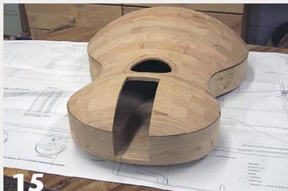
15 The assembled guitar body, ready to accept the neck.
