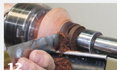
12 Reverse the piece in the chuck one last time, and part the tenon from the base. Complete and sand the bottom.
