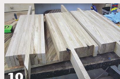
The author glues up several boards from which he cuts the guitar sides.
