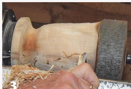
3 A detail gouge cleans up the wood surface. A skew could also be used, but the detail gouge may be easier for navigating curves.
