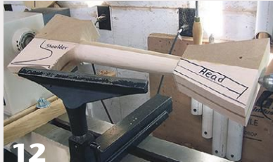
12 The neck is a split turning, generating two necks. The headstock and shoulder are drawn and rough-shaped on the bandsaw, while the neck portion is turned to dimension before the two pieces are cut apart.
