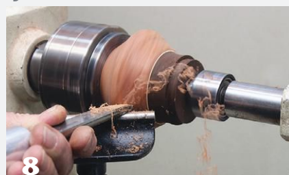
8 Reverse the blank in the chuck, holding it once more in expansion mode, and shape the lower section of the candleholder. The author uses a gouge, followed by a negative-rake scraper to refine the surface.
