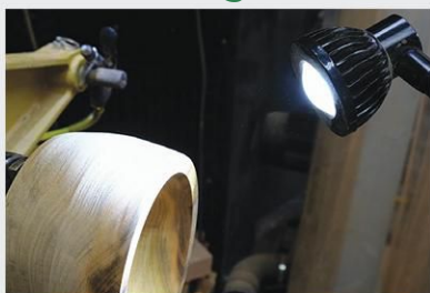
A task light aimed at a low, raking angle illuminates imperfections on the wood surface.
