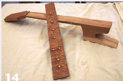
14 The turned and shaped neck, ready to accept the fretboard.
