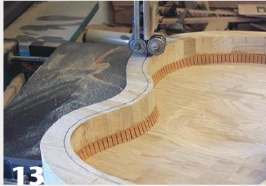
13 After the sides are glued to the back, reinforced with kerfing, the author trims the sides to final thickness at the bandsaw.
