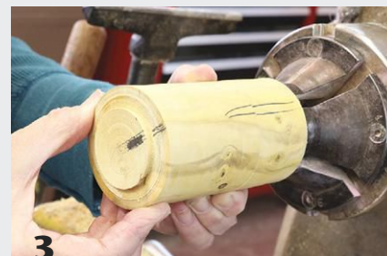
3 Hold the base up to the lid with the grain aligned and make registration lines to help with realignment later.
