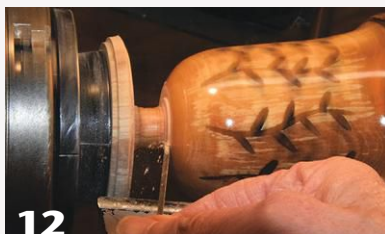
A thin parting tool is used to slightly undercut the bowl's base as the bowl is parted off the lathe.
