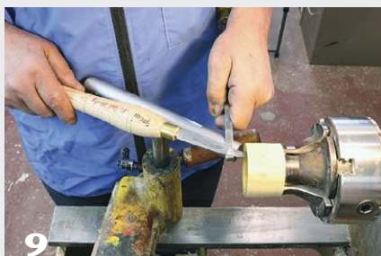
The female thread chaser is used with the armrest tool to form interior threads. An initial groove in the chamfer acts as a starting point for cutting the threads. Note that the chaser tool progresses to parallel with the bed ways as the threads develop.
