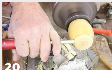
The box base is reverse-mounted on a “threaded chuck” made from waste wood so the base can be completed.
