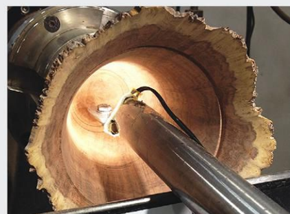
Some task lights are extremely small and can be placed very strategically. This Microlight, made and sold by Cindy Drozda, is kept in place on the toolrest (left) and on a cutting tool (right) by magnets.
