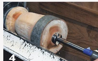
4 Drill to the desired inside depth with a Forstner bit held in a drill chuck in the tailstock. This hole will act as a starting point for endgrain hollowing.
