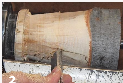
2 A bowl gouge handles the rough-shaping of the bowl's outside profile. The author chooses to leave a band of bark at the rim.
