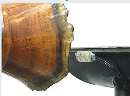
Some task lights are extremely small and can be placed very strategically. This Microlight, made and sold by Cindy Drozda, is kept in place on the toolrest (left) and on a cutting tool (right) by magnets.
