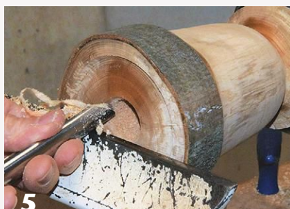
5 The author uses a bowl gouge to hollow this endgrain bowl. The tool cuts from center hole toward the outer wall.
