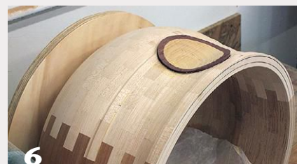
5 Soundhole accents are inserted, then turned flush before construction of the vessel continues.
