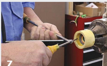
The armrest tool (in the author's left hand) provides cutter access (right hand) inside the lid without having to position the toolrest perpendicular to the lid opening. Form a chamfer at the outer edge, then a recess where the threads will stop.
