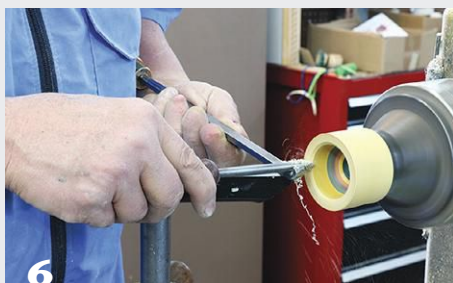
The armrest tool (in the author's left hand) provides cutter access (right hand) inside the lid without having to position the toolrest perpendicular to the lid opening. Form a chamfer at the outer edge, then a recess where the threads will stop.
