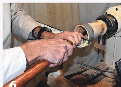
6 Pressing the gouge's long handle against your right forearm helps reduce vibration and counteracts the "grabby" tendency that occurs when a tool is extended well beyond the toolrest.
