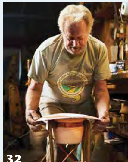
The hat is set in a bending jig, whose curved jaws squeeze the band into an oval shape. Rubber bands pull the brim into the desired curve.
