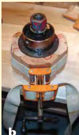
(b) The bevels align the wood jaws into an octagon. Pre-drill and use long screws to attach the wood to the jaws.
