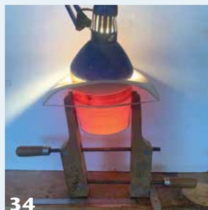
33 With the hat in a screw clamp, a stop block defines the final interior width, and heat from a lamp "bakes" it dry in this position.
