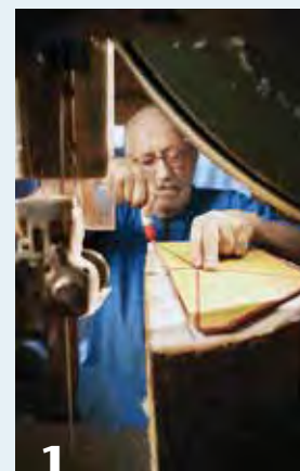
1 Mark the block's endgrain using a sizing/positioning template.
