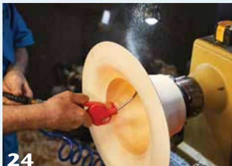
Compressed air blows water out of the wood, so the wood can be sanded.
