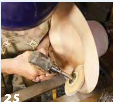
Compressed air blows water out of the wood, so the wood can be sanded.
