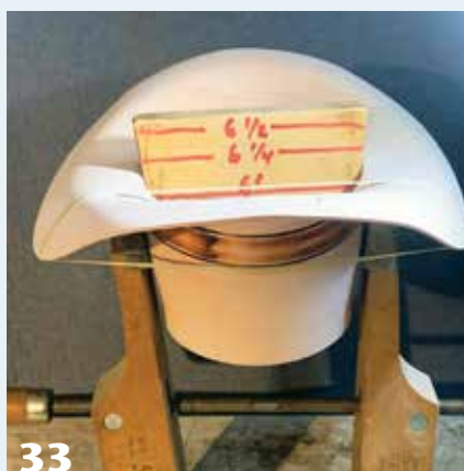
33 With the hat in a screw clamp, a stop block defines the final interior width, and heat from a lamp "bakes" it dry in this position.
