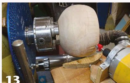
13 A custom curved fence mirroring the bowl's shape ensures a consistent depth of cut.
