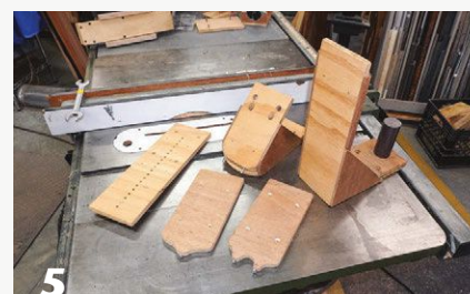
5 The author's router carriages, used for different purposes.
