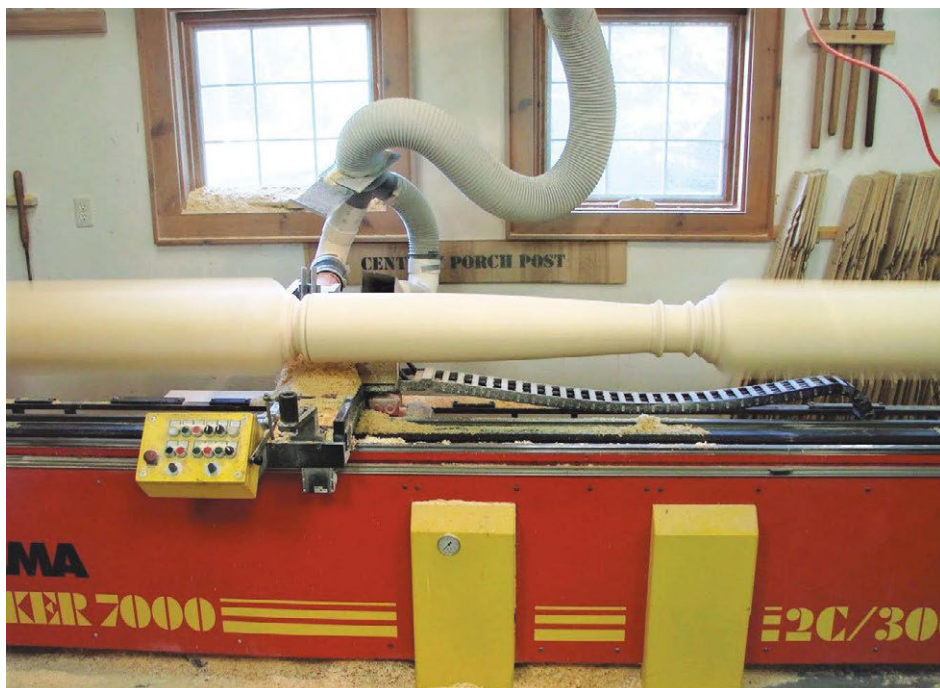
CPP's bread-and-butter machine: an automated, large-capacity Wema lathe.
