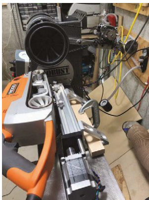
Automated, shopmade two-axis CNC for the wood lathe, using a belt sander to form a scalloped rim.
