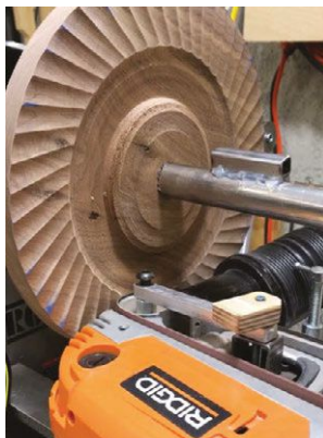
Automated, shopmade two-axis CNC for the wood lathe, using a belt sander to form a scalloped rim.
