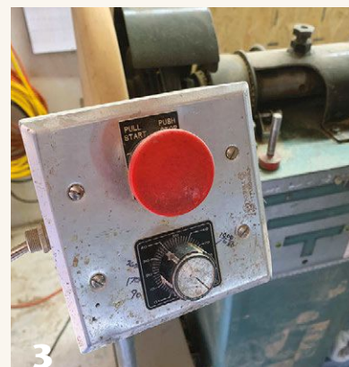
3 Marks applied to a standard speed control give an idea of rpm and, by calculation, an idea of surface speed. This controller is on a pedestal stand, so the author can keep it close at hand when working on longer pieces.
