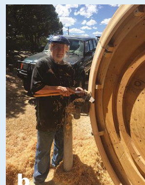
b The large diameter of this molding meant the author could turn at sufficient surface speeds without getting the lathe above 100 rpm.
