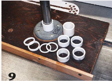
9 Various lengths of PVC pipe fit over the table post and take the guesswork out of setting the height.
