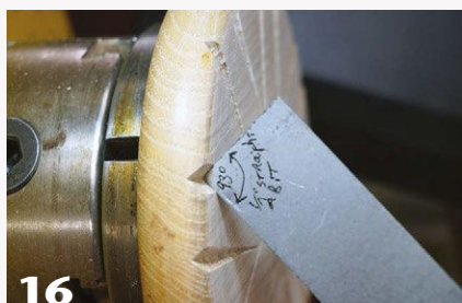
16 When sawing contrasting inserts, don't trust that the routed V-cut is a true 90 degrees. Gauge the actual routed angle by filing a piece of steel until it fits perfectly, then use the steel as a guide for setting your table saw tilt.
