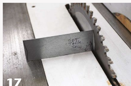
16 When sawing contrasting inserts, don't trust that the routed V-cut is a true 90 degrees. Gauge the actual routed angle by filing a piece of steel until it fits perfectly, then use the steel as a guide for setting your table saw tilt.
