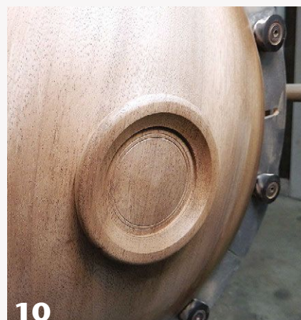
Reverse-mount the bowl to turn away the tenon and form the foot.
