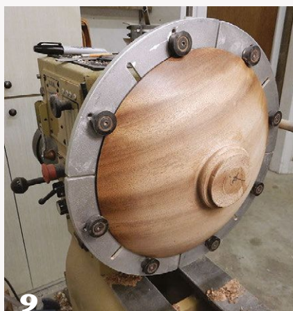
Reverse-mount the bowl to turn away the tenon and form the foot.
