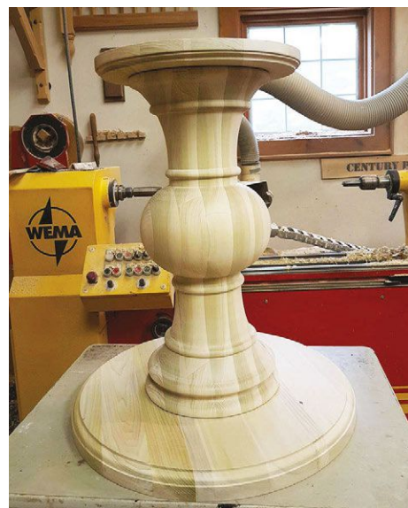
Large-diameter column caps and bases, as well as pedestals, are turned by hand.
