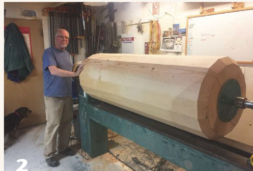
2 A typical live center in the tailstock wouldn't suffice for this large turning. Some custom metal work connected a large faceplate to a bearing on the outside of the #3 Morse taper tailstock quill.
