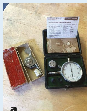
a Determining surface speed, with either a gauge or formula, provides useful information in setting lathe speed.
