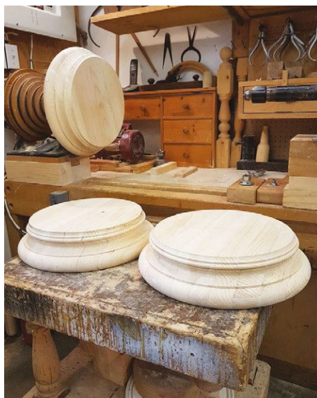
Large-diameter column caps and bases, as well as pedestals, are turned by hand.
