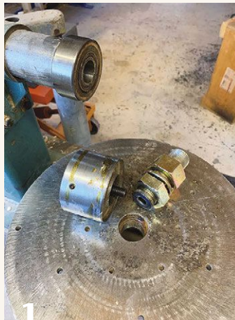
2 A typical live center in the tailstock wouldn't suffice for this large turning. Some custom metal work connected a large faceplate to a bearing on the outside of the #3 Morse taper tailstock quill.
