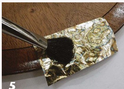
A dry brush is used to press the metal leaf into the tacky size. Additional pieces of leaf slightly overlap subsequent pieces.
