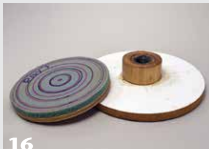
16 Shopmade jam chucks. One (left) is mounted by means of a faceplate and the other with a nut epoxied in a block at the back of the disk. Both are covered with closed cell foam.
