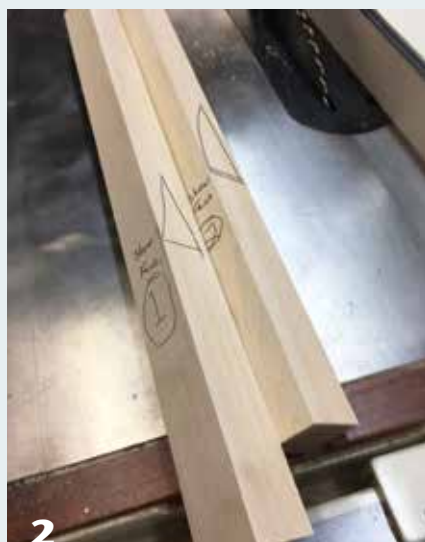
2 Whole, uncut leg blanks are labeled with leg number and “show face,” as well as a reference triangle on one side and the leg number on the back face (not visible in photo).
