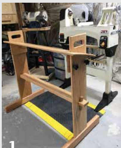
R.C.'s standing rest was inspired by a photo of a seat attached to an antique lathe and modeled after a weaver's bench. The rest supports his buttocks and alters his weight distribution while standing for spindle work.
