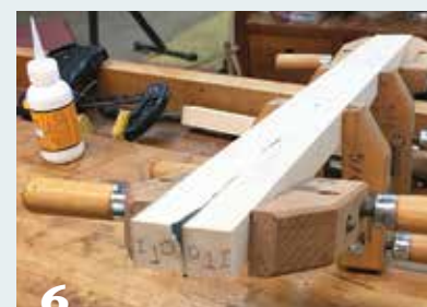
6 The author makes a newspaper glue joint to temporarily join the show face parts, now with the outside edges facing in.
