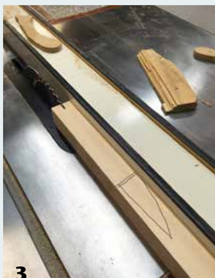
3 Leg blank being halved into show face and back face pieces. The triangle will aid in realignment later, when the parts are reassembled.
