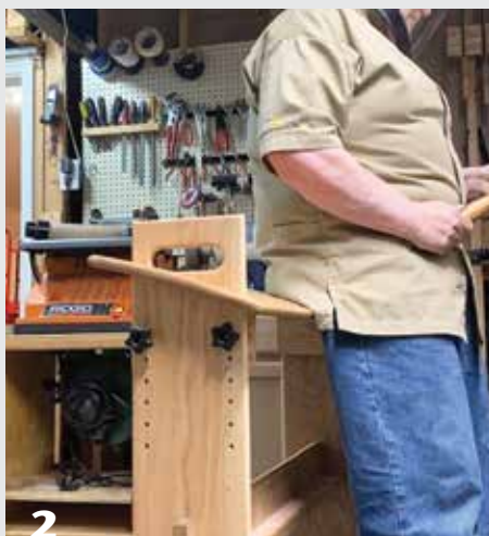
R.C.'s standing rest was inspired by a photo of a seat attached to an antique lathe and modeled after a weaver's bench. The rest supports his buttocks and alters his weight distribution while standing for spindle work.
