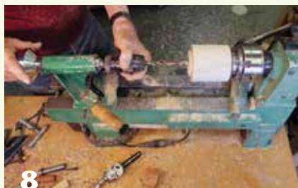
8 Mount the base in a scroll chuck, drill a \frac{3}{8} "-diameter, 2"-deep hole, and hollow the interior.
