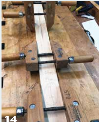
14 Glue show face parts of legs back together in their original configuration. Note the turned inside-out detail now completed and facing inward.
