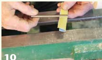
10 Use a sanding aid to safely finish the interior. The author uses a shopmade flap sander mounted in a drill for the task.
