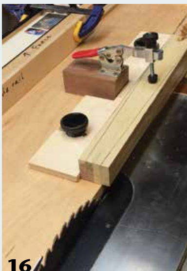
16 The author uses a tapering jig on the table saw for final shaping of the stool leg.
