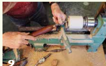
8 Mount the base in a scroll chuck, drill a \frac{3}{8} "-diameter, 2"-deep hole, and hollow the interior.
