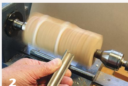
2 Carefully turn the blank to a cylinder, moving and retightening the cable ties as you go. Form a tenon at the tailstock end.
