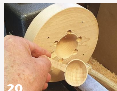
20 Remove the MDF plate and pick out the hot-melt glue to release the finished spoon.
