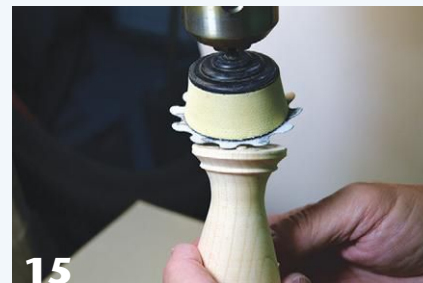
15 Carve or sand away the remaining nub, and sand the base with the same series of abrasives used on the outside of the form.
