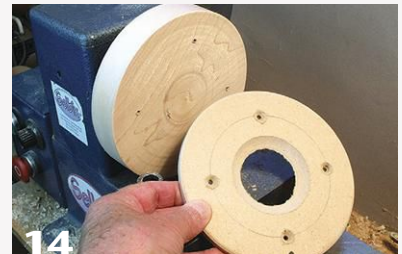
14 The author's shopmade chuck comprises a softwood disk and an MDF cover plate that holds the spoon in place. After turning a “window” in the MDF, make reference marks and temporarily remove the MDF cover plate.
