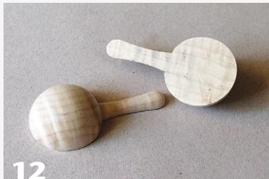
12 Split the turning at the newspaper joint line. Sand the two halves clean so they are ready to be hollowed.
