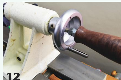
12 Adjusting the nut and washer to allow a small amount of travel facilitates centering the bit in the blank. After centering, tighten the nut and washer to remove the travel and lock the drawbar.
