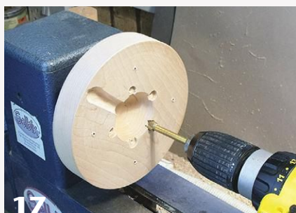
17 Drill ⅜" holes around the periphery of the hemispherical hollow, such that the holes break into the hollowed area.
