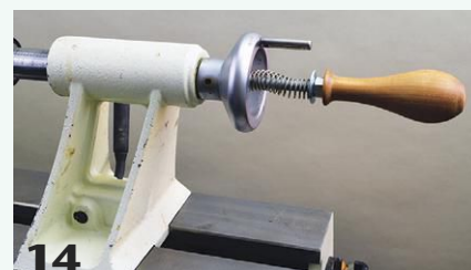
13 A strong spring over the threaded rod spring-loads the drawbar, applying a counter force to keep the arbor and quill snug.
