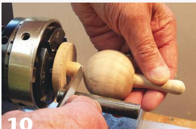
10 Part the spoon off, first at the tailstock end, then at the headstock.
