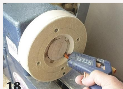
18 With the spoon in place and the MDF cover plate screwed down, add hot-melt glue into the drilled holes to secure the spoon blank.
