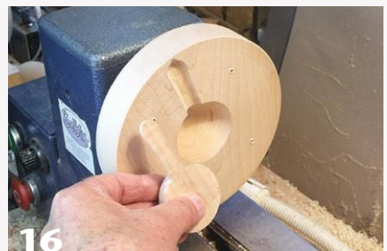
16 Outline the spoon handle on the softwood disk and carve out a recess to accept it.
