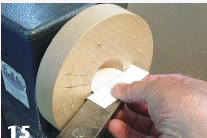
15 and Figure 3. Turn a hemispherical hollow in the softwood chuck, and use a card template made to the specifications shown for sizing.
