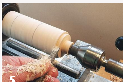
5 Turn the first section to \frac{3}{4} " diameter, then the handle area to \frac{1}{2} " diameter.
