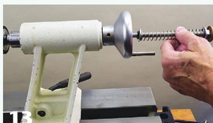
13 A strong spring over the threaded rod spring-loads the drawbar, applying a counter force to keep the arbor and quill snug.
