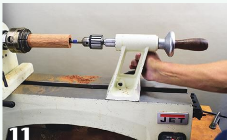
11 Properly tensioned with a washer and nut, a drawbar maintains firm contact between the arbor and quill, even when extracting the bit.
