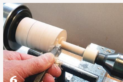
5 Turn the first section to \frac{3}{4} " diameter, then the handle area to \frac{1}{2} " diameter.
