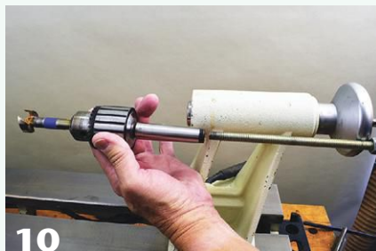
10 Many arbors will accept a drawbar made from threaded rod.
