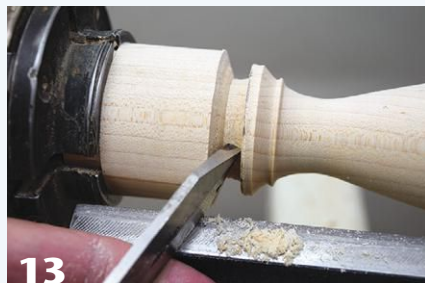
13 Slightly undercut the base with a parting tool, then complete the cut with a fine-toothed saw with the lathe off.
