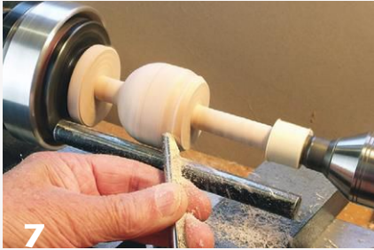
7 Turn the outside of the “bowl” section of the spoon.
