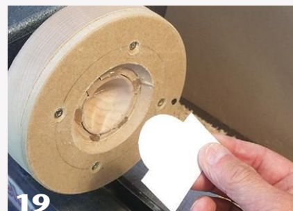
Figure 4 and 19. Hollow the bowl section of the spoon, using a card template made to the specifications shown for sizing.
