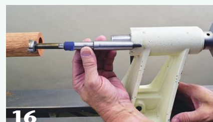
16 Arbors for using Forstner bits directly in the tailstock quill are also available.
