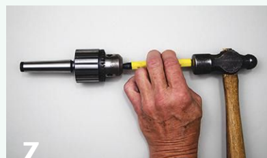
A drill chuck arbor separates from the head with a punch and sharp hammer tap for easy replacement.
