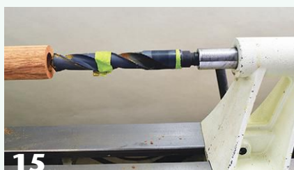
15 Twist bits can be purchased that are milled with a Morse taper to fit directly into the quill.
