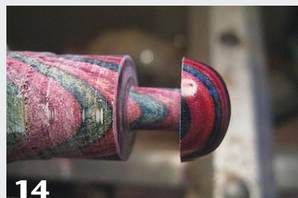
14 After the magnets are installed, the exposed hole on top of the box lid can be concealed with a decorative button of a contrasting wood species.
