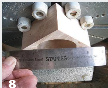
The author uses a sharp hand plane blade as a scraper, then checks for flatness with a straightedge.
