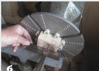
6 Use a depth gauge to ensure about ¼" thickness at the bottom.
