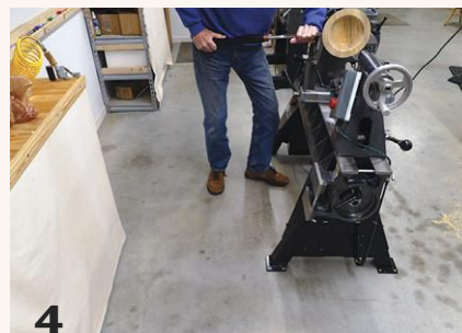
3 These all-too-common stances at the lathe will require you to either interrupt the cut to move your feet or risk falling over. Either way, a catch is likely.
