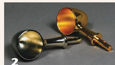
2 A smooth metal stem acts as a tenon that is glued into a hole drilled in a turned handle.
