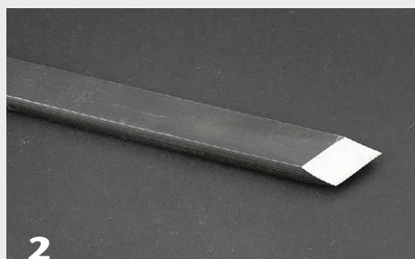
2 Rectangular skew with flat top edge and rounded bottom edge.
