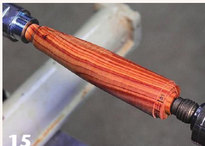
15 Rough-turned blank reversed onto a bottle-stopper mandrel for turning between centers.
