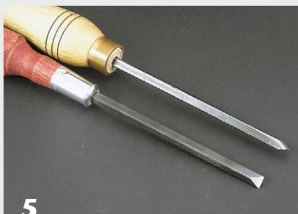
Skews come in different shank sizes and shapes. The square-shanked skews at right (aka, beading and parting tools) were fashioned from old screwdrivers.
