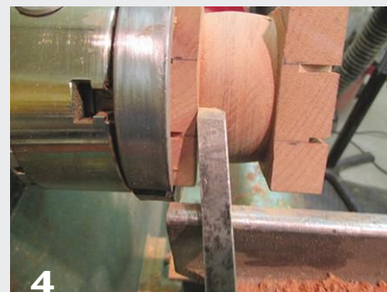
4 Turn away only the center material in the shape of a sphere.
