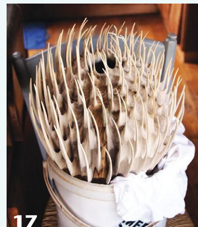
17 A small hose connected to a pressure cooker provided steam, which allowed the filaments to be bent without breaking.
