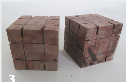
3 Marked and pre-cut cubes. Making small kerfs inside each corner cube helps to preserve the cube's clean surfaces during turning.
