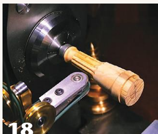
18 A bottle-stopper mandrel used on a rose engine lathe without a tailstock, to turn handle for a threaded-stem kit.
