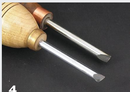
Skews come in different shank sizes and shapes. The square-shanked skews at right (aka, beading and parting tools) were fashioned from old screwdrivers.
