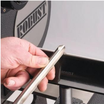
Straight Rests w/Hardened Rod
