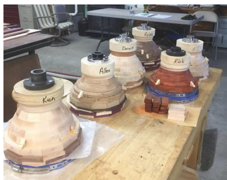
Segmented bowls in process of construction.
