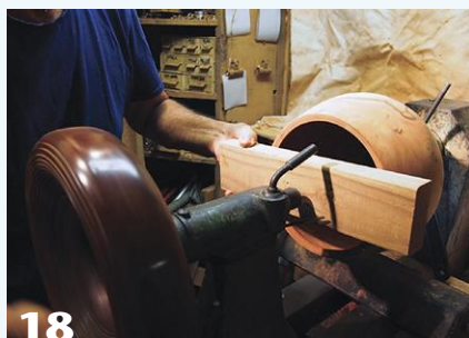
18 When remounting the bowl after drying, use tailstock pressure to ensure the tenon shoulders seat properly on the chuck jaws.
