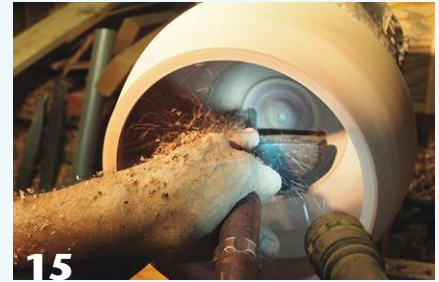
14 A bowl gouge with a very short bevel ground nearly straight across is useful for making supported bottom cuts. A gouge with swept-back wings and a longer bevel would not maintain bevel contact during these cuts.
