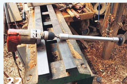
22 Many Hawaiian bowl forms are taller than they are wide, so a sanding pad on a long extension comes in handy.
