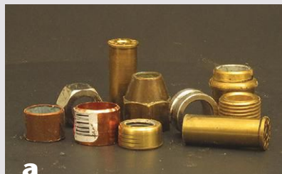
a Options for making ferrules include copper pipe, brass shell casings, and brass plumbing fittings.
