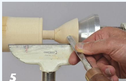
4 With the interior hollowed and the workpiece supported by a cone center on the tailstock, shape the outside of the funnel, including the stem.
