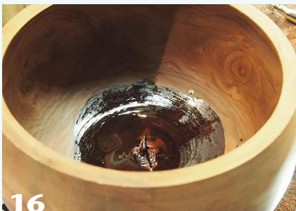
16 Since the bowl is turned endgrain, the log's unstable pith remains in the bottom. The author soaks the softer, crumbly fibers with thinned lacquer to stiffen the area. He then glues in wedges to fill the gaps.
