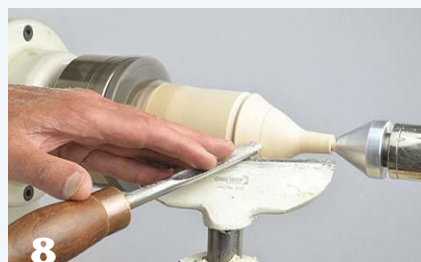
7 Shape the remaining waste material still mounted in the chuck into a jam chuck that will accept the funnel's interior when reverse-mounted. The cone center inserted into the funnel's hole automatically realigns the work. Make final passes to turn away any off-center wobble.
