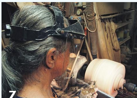
7 A spindle-roughing gouge is used to continue shaping the bowl's outside profile.
