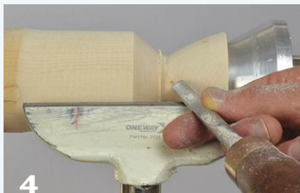
4 With the interior hollowed and the workpiece supported by a cone center on the tailstock, shape the outside of the funnel, including the stem.
