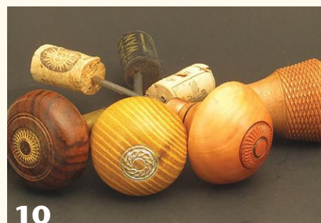
10 A variety of textured handles, framed with V-grooves or beads and embellished with metallic wax.
