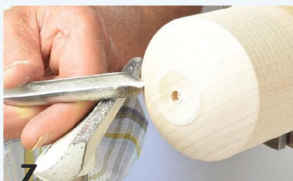
7 Shape the remaining waste material still mounted in the chuck into a jam chuck that will accept the funnel's interior when reverse-mounted. The cone center inserted into the funnel's hole automatically realigns the work. Make final passes to turn away any off-center wobble.
