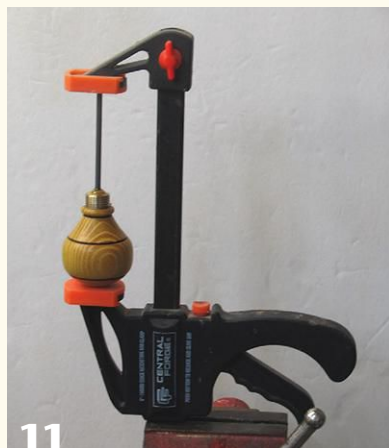
11 Clamp the shaft in the handle while the glue is curing.
