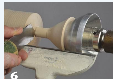
6 Part off the funnel using a narrow parting tool.
