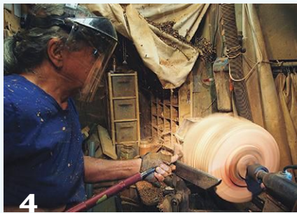
4 With the wood's natural features aligned as he wants them, the author completes the rough-turning, first with a large bowl gouge, then with a spindle-roughing gouge.
