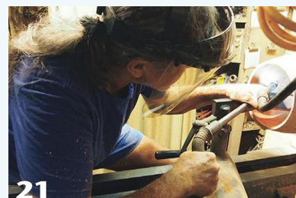
21 The author uses an armbrace tool with a teardrop-shaped scraper to refine the inside walls.
