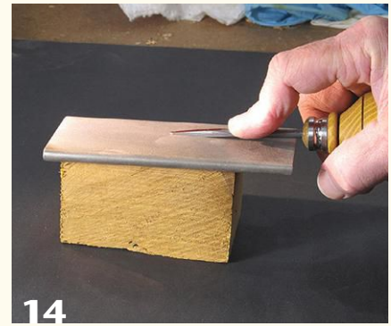
14 Use a hone for fine-tuning the tip after rough-shaping.
