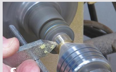
c You can use a parting tool as a scraper to remove threads or flats from brass plumbing fixtures.
