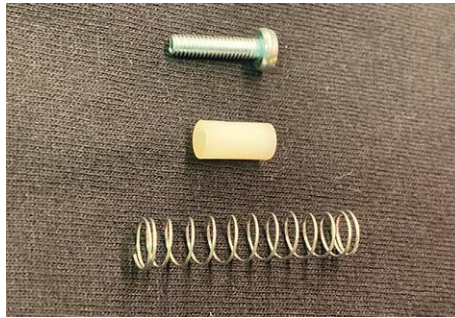
A hardware-store replacement screw, plastic spacer, and spring save you the cost of replacing the entire assembly.
