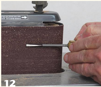
12 Shape the awl tip with a belt sander, creating four flat facets with bevels of equal length.
