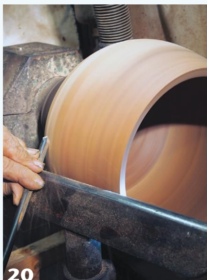
20 A shear-scraping cut refines the bowl's elegant lines.
