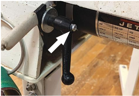
The motor plate lock handle assembly on the author's JET mini-lathe. The affixing screw can sometimes vibrate loose.
