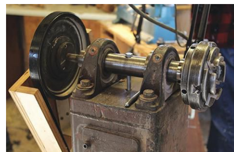
The headstock of Jerry's shopmade bowl lathe—functional, sturdy, stripped down, perfect. Filled with sand and bolted to the floor, the welded-steel unit refuses to vibrate.
