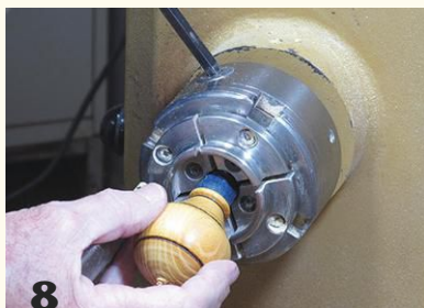
8 Reverse-chuck the handle for finishing its bottom. The bead at the top of the ferrule acts as a bearing surface against the front face of the chuck jaws.
