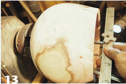
13 A simple gauge set to the desired interior depth, applied with the lathe off, indicates how much material still needs to be removed.
