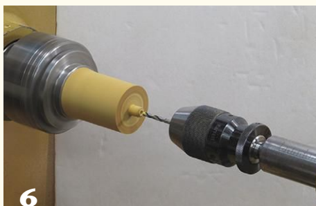
6 Drill the hole for the metal shaft.
