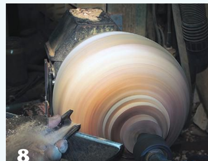
7 A spindle-roughing gouge is used to continue shaping the bowl's outside profile.
