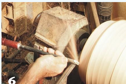
6 At the headstock end, the author uses a bowl gouge to define the rim diameter and true part of the endgrain face.
