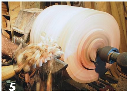
4 With the wood's natural features aligned as he wants them, the author completes the rough-turning, first with a large bowl gouge, then with a spindle-roughing gouge.
