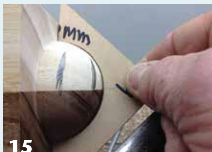
15 After using the template to arrive at the precise dimension, the pieces are easily separated with denatured alcohol.
