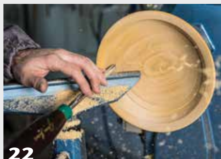
22 The author uses a 3/8" bowl gouge to refine the rim and take light, cleaning passes inside the bowl.
