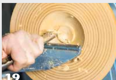
19 Pull the tool handle towards you to guide the cutting edge deeper into the wood.
