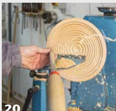
20 Repeat the hollowing cuts, working from center to rim. The steps that are formed will make it easier to start subsequent cuts as you hollow the bowl.
