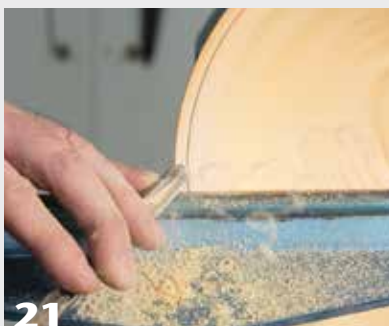
21 The author uses a 3/8" bowl gouge to refine the rim and take light, cleaning passes inside the bowl.
