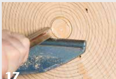
17 Mark circles on the face of the blank about 1/4" apart using a pencil. With the gouge flute rolled away from you, push to form a small V-groove. This helps prevent the tool from skating to the left.
