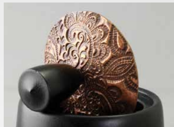
Firing precious metal clay, or PMC, in a kiln burns away the binders and leaves a solid metal object—in this case, a textured copper lid for a turned box. Jennifer Shirley was awarded a POP Fellowship Grant to explore the use of PMC in woodturning.
