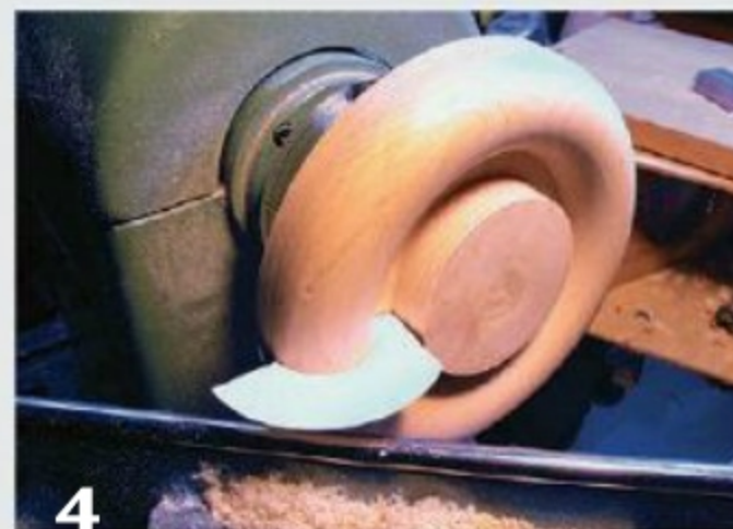
It is important to work from a trued and squared blank, as critical measurements for the torus will be taken from those surfaces. After truing the blank, I formed the outside profile of the half-torus and verified its accuracy with the template. The tenon at center will be used to reverse-mount the workpiece.
