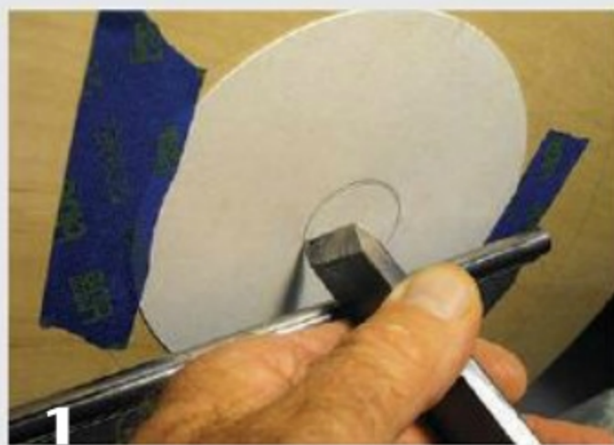
Cardboard templates can be made perfectly concentric on the lathe.
