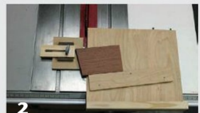
2 The saw is set up for cutting staves. An adjustable stop block, at left, ensures each stave is cut at identical width. The saw blade is tilted to the required bevel angle, in this case, 13°.
