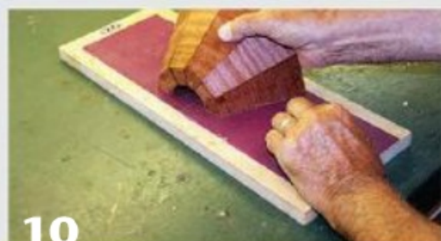
Sand to flatten the mating edges of each half yet to be glued.
