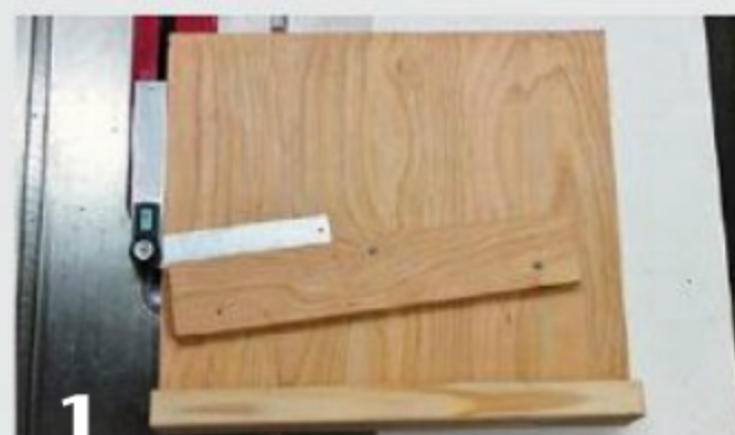
1 The author's shopmade table saw sled for cutting tapered staves, set for a miter angle of 7.6°. Since the digital protractor is aligned with the left edge of the sled, its angle is set to the complement of the miter angle: 90^\circ - 7.6^\circ = 82.4^\circ .
