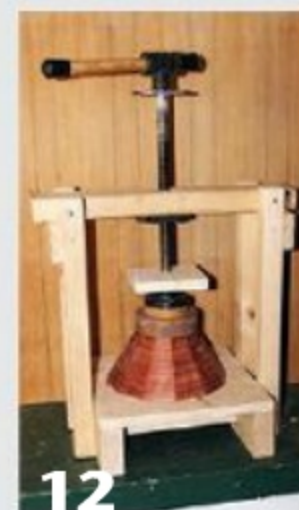
Sand the bottom smooth and flat prior to gluing on the base. I use a shopmade fixture to apply pressure, but an F clamp with a deep enough throat would also work.
