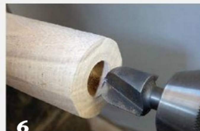
The box body is also hollowed with a Forstner bit, then refined with a box core router bit.
