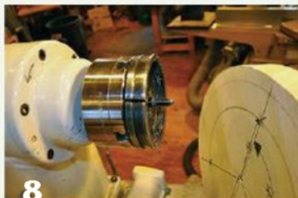
8 A screw held in large chuck jaws provides ample support for turning the seat.
