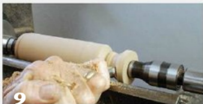
On the true center, create the rough shape of the pepper.
