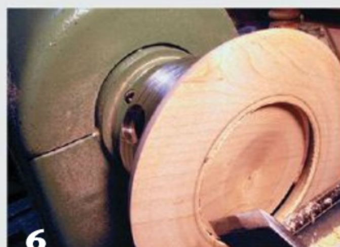
The piece is reverse-mounted so the rounded half-torus is facing the headstock, and what will be the inside gluing surface can be reduced to the desired radius ( \frac{5}{8} " in this case). This face must be dead flat, verified with a straightedge, to ensure a good glue joint. I then parted the half-torus ring from the center material.
