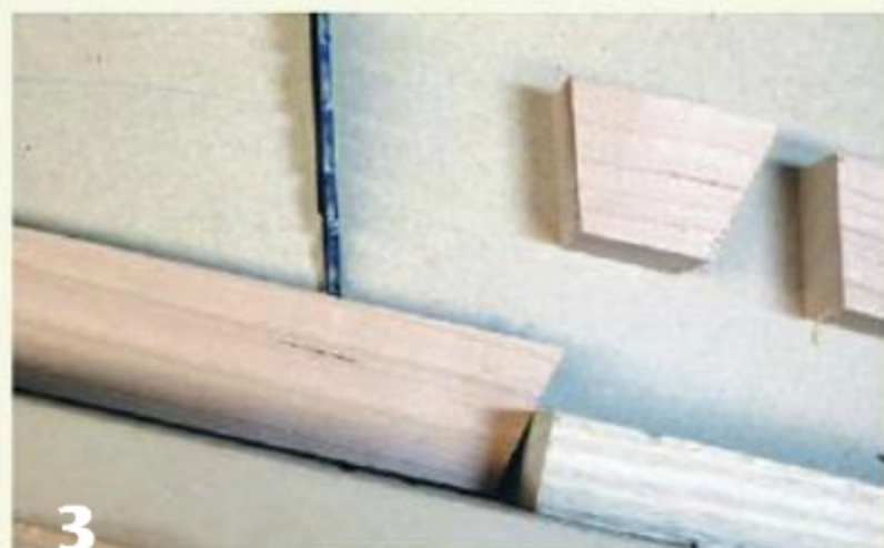
3 The table saw cutting jig makes perfect 30° segments from strips of cherry wood.
