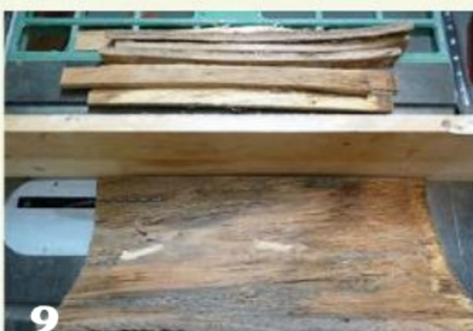
9 Joint one edge of the bark, saw it into strips, and sand the inside surface lightly to flatten each strip.
