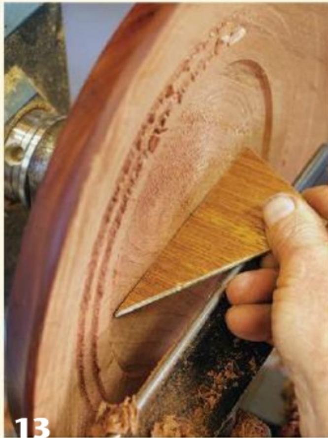
14 Use a shopmade or steel straightedge to identify high spots.
