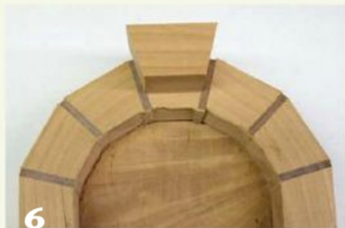
6 Eyeball the overlap between the first and second rings and measure the width of the segments needed.
