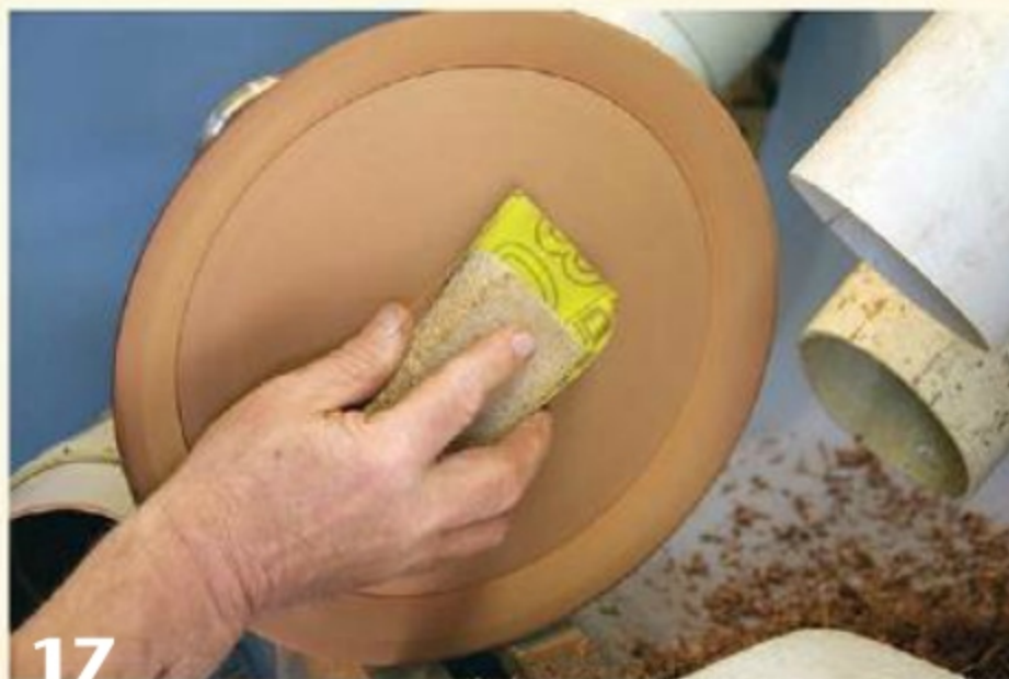
A sanding block helps to eliminate ridges and maintain a flat surface.
