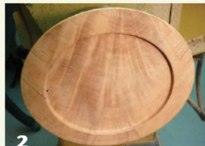
2 Chuck the blank by the tenon and turn what will be the inside bottom surface. Flatten the rim using a sanding board to prepare it for gluing the first segmented ring.
