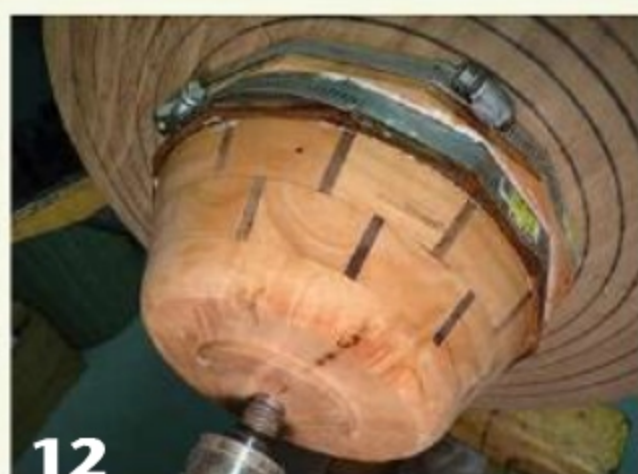
(10) Clamp the bark accent strips to the cherry support strip. Keep everything in line by clamping one strip at a time.
