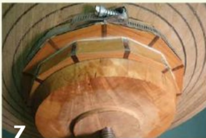
7 Rotate the second segmented ring to position the walnut splines, then glue and clamp it as before.
