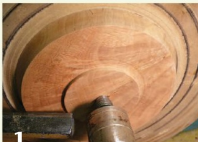
1 Begin by turning the base of the bowl, with a stub tenon for chucking.
