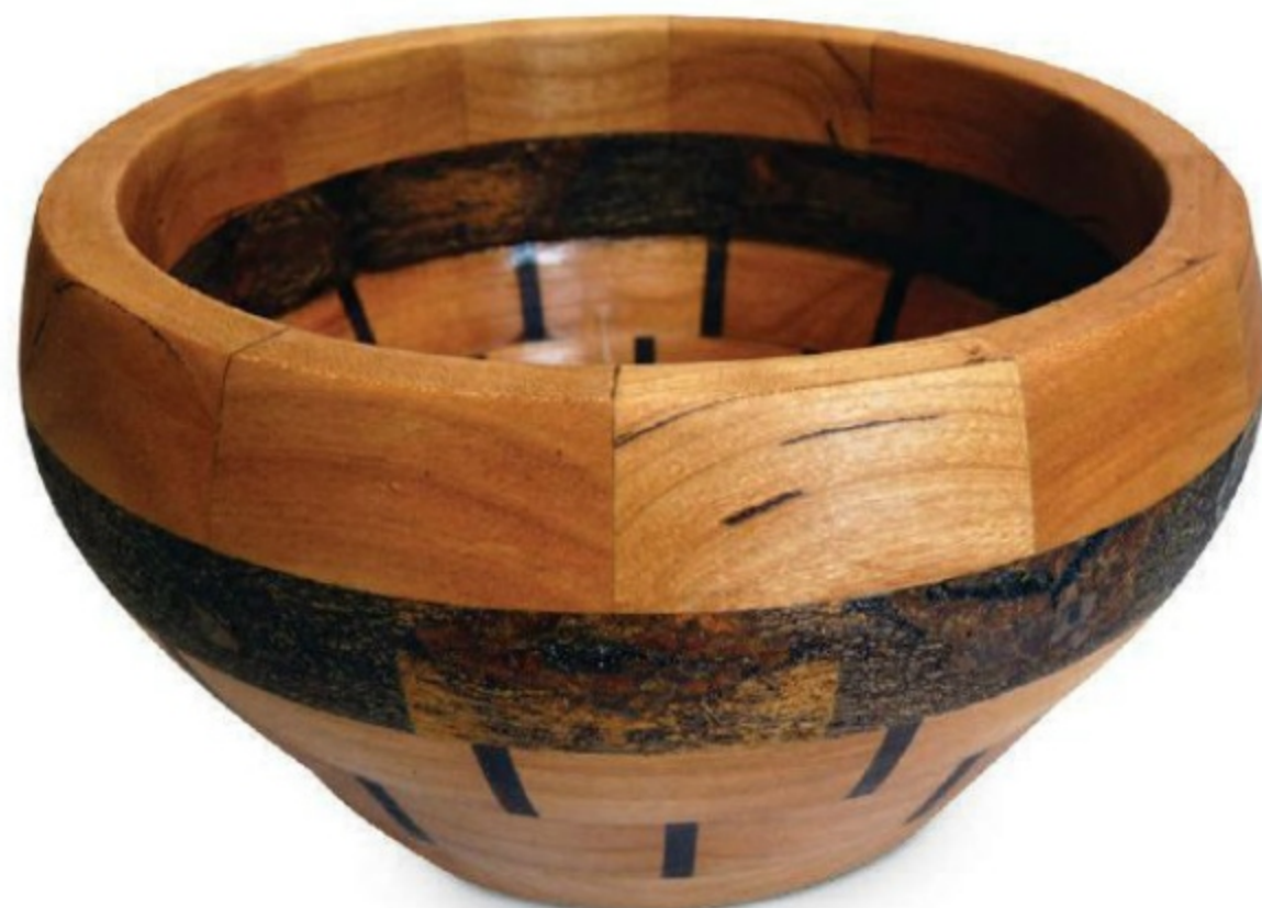
Segmented cherry bowl with walnut splines between the segments and a bold accent ring of oak bark glued onto a solid-wood support strip.
