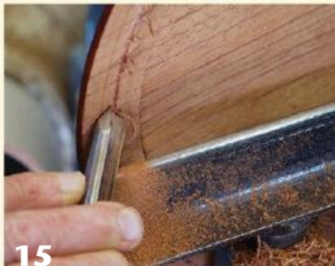
15 Shape the rim using a spindle gouge, cutting from outside in, then define its edge, cutting with the nose of the gouge from inside out.
