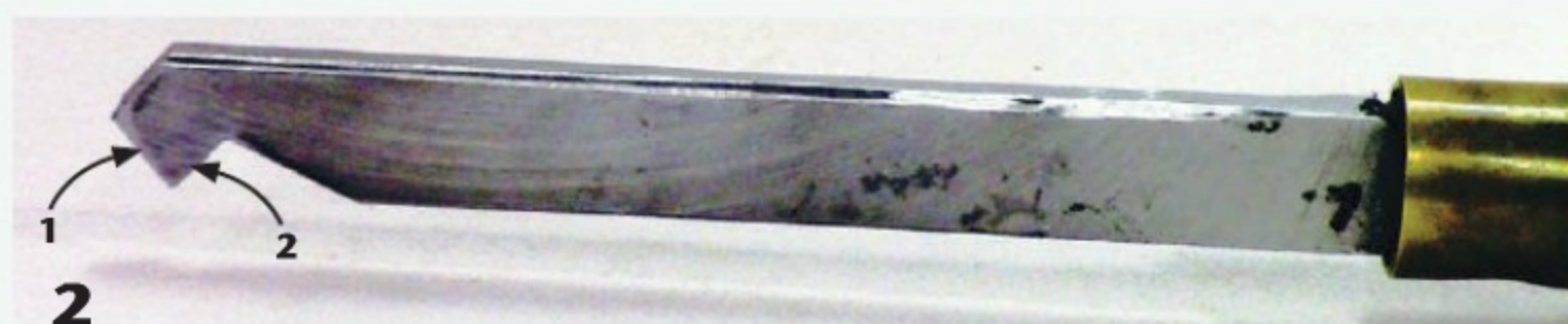
The author's shopmade dovetail recess tool, made from an old skew ½" (13mm) wide and a bit less than ¼" (6mm) thick. Edge 1 forms the bottom of the recess, and edge 2 forms the angled wall. The angle between these two edges should match the angle on the outside of your dovetail jaws (in my case, about 80°). Since edges 1 and 2 are being used as scrapers, their bevels should be ground at a 70° to 80° angle.
