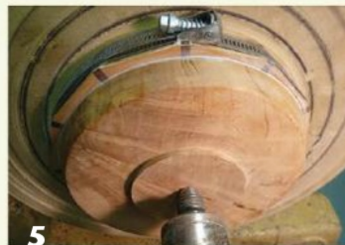
5 The lathe's tailstock applies clamping pressure for gluing the bowl base to the first segmented ring.
