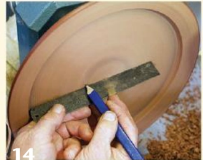
14 Use a shopmade or steel straightedge to identify high spots.
