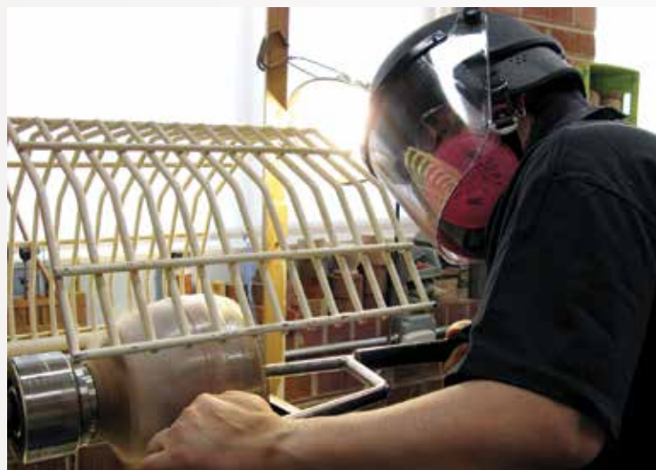
Turning with the wire guard in place, wearing my riot helmet and respirator. The piece, which has multiple cracks, is wrapped in plastic stretch wrap for reinforcement.
