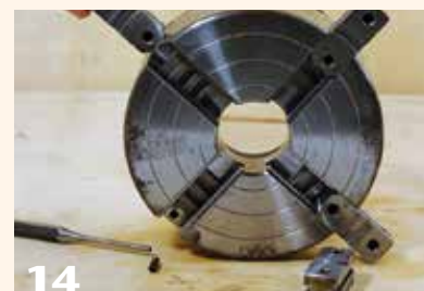
14 Reinstall the jaw slides in sequential order.
