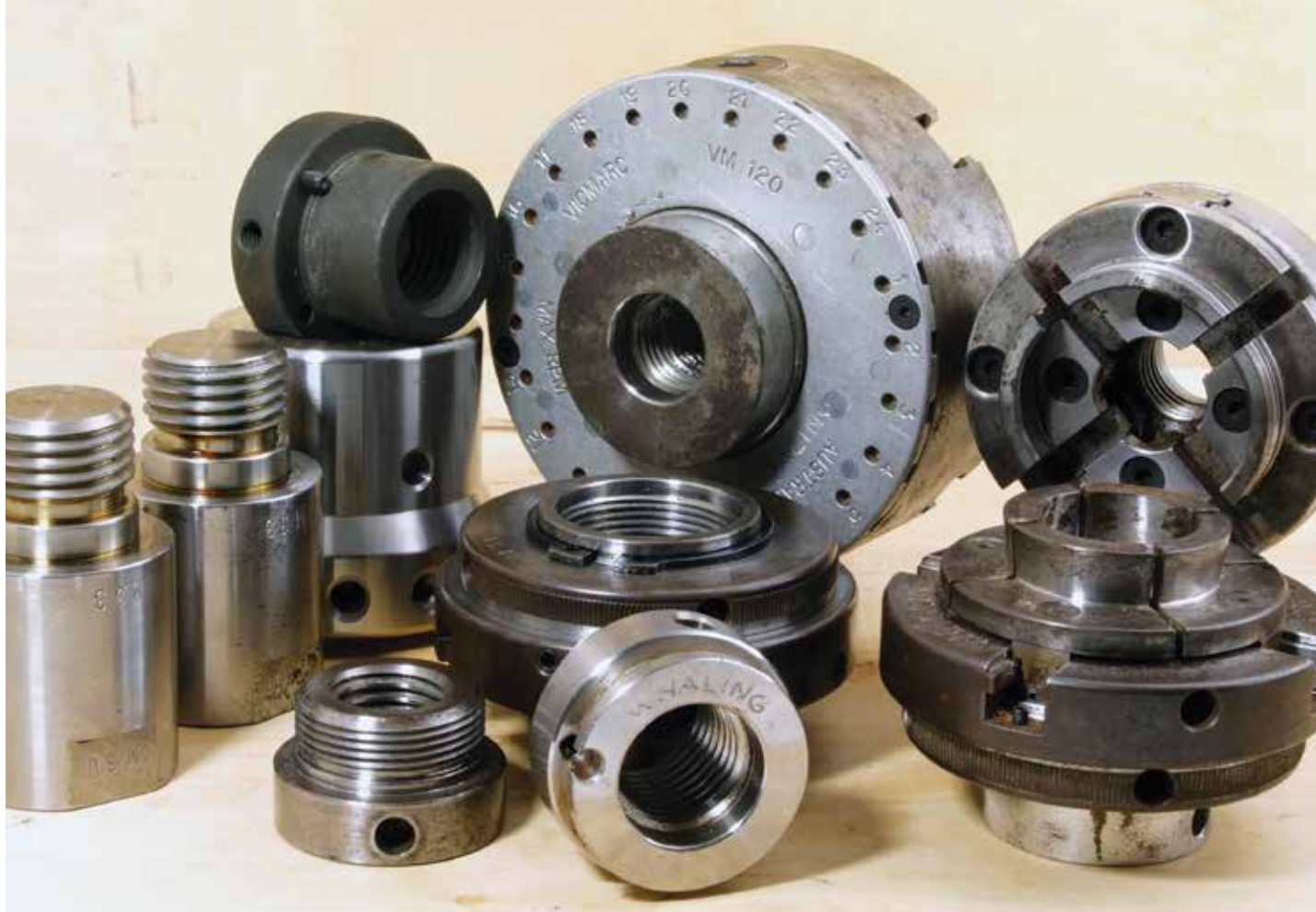
A selection of four-jaw scroll chucks and spindle inserts.
