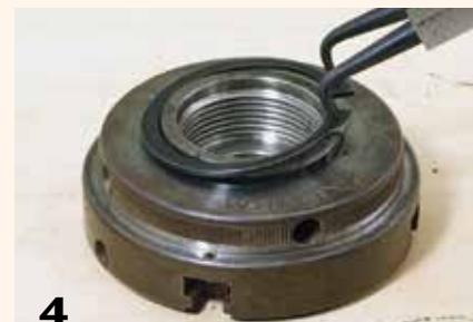
4 Removing the retaining clip from the back of the chuck.
