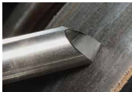
The leather honing wheel removes the grooves from the wet wheel.
