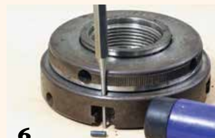
6 Removing the stop pins that prevent the jaws from backing out of the chuck body.
