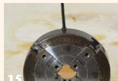
15 Setting the washer and grub screw to establish resistance in the scroll mechanism.
