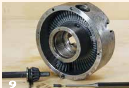
Exposed inner workings of geared chuck. Note the small grub screws that secure the pinion dowels.
