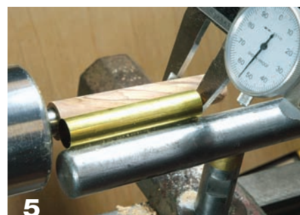
Measure the thickness at the end of the internal brass tube to avoid breaking through on the blank.
