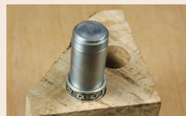
A conical steel round will allow you to slightly expand a sterling-silver ring.
