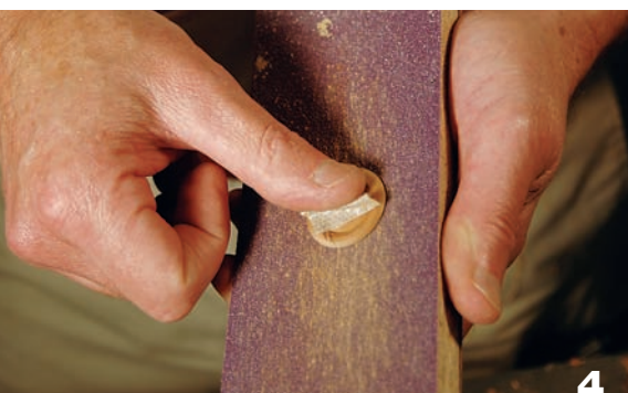
Sand the back of the button on a 180-grit belt. A piece of double-faced tape will help you keep the button in contact with your thumb.
