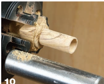
10 Drill and turn a wood tube for the finial.
