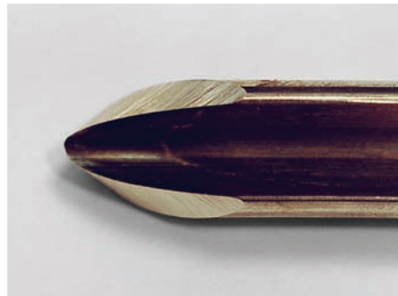
The wing (side) profile of Lyle Jamieson's favorite grind has a nearly straight line from the tip to the wing corner.
