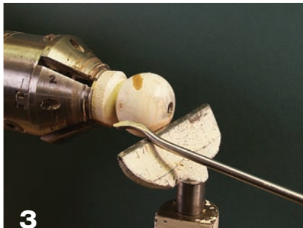
3 With micro hollowing tools, reduce the globe wall thickness to ⅛".
