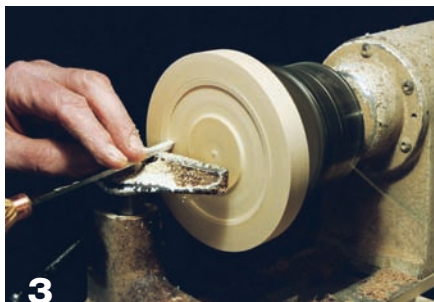
3 Slide the friction-fit tool along the tool rest until you reach the marked diameter.
