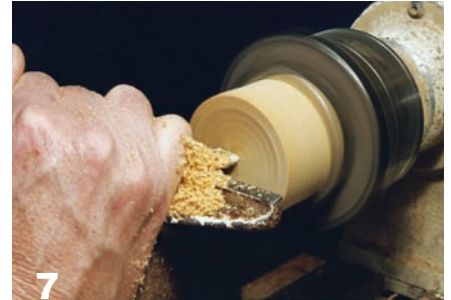
7 Before fitting the lid, use a spindle gouge to remove the waste material.
