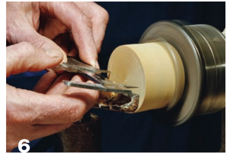
6 On a soft pine wasteblock, use calipers to mark the diameter of the lid interior.
