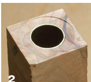
Square the blank before turning.
