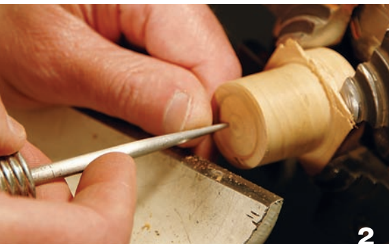
Use a scratch awl to lay out button holes, then use a \frac{1}{32} " or \frac{1}{16} " bit to drill the holes.
