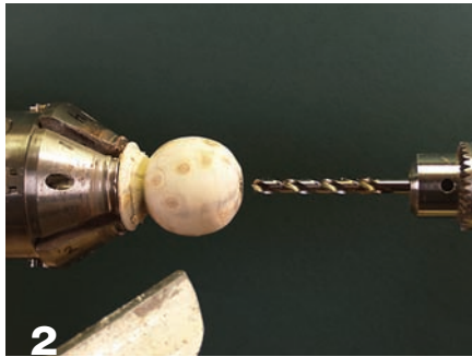
2 Mount a ¾" brad-point bit in a Jacobs chuck, then drill through the globe.
