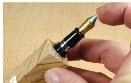
Dry-fit the pen parts to test the drill depth.
