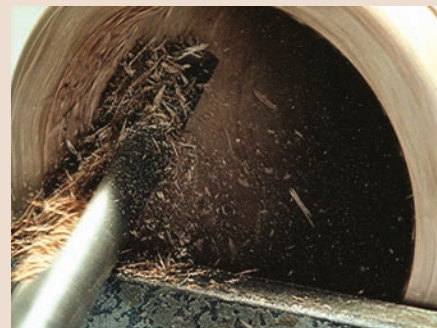
Even with hard and dry wood, this pull cut on a hollow vessel works well to remove shavings.
