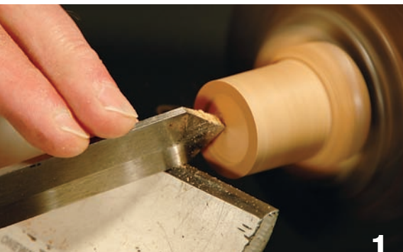
With a parting tool, turn the button profile. The cherry stock above is \frac{5}{8} "-diameter face grain.
