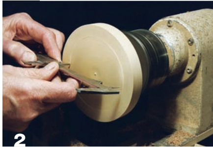
2 With calipers, transfer the bowl's rim diameter to the wasteblock.
