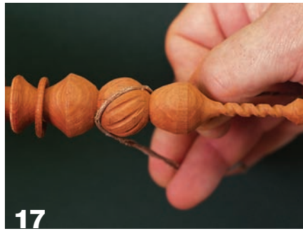
17 Use ropes of twisted sandpaper to smooth the twists in the icicles.
