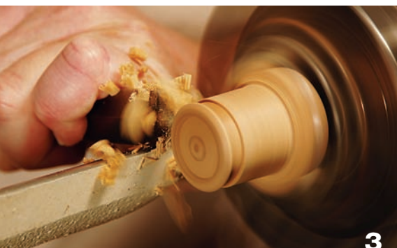
Use a parting tool to separate the button from the turning block. There should be plenty of stock remaining in the chuck to turn matching buttons.
