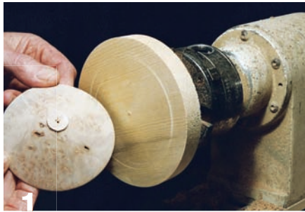
1 To turn the bottom of a bowl, first prepare a flat surface on a wasteblock.
