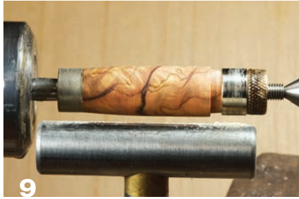
9 With a skew, turn a gentle curve.
