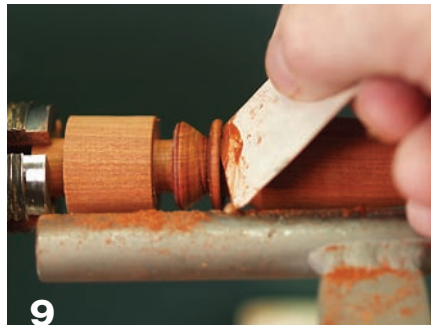
9 Before parting off the captive ring, smooth the surfaces with wax-loaded sandpaper.
