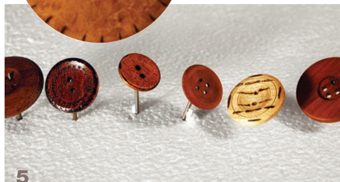
Rest the buttons on the tips of small finish nails or tacks while the finish dries.
