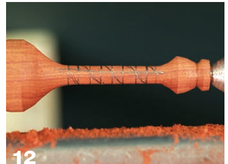
12 Lay out the two cut lines for the right-handed double-barley twist.
