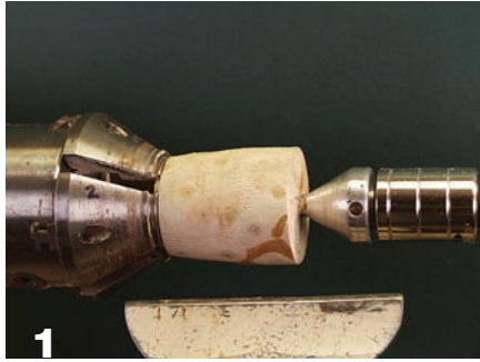
1 With a spindle roughing gouge, turn the globe stock to about a 2½" diameter.
