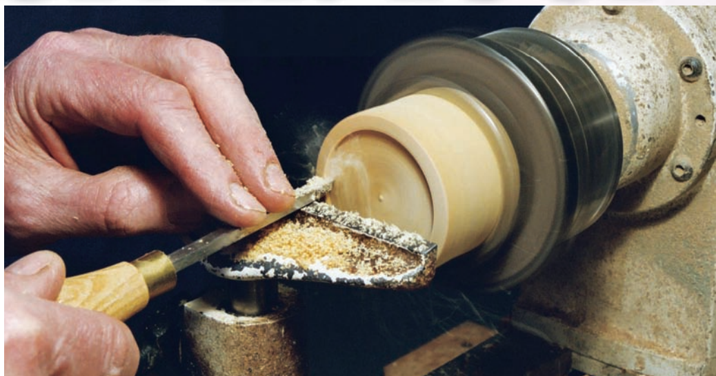
A friction-fit tool is ideal to create a tight-fitting wasteblock before turning the bottom of a bowl.
