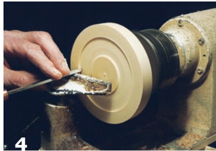
4 Tilt the friction-fit tool to the left to finesse the final diameter.
