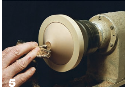
5 Mount the bowl in the wasteblock, then turn the bowl bottom with a spindle gouge.
