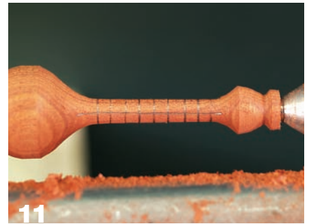
11 At the tailstock end, lay out start and pitch lines for the double-barley twist.
