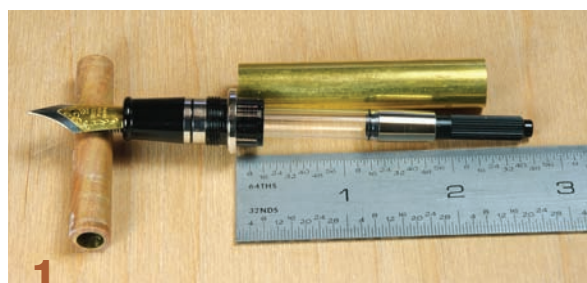
To determine the drill depth, assemble the pump on the front section.
