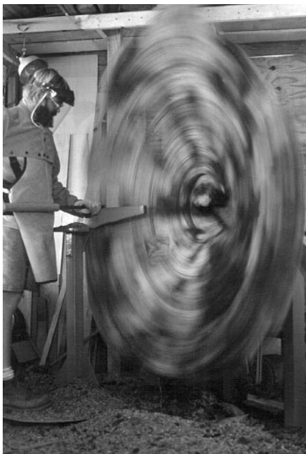
Hultgren's lathe, upper left, is constructed of 3" angle iron and 5/8" steel plate, and the 2" spindle is powered by a 5-hp motor geared down with a truck transmission. At 150 rpm, left, the speed at the perimeter of the root blank sent chips up to 30' away. The finished piece, above, includes holly inlay and is 5'9" across and 18" deep.
