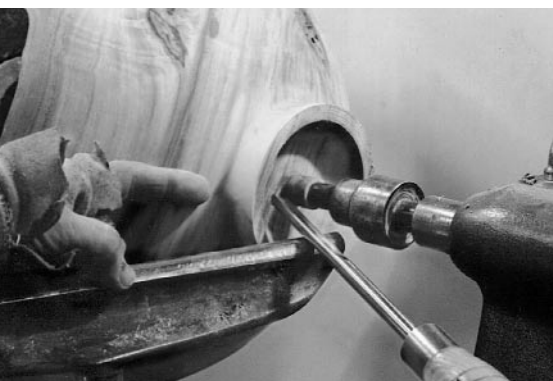
A small (3-inch) faceplate, top, allows flexibility in designing the legs. With the bowl reverse-mounted, above, use a \frac{3}{8} " gouge to hollow the base.
