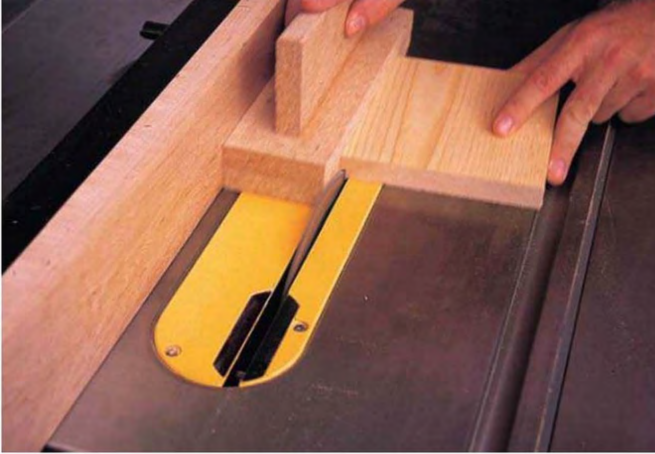
Shown here is the wedge jig.
