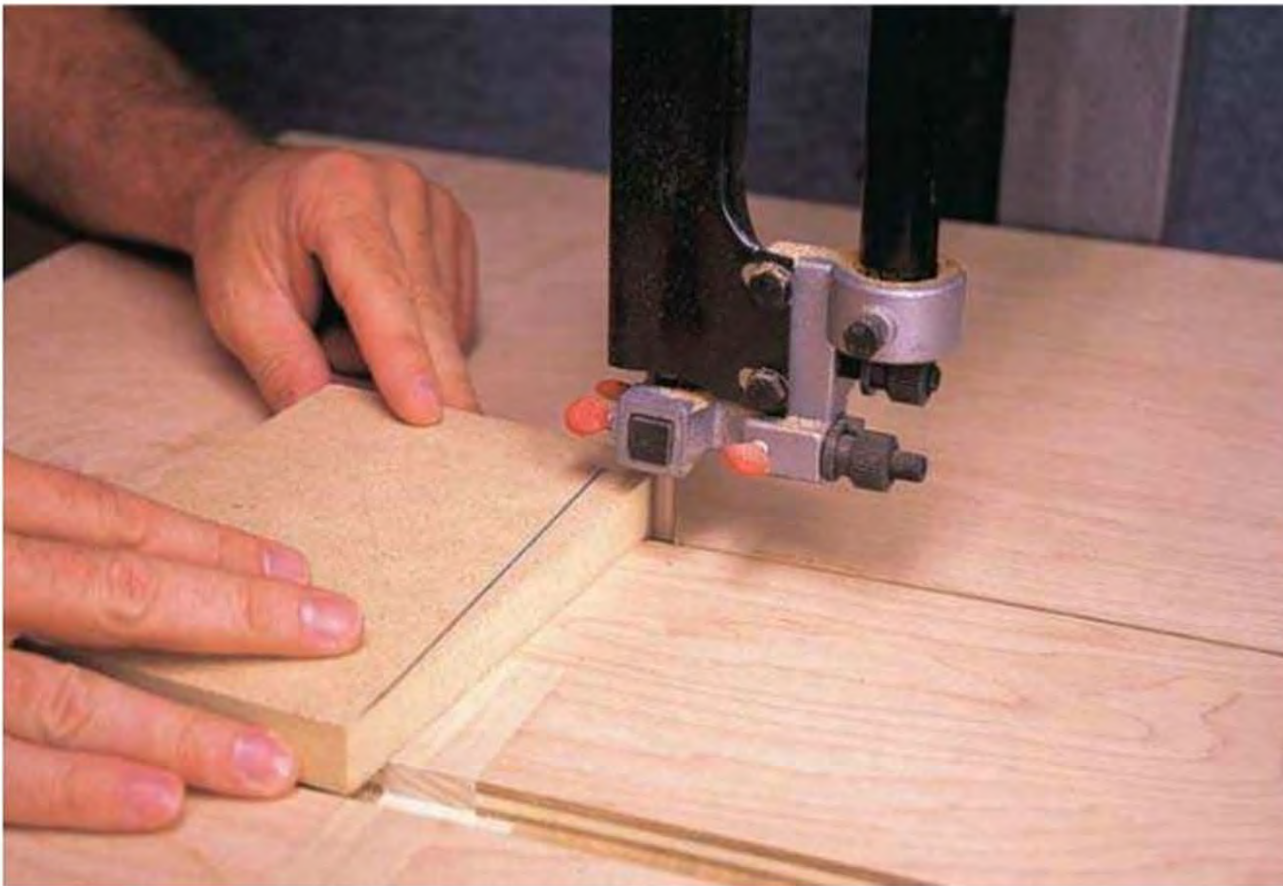
After drawing the shape of the taper for either the taper jig or the wedge jig, make the short cut first.
