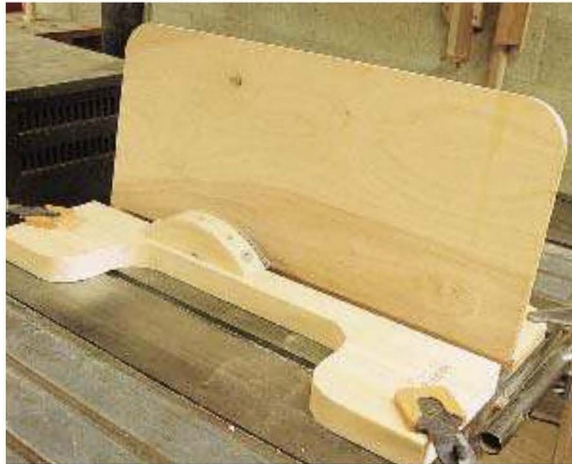
STEP 13 Fasten the jig and the blade guard to the saw with clamps as shown.
