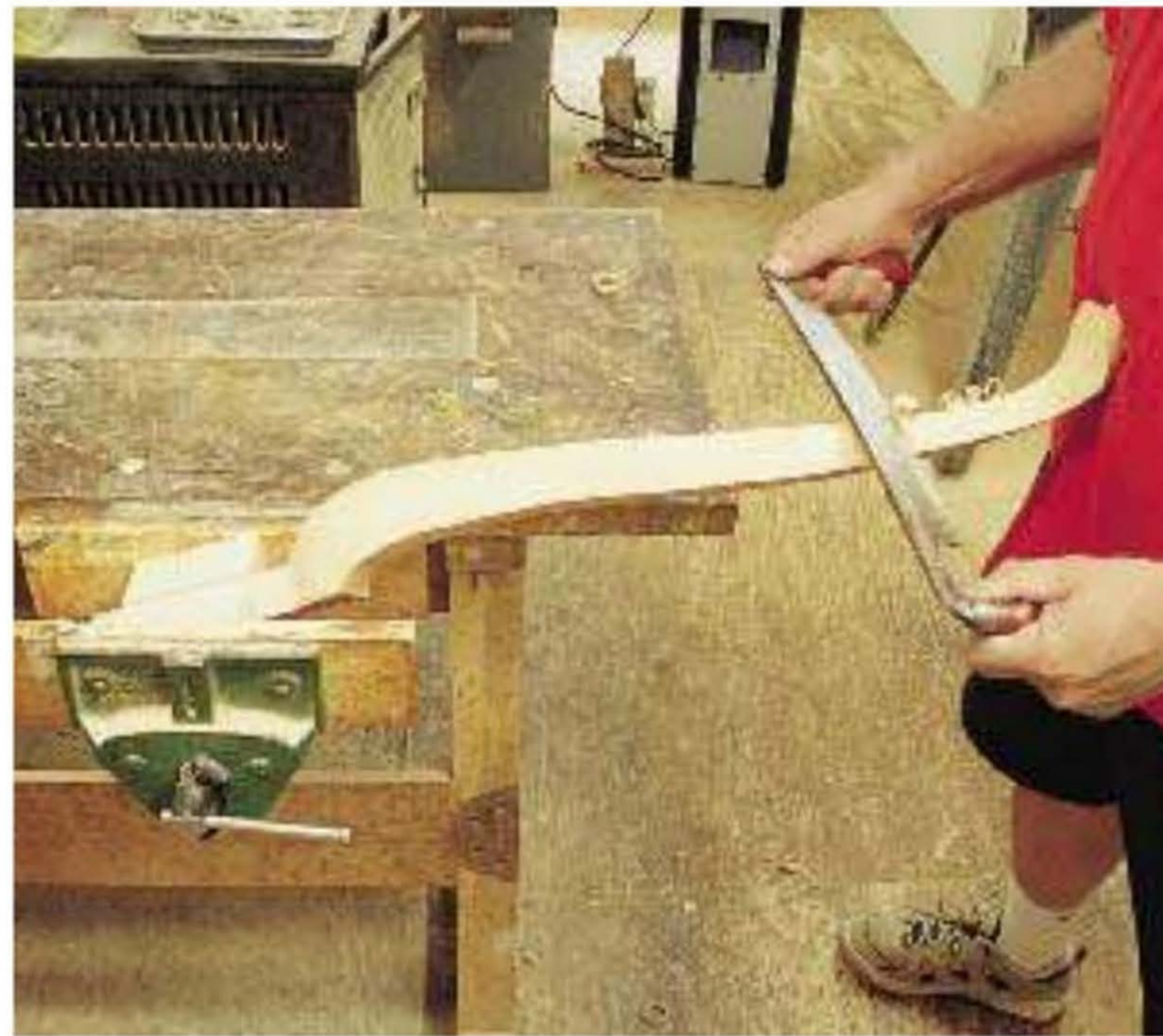
STEP 7 A pair of V-blocks can be used to hold a cabriole leg in your vise in a position that allows you to fair together two faces of the cabriole leg.
