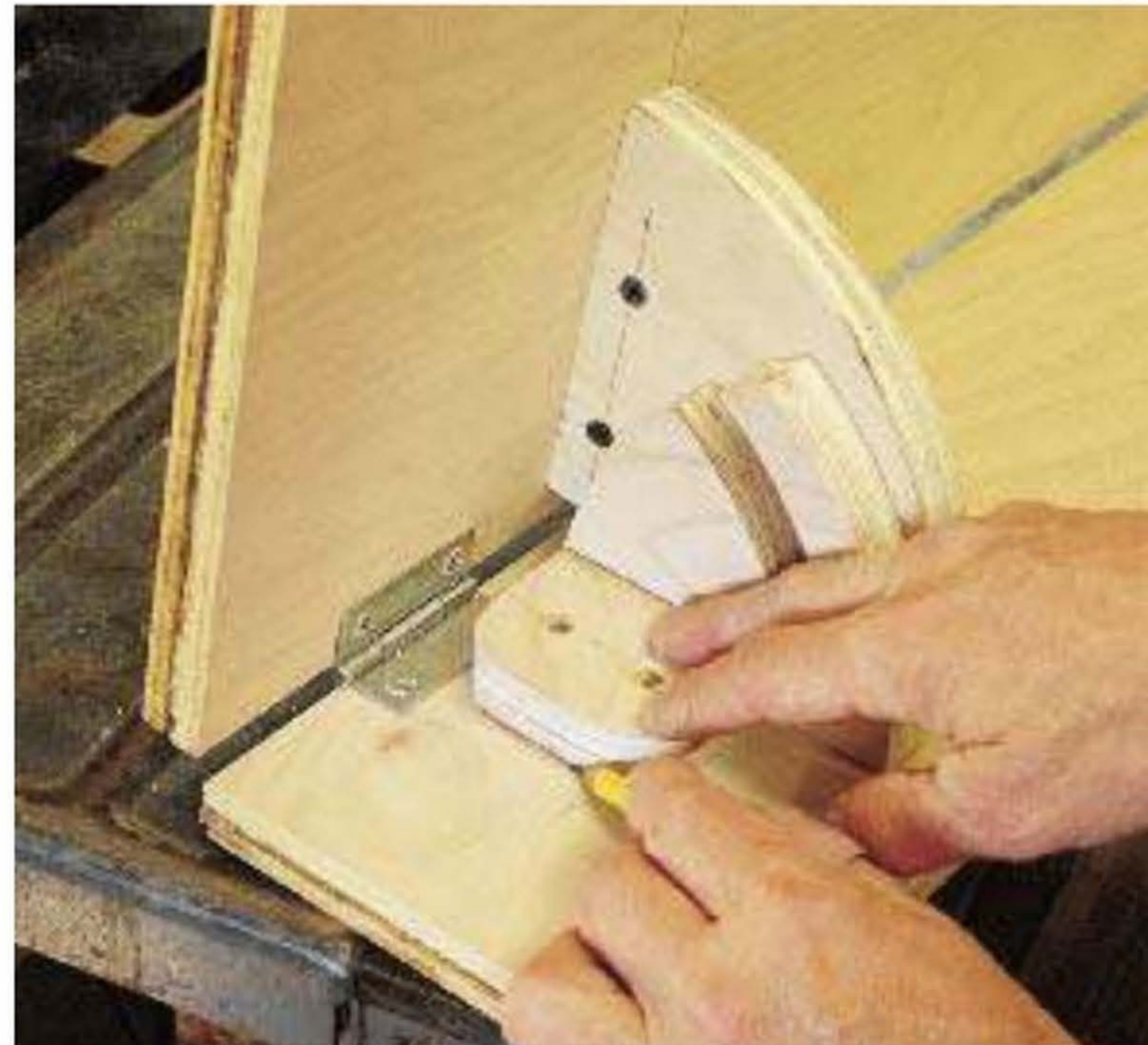
STEP 7 Using the bracket on the vertical leaf as a guide, determine where to place the cleat that will mount the bracket on the horizontal leaf.
