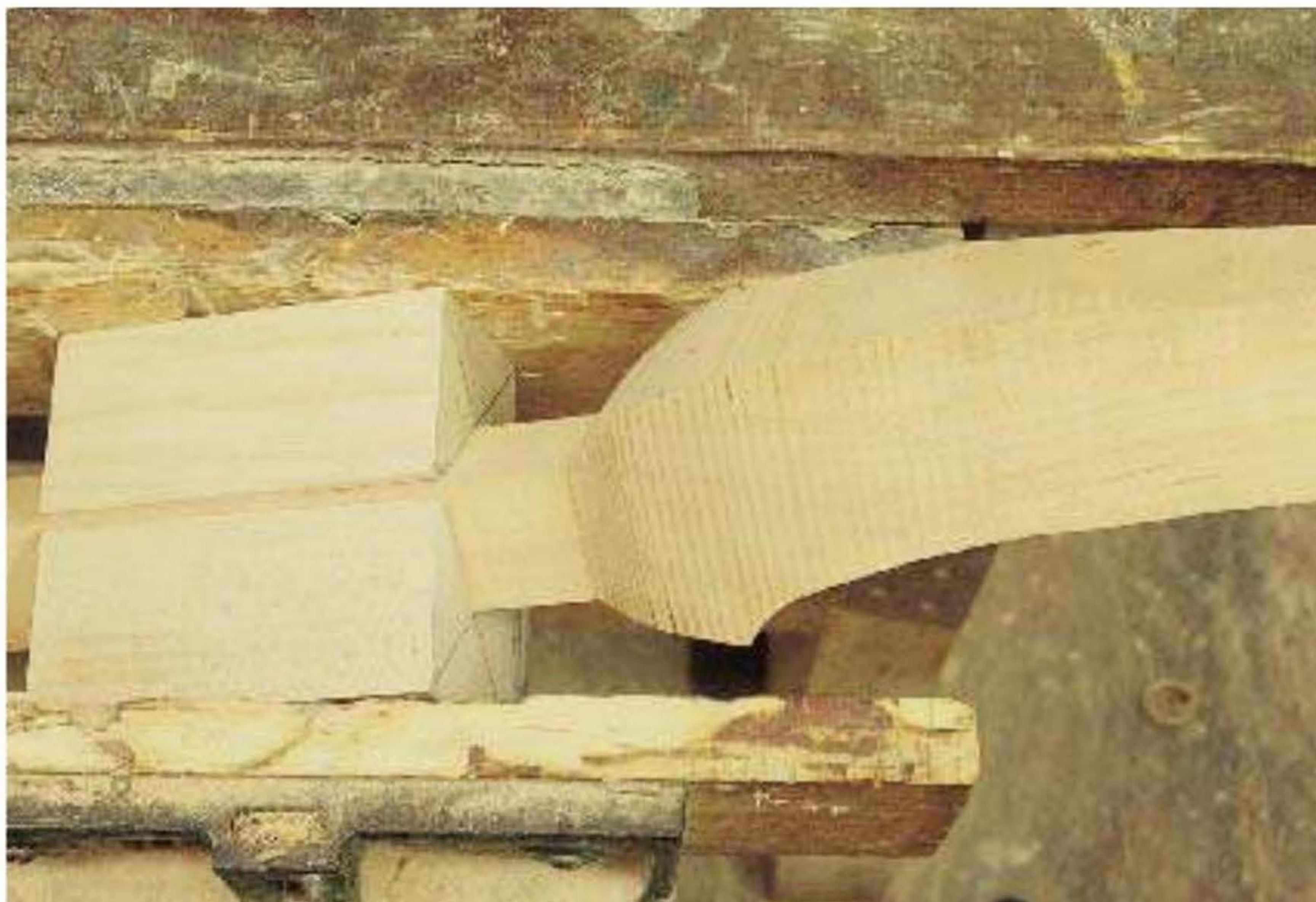
STEP 8 This detail shows how the V-blocks fit into the vise. Notice that in order to hold this rather thin leg post, I had to select V-blocks small enough so that the depth of the V cut in each is less than the thickness of the post being worked.
