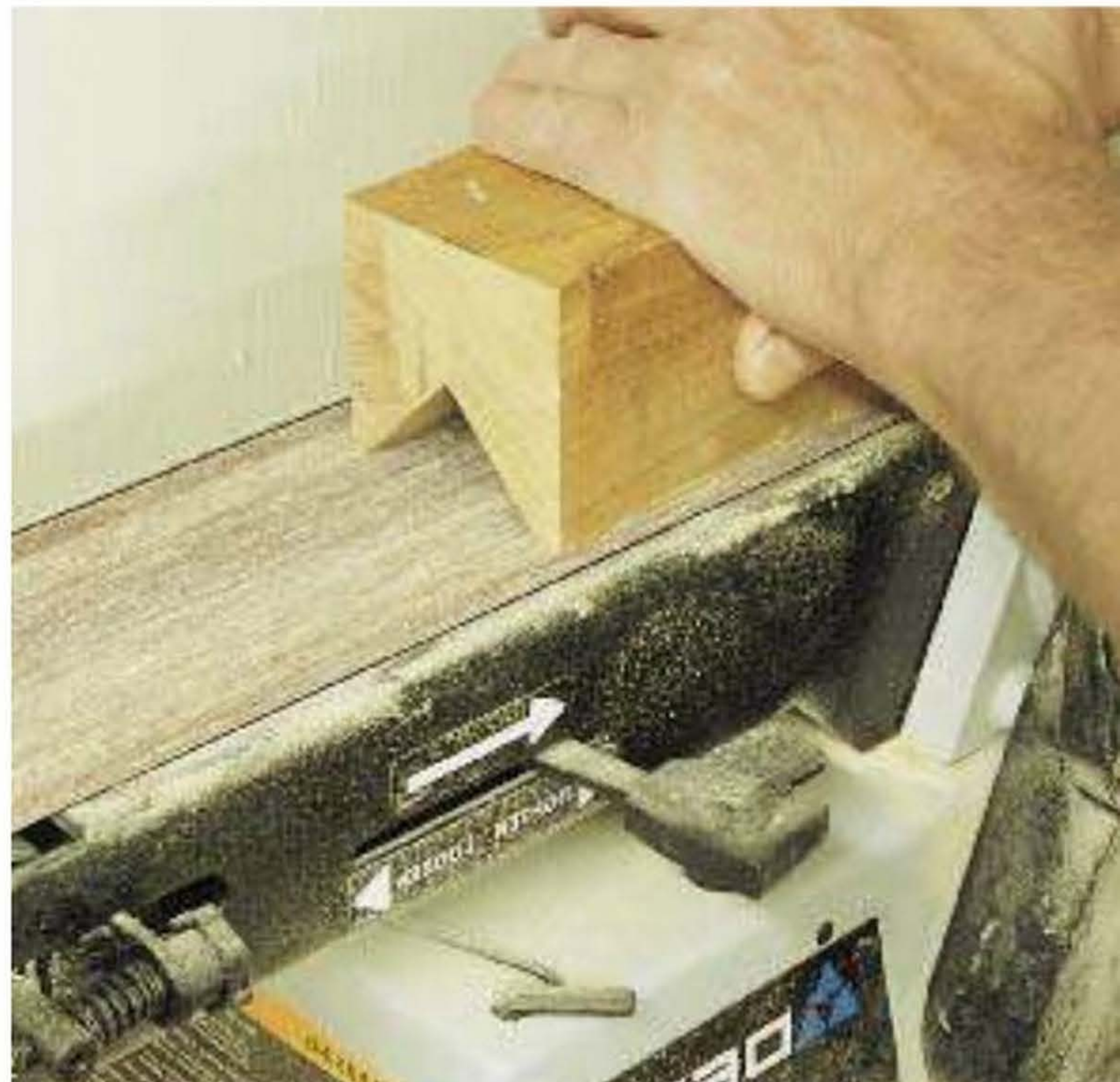
STEP 3 I laid the cut corners on my belt sander to flatten the sharp, and therefore fragile, corners.
