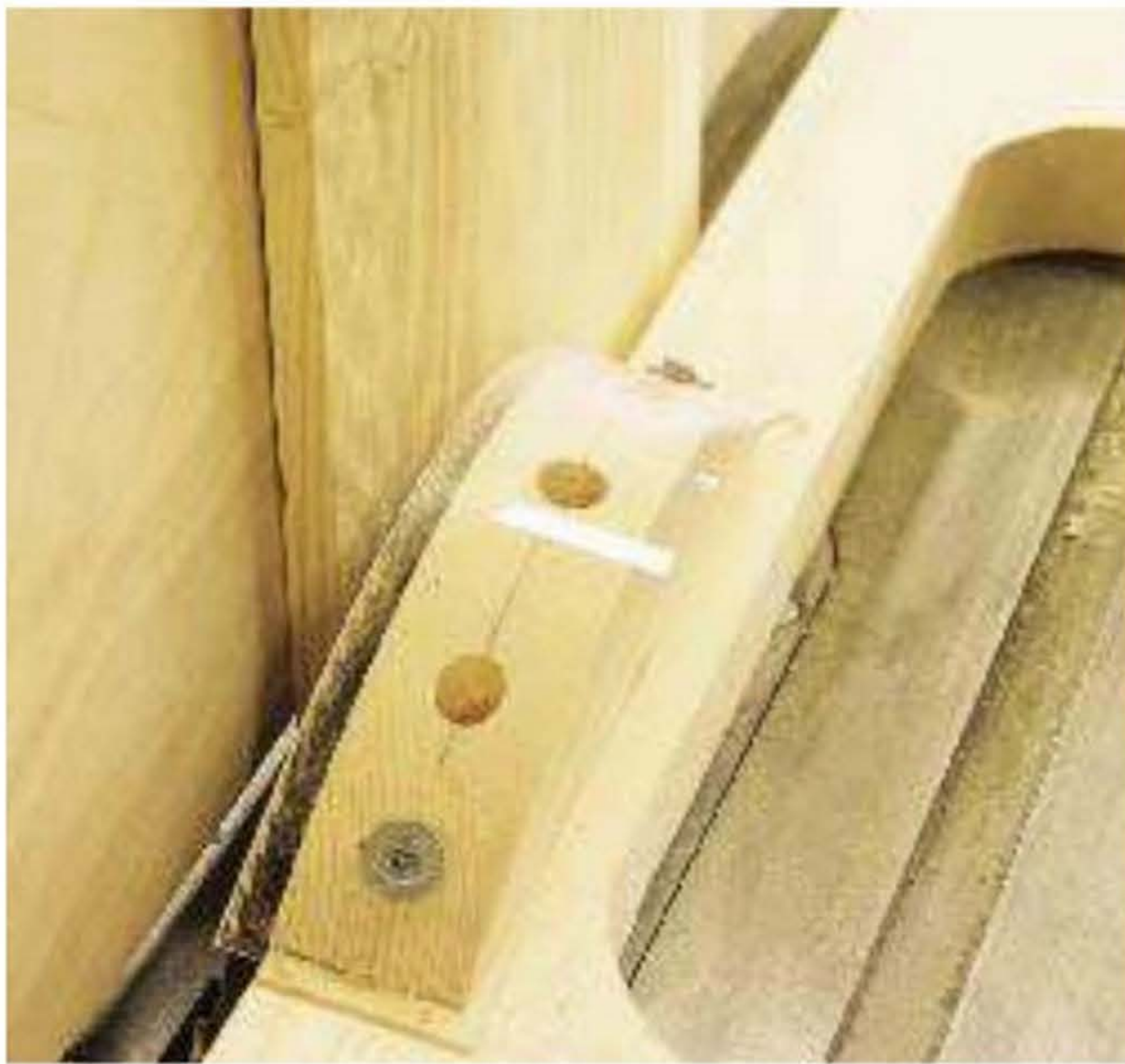
STEP 14 It would be very difficult for your fingers to make contact with the saw blade.
