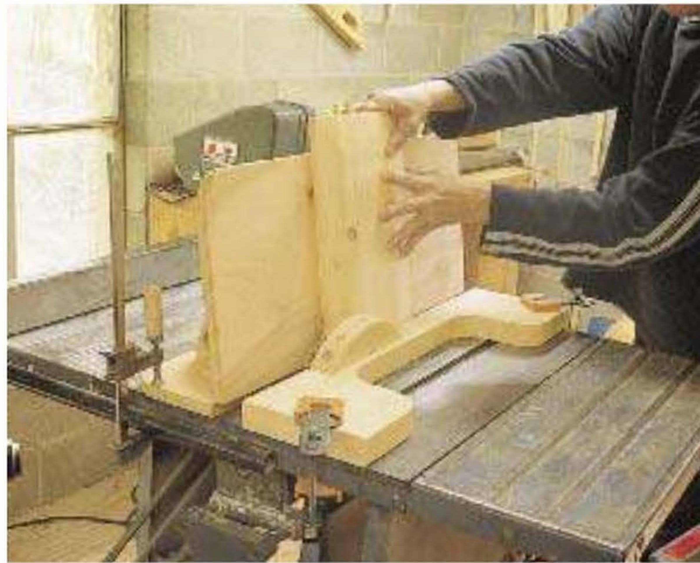
STEP 15 Set up the jig by placing it in the approximate location on the saw table. Then measure from two points along the miter-gauge slot to the jig. It's important to measure from two points because the jig must be parallel to the miter gauge slot and therefore the blade. If it isn't, the heel of the blade may dig into the work leaving behind unsightly saw marks that will be difficult to clean up with hand tools.
