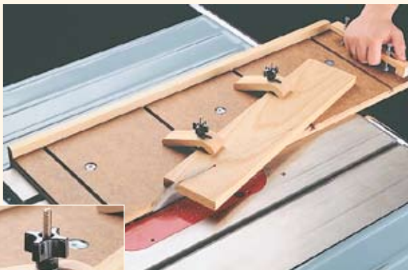
▲ Angled Cuts. Two adjustable hold-downs clamp work securely in place when making angled cuts.
