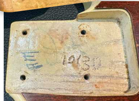
When it was modified/fixed at the Fender factory, workers applied nail-marked numbers to the neck end and neck cavity to ensure they'd be properly reunited.
