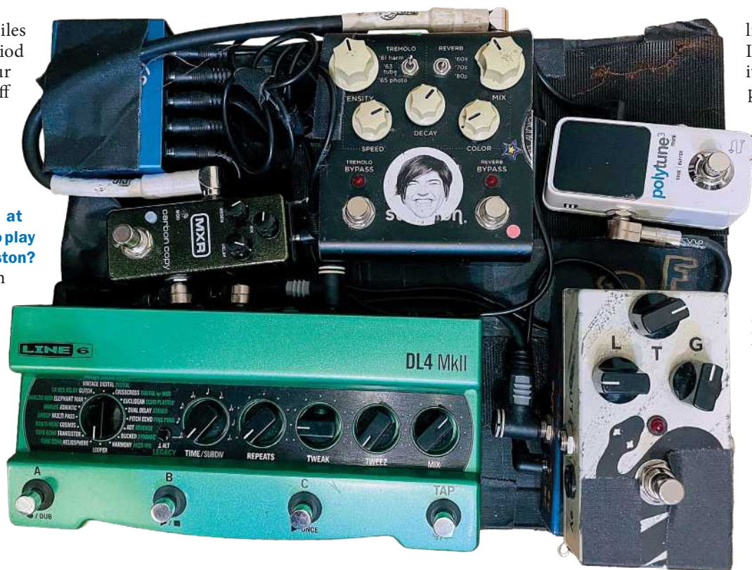
Frisell lists his effects pedals as TC Electronic Polytune 3 tuner, Line 6 DL4 Mk II, JAM Pedals Rattler distortion, MXR Carbon Copy Mini analog delay, Strymon Flint Reverb-Tremolo, and a Strymon Ojai power supply.
