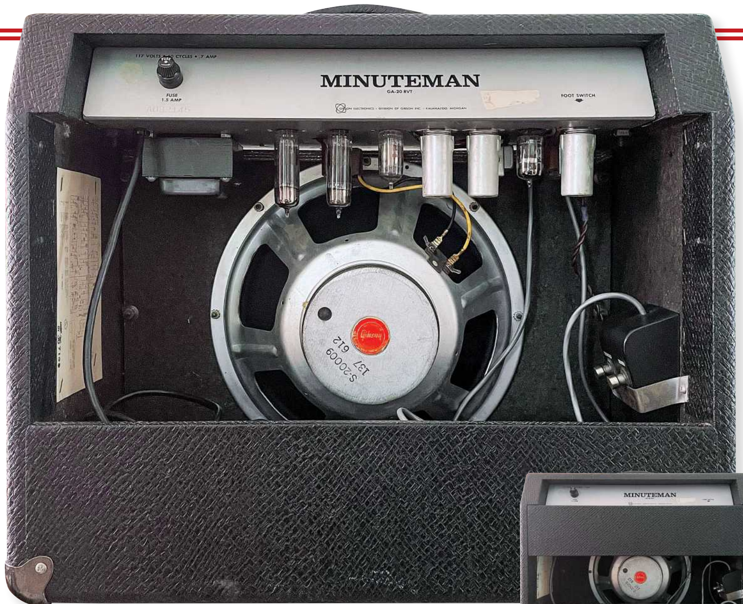
The 6EU7 (inside metal shields) and 12AU7 preamp tubes lead to the dual EL84 output tubes (left); note the footswitch in its holder.
