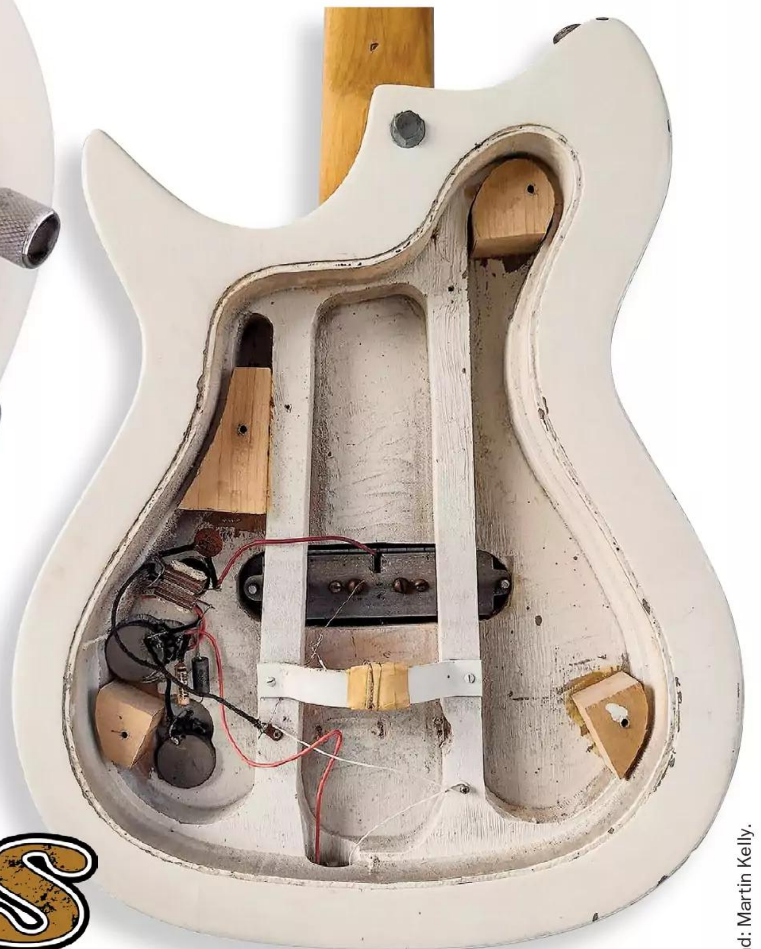
The Combo 600's back reveals extensive routing and basic wiring for the horseshoe pickup.
