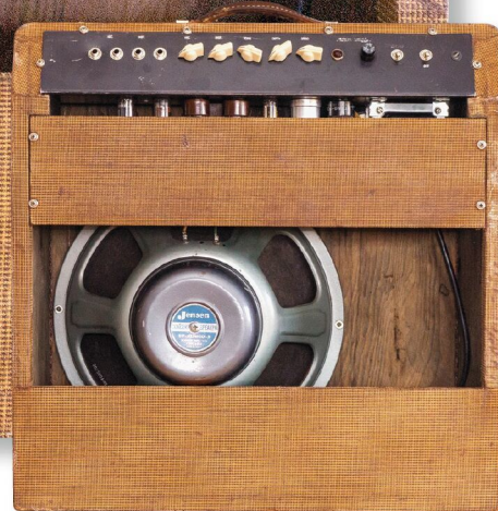
A look at the back reveals the 15" Jensen P15P speaker and DIY aesthetic of the chassis, control panel, and tweed covering. The 8" Jensen is tucked high, behind the chassis.
