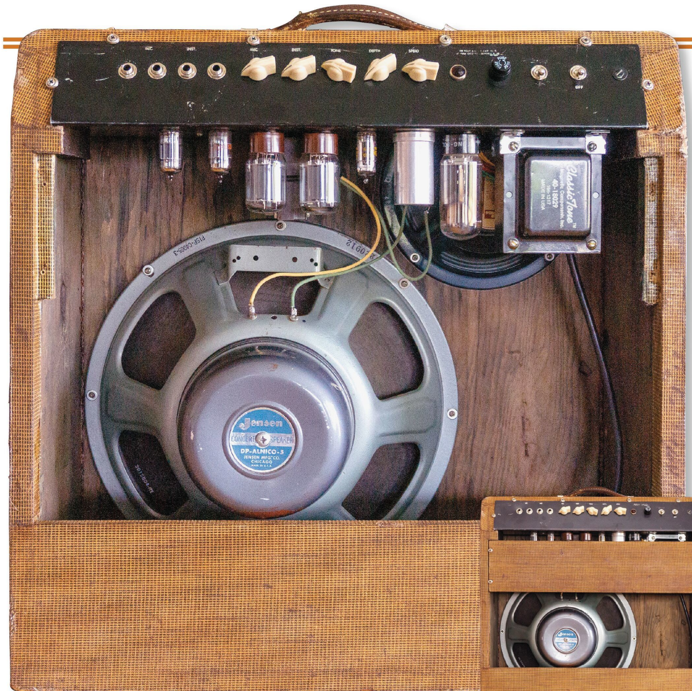
A look at the back reveals the 15" Jensen P15P speaker and DIY aesthetic of the chassis, control panel, and tweed covering. The 8" Jensen is tucked high, behind the chassis.
